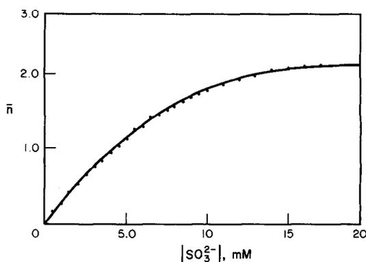
Fig. 2. Definitive formation curve obtained by extrapolation of  $\log \bar{n}$  vs  $C_{\text{HSO}_3^-}$ . These data were integrated in order to give the  $F_0(x)$  function.
