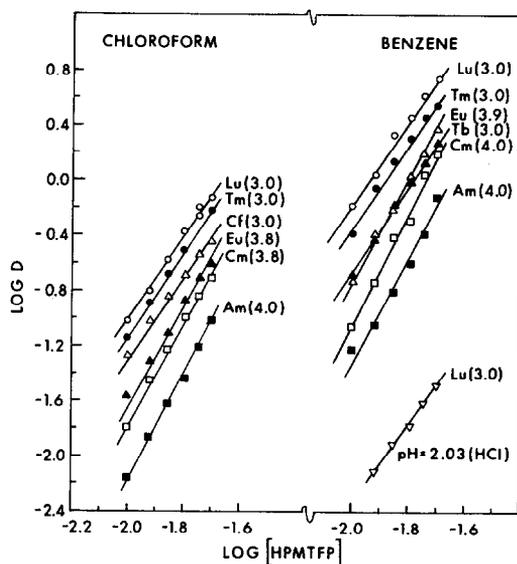
Fig. 1. Variation of  $\log D$  of trivalent actinides and lanthanides as a function of HPMTFP concentration. Aqueous phase: pH 2.70 (0.01 M chloroacetate buffer containing 0.1 M  $\text{NaClO}_4$ ) in all systems except the lower curve for Lu having pH 2.03 (HCl). Org. phase: 0.01–0.02 M, HPMTFP in chloroform or benzene.
