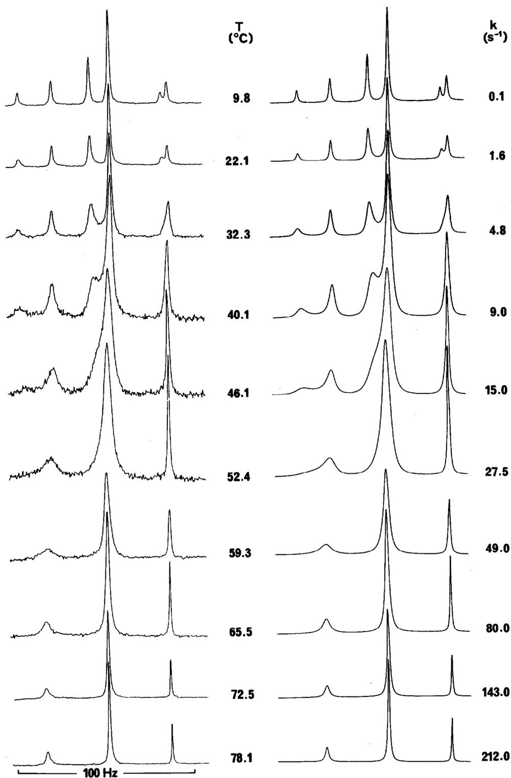
Fig. 11. Experimental and computer synthesised  $^1\text{H}$  NMR spectra of  $[\text{PtMe}_3(\text{MeSCH}_2\text{CH}_2)_2\text{O}]^+\text{BF}_4^-$  showing the effects of scrambling of the Pt—Me signals.
