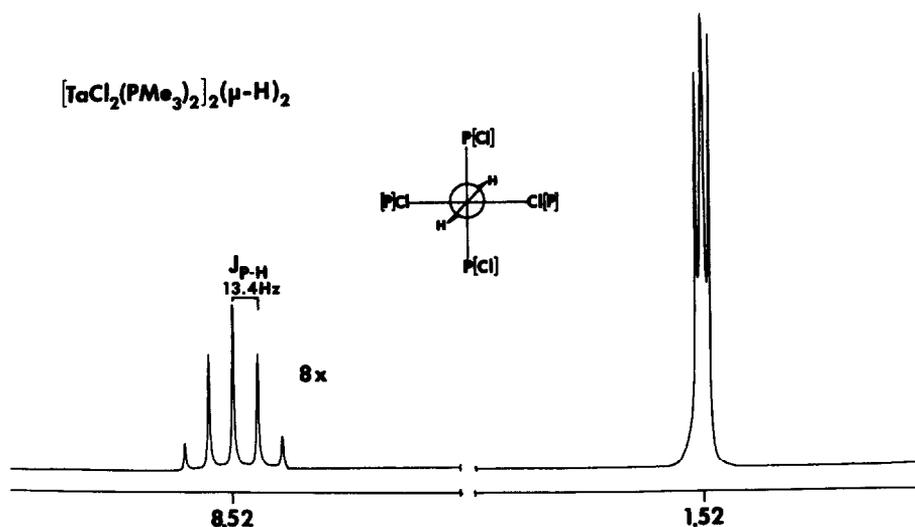
Fig. 1. 360-MHz  $^1\text{H}$  NMR spectrum of  $\text{Ta}_2\text{Cl}_4(\text{PMe}_3)_4\text{H}_2$ . In this and the following proton NMR spectra, end-on Newman projections are included and the atoms in brackets ([ ]) are associated with the back tantalum.
