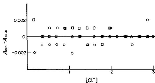
Fig. 5.  $A_{\text{exp}} - A_{\text{calc}}$  plotted as a function of  $[\text{Cl}^-]$  for different chromium(VI) concentrations at  $\lambda = 330 \text{ nm}$ .
