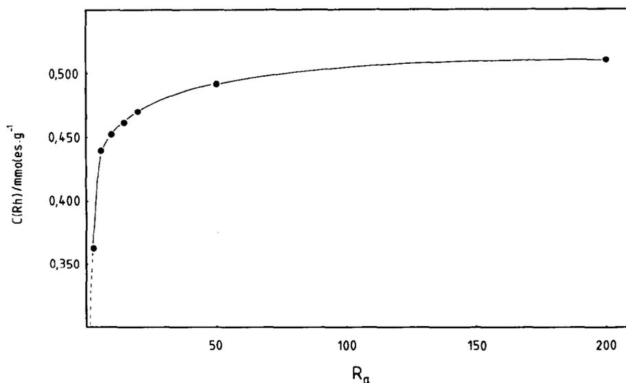
Fig. 3. Sorptive capacity of polyurethane foam toward Rh(III)[C(Rh)] as a function of the Sn(II):Rh(III) mole ratio ( $R_a$ ) from  $2.0 \text{ mol dm}^{-3}$  HCl at 313 K.
