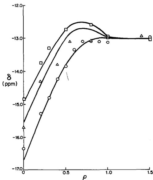
Fig. 1. K-39 chemical shifts as a function of the ratio [DB30C10]/[KSCN] for different total KSCN concentrations. ○: [KSCN] = 0.025 M; △: [KSCN] = 0.050 M; □: [KSCN] = 0.070 M. The data points are experimental and the curves were calculated following the results of the regression analysis displayed in Table 1.
