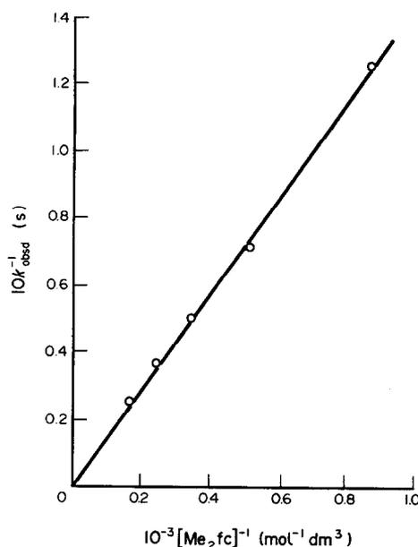
Fig. 3. Plot of  $k_{\text{obsd}}^{-1}$  against  $[\text{Me}_2\text{fc}]^{-1}$  for the reaction of complex 1 with  $\text{Me}_2\text{fc}$  in acetonitrile at 25°C.
