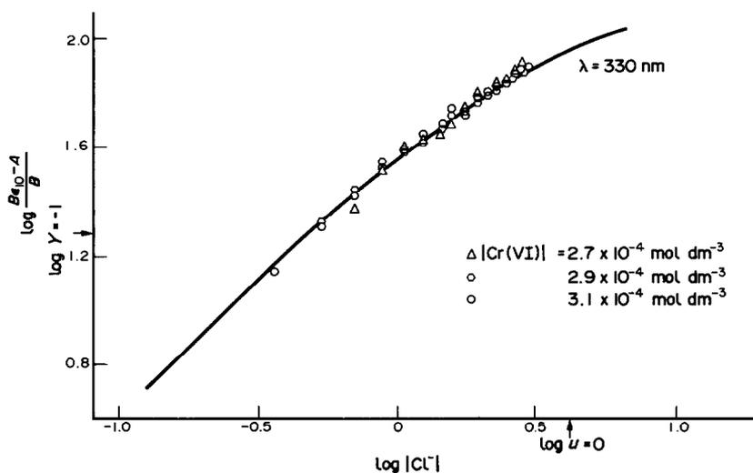
Fig. 2.  $-\log(B\epsilon_{10}-A)/B$  plotted vs  $\log[\text{Cl}^-]$  at  $\lambda = 330$  nm for different chromium(VI) concentration. The full drawn line gives  $\log Y$  as a function of  $\log u$  in the position of the best adjust.
