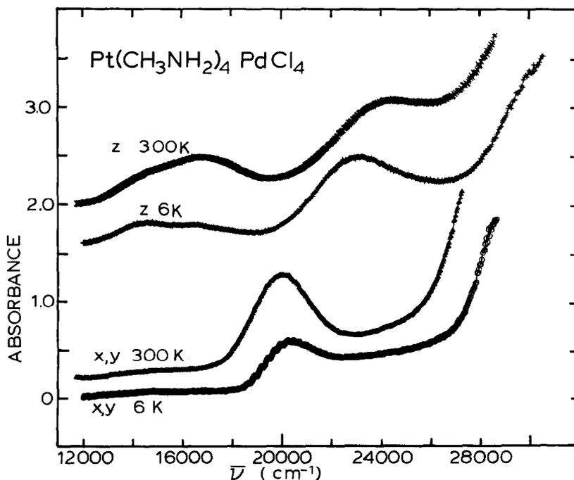
Fig. 16. Polarized spectra for  $\text{Pt}(\text{CH}_3\text{NH}_2)_4\text{PdCl}_4$  crystal,  $11\ \mu\text{m}$  thick.
