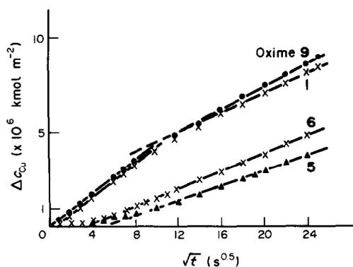
Fig. 2. Relationship between the copper transferred and the square root of the extraction time (xylene, pH = 3.0,  $c_{\text{Cu}^{2+}} = 0.015 \text{ mol dm}^{-3}$ ,  $c_{\text{oxime}} = 0.025, 0.05, 0.025$  and  $0.009 \text{ mol dm}^{-3}$ ).
