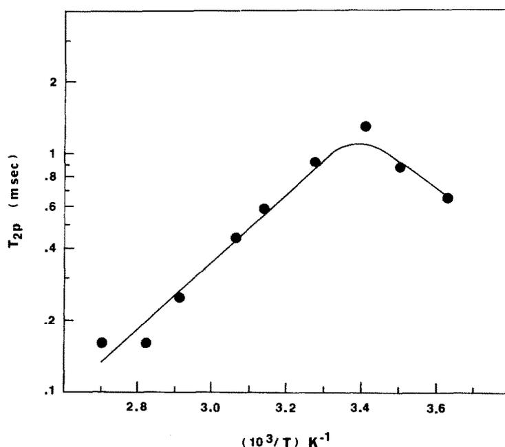
Fig. 12. Dependence of the  $^{14}\text{N}$  paramagnetic transverse relaxation time of proline upon inverse temperature, for a solution containing 1.5 M proline and 2.0 mM  $\text{CuCl}_2$  (Solution H), at pH 11. The spectrometer frequency was 18.075 MHz.
