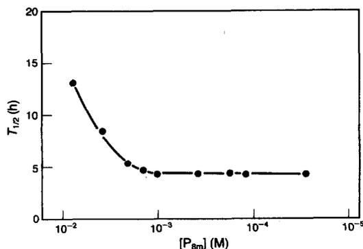
Fig. 1. Concentration dependence of half-life period of cyclo-octaphosphate hydrolysis in 0.1 M HCl at  $40^\circ\text{C}$ .
