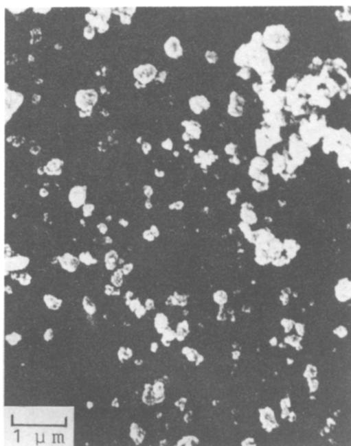
Fig. 1. Scanning electron micrograph for starting powder.
