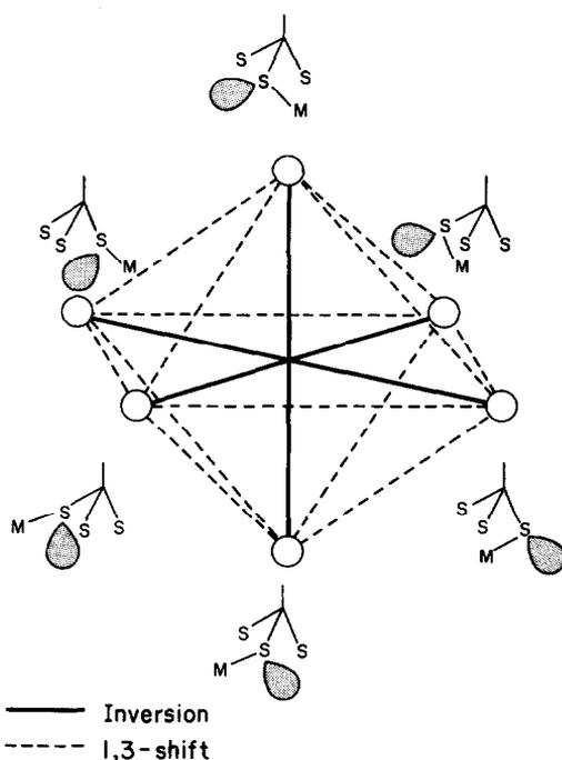
Fig. 4. Graph diagram illustrating the six topomers of  $[\text{M}(\text{CO})_5(\text{CH}_3\text{S})_3\text{CH}]$  and their exchange pathways.
