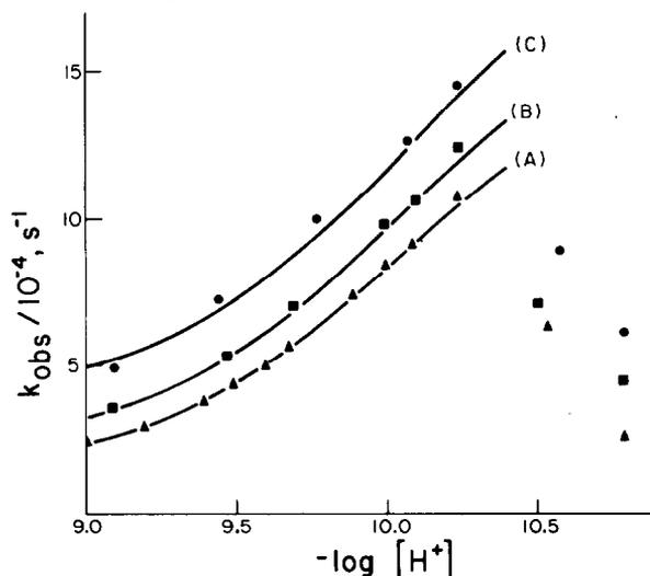
Fig. 2. Dependency of the rate constants on the pH of the medium. Solid lines represent the calculated values from eqn (5) at different pH values; the solid values are those obtained experimentally. (A) 30°C; (B) 35°C; (C) 40°C.
