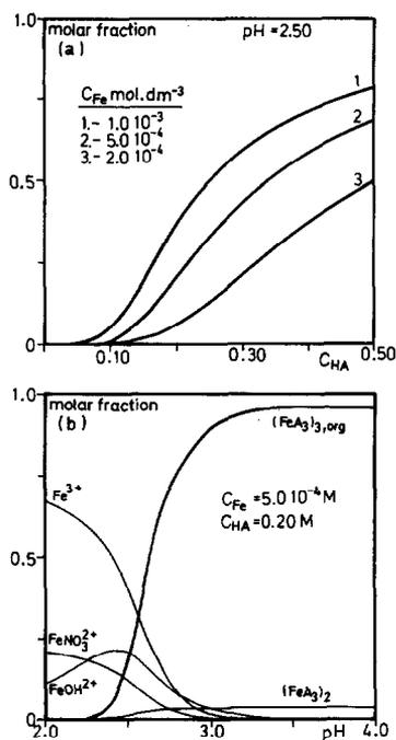
Fig. 7. Distribution diagrams in the system Fe(III)-NaNO<sub>3</sub>/HA-toluene. (a) Molar fraction of the trimer, (FeA<sub>3</sub>)<sub>3</sub>, in the organic phase as a function of C<sub>HA</sub> at constant pH and different total metal concentration. (b) Molar fraction of the main species in both phases as a function of pH at constant metal and *n*-dodecanoic acid concentration.
