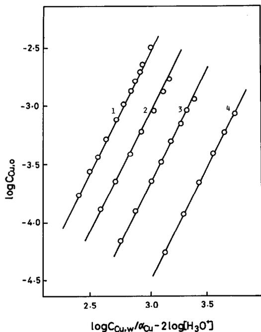
Fig. 3. Identification of the degree of polymerization of Cu(II)  $\alpha$ -bromovalerate extracted in benzene. Aqueous ionic strength: 1.0 (Na,H)ClO<sub>4</sub>.  $C_{HA,o}$  (mol dm<sup>-3</sup>): (1) 0.93, (2) 0.70, (3) 0.45, and (4) 0.23.
