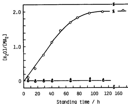
Fig. 5. Hydration of the divalent metal chelates under a constant vapor pressure of water (9.76 mmHg) at 25°C.  $\circ$  Ni(tta)<sub>2</sub>;  $\bullet$  Cu(tta)<sub>2</sub>;  $\diamond$  Ni(dmdtc)<sub>2</sub>;  $\blacklozenge$  Cu(dmdtc)<sub>2</sub>.
