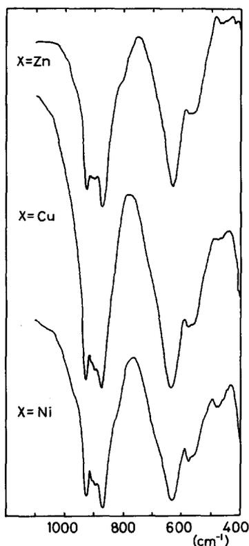
Fig. 2. Solid IR spectra of Anderson-type  $[X(\text{II})\text{Mo}_6\text{O}_{24}\text{H}_6]^{4-}$  polyanions.
