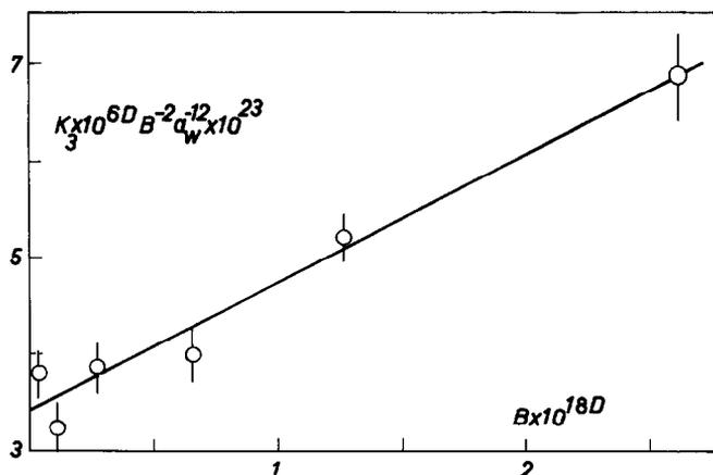
Fig. 3.  $K_3 B^{-2} \alpha_w^{-12} \times 10^{6D}$  [eqn (15)] as a function of  $B \times 10^{18D}$ . The straight line was calculated with:  $3.39 \times 10^{-23} + 1.26 \times 10^{-23} B \times 10^{18D}$ .
