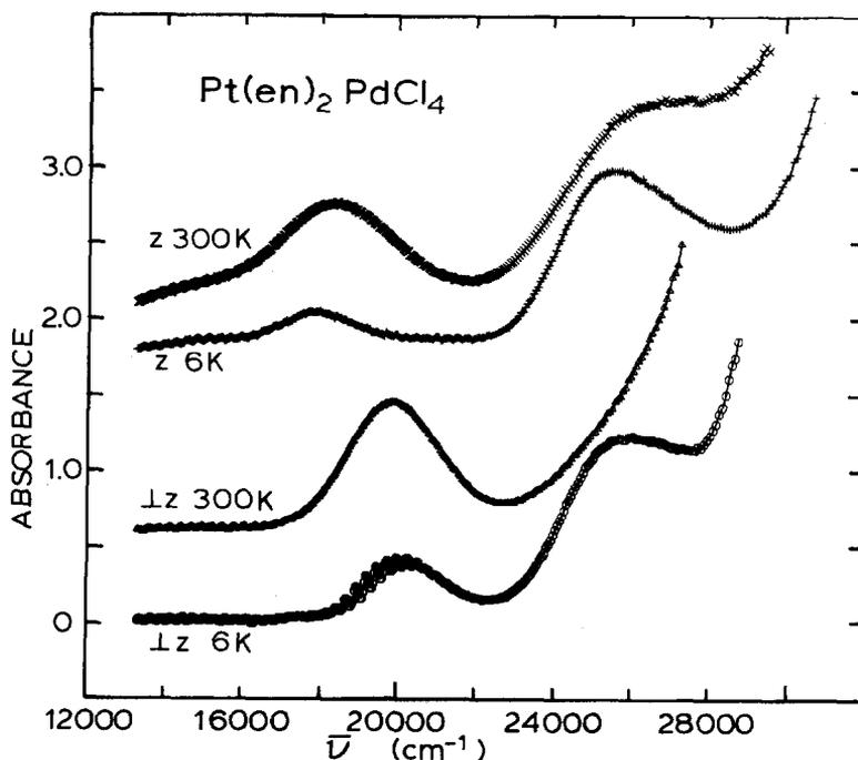
Fig. 14. Polarized spectra for  $\text{Pt}(\text{en})_2\text{PdCl}_4$  crystal,  $8 \mu\text{m}$  thick.
