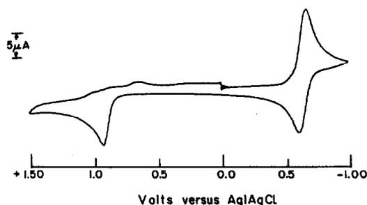
Fig. 1. Cyclic voltammogram of Os<sub>2</sub>(fhp)<sub>4</sub>Cl (measured at 200 mV s<sup>-1</sup> in 0.2 M TBAH-CH<sub>2</sub>Cl<sub>2</sub> at a Pt-disk electrode).
