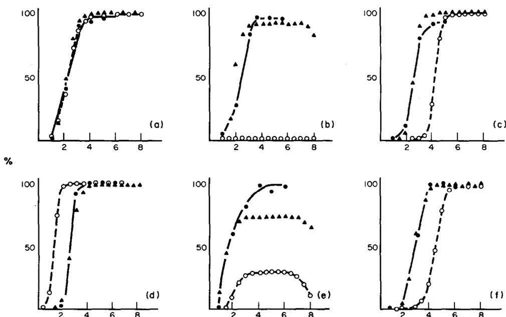
Fig. 2. (a) Experimental and computed percent recovery yield for Pb(II) onto NTA filters as a function of pH: (●) experimental, (○) computed with literature stability constants  $\beta$  of Table 3, (▲) computed with the apparent stability constants  $*\beta$  of Table 3. (b) Pb(II), THIO filters; (c) Pb(II), CYS filters; (d) Cu(II), NTA filters; (e) Cu(II), THIO filters; (f) Cu(II), CYS filters.
