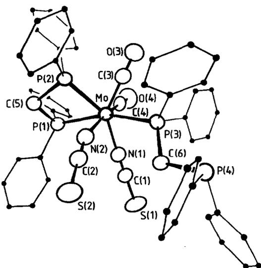
Fig. 1. Molecular structure of  $[\text{Mo}(\text{CO})_2(\text{NCS})_2(\text{dppm-PP}')(\text{dppm-P})]$ , showing the principal atomic numbering.
