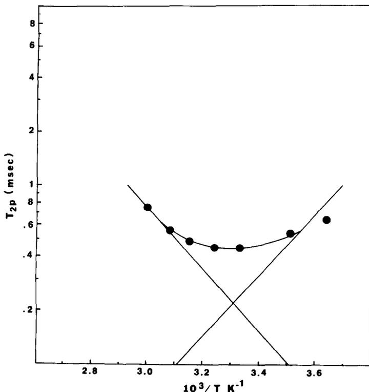
Fig. 5. Dependence of the  $^{17}\text{O}$  paramagnetic transverse relaxation time of glycine upon inverse temperature at pH 3, for a solution containing 0.115 M glycine and 5.0 mM  $\text{CoCl}_2$  (Solution B). The data were recorded at 24.4 MHz.
