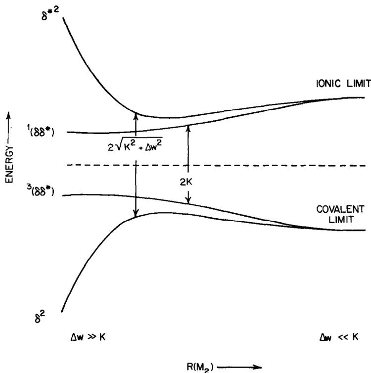
Fig. 1. Dependence of the energies of the  $\delta, \delta^*$ -manifold of electronic states upon metal-metal distance.
