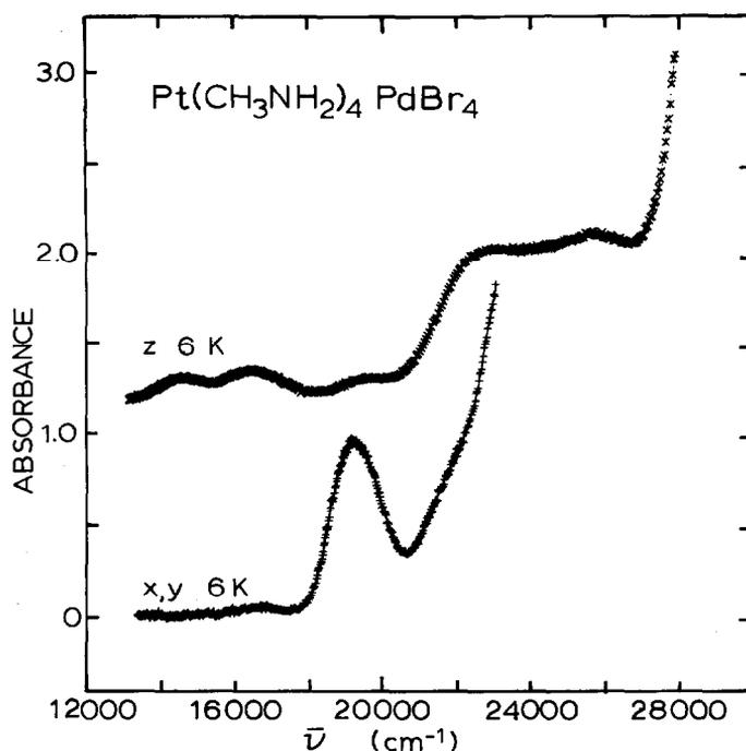
Fig. 20. Polarized spectra for  $\text{Pt}(\text{CH}_3\text{NH}_2)_4\text{PdBr}_4$  crystal, 13  $\mu\text{m}$  thick.
