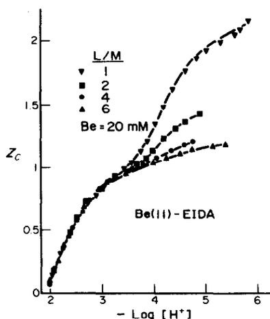
Fig. 2.  $Z_c$  vs  $-\log[H^+]$  curves of the EIDA-Be(II) system. Full curves = calculated curves (Model "FONDO +  $[\text{Be}(\text{OH})\text{C}]^-$ ", using  $\beta_{-311}$  in Table 3).
