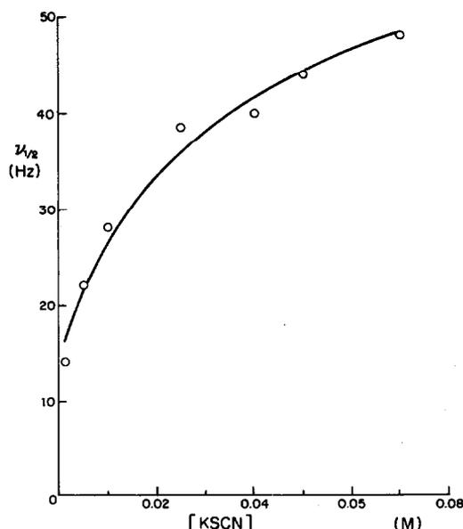
Fig. 3. K-39 linewidths of half-height as a function of the total KSCN concentration in nitromethane. The data points are experimental and the curve was calculated from the results of the non-linear regression analysis on eqns (2) and (3) applied to the linewidths.  $(\nu_{1/2})_{\text{F}} = 14$  Hz;  $(\nu_{1/2})_{\text{P}} = 87$  Hz. The RMS on the regression was 2.5 Hz.
