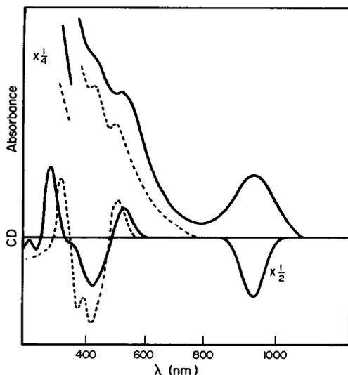
Fig. 10. Absorption and CD spectra of  $\Lambda$ -[Re<sub>2</sub>Cl<sub>4</sub>(S,S-dppb)<sub>2</sub>]<sup>2+</sup> (full line) and  $\Lambda$ -[Re<sub>2</sub>Cl<sub>4</sub>(S,S-dppb)<sub>2</sub>] (dashed line), both in dichloromethane solution.
