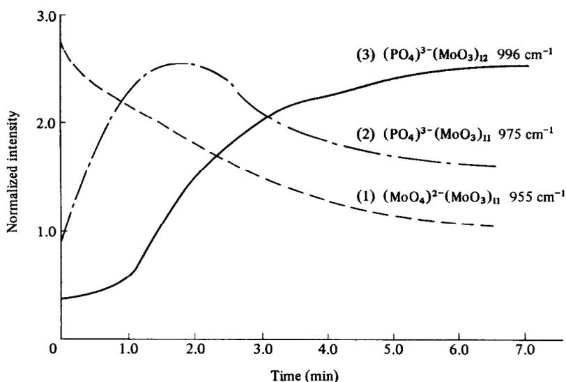
Fig. 2. Formation and decomposition curves of three species observed at each wavenumber. (1)  $(\text{MoO}_4)^{2-}(\text{MoO}_3)_{11}$  at  $955\text{ cm}^{-1}$ , (2)  $(\text{PO}_4)^{3-}(\text{MoO}_3)_{11}$  at  $975\text{ cm}^{-1}$ , (3)  $[\text{PMoO}_{40}]^{3-}$  at  $996\text{ cm}^{-1}$ .
