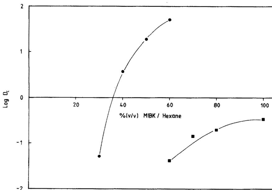
Fig. 1. Distribution coefficients ( $\log D_c$ ) of Pt(II) and Pd(II) between  $2.4 \text{ mol dm}^{-3}$  HCl and various mixtures of MIBK in *n*-hexane [% (v/v)], in the presence of excess tin(II) chloride at 295 K [ $\text{Sn(II)}$ ]:  $M = 10$  ( $M = \text{mol Pt} + \text{Pd}$ ).
