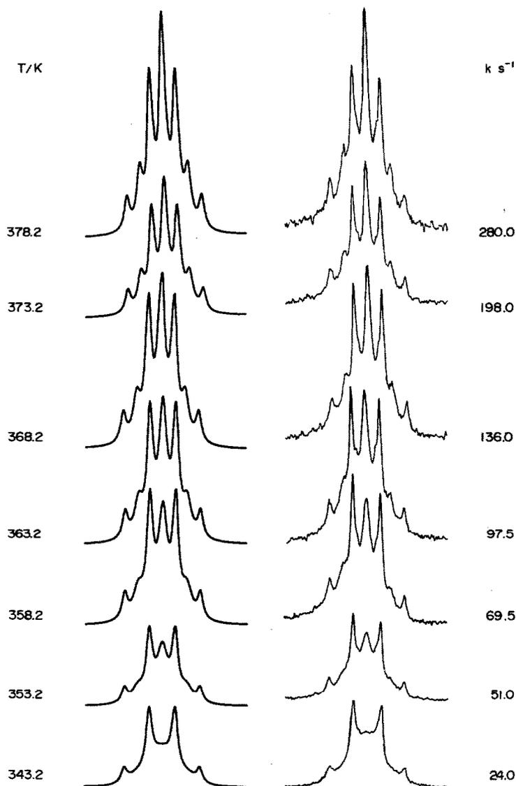
Fig. 6. Variable-temperature experimental and computer-simulated  $^1\text{H}$  NMR spectra of  $[\text{Pd}(\text{dppe})(\mu_2\text{-SMe})_2\text{PtClMe}_3]$  showing the effects of the rotation of the  $\text{Pd}(\text{dppe})$  moiety.
