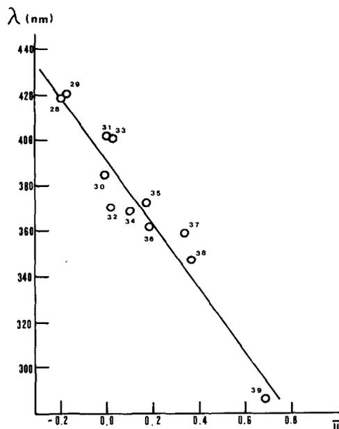
Fig. 4. Dependence from the  $\pi$ -acceptor capacity on  $\lambda_{\text{max}}$  for  $\text{W}(\text{CO})_5\text{L}$ .
