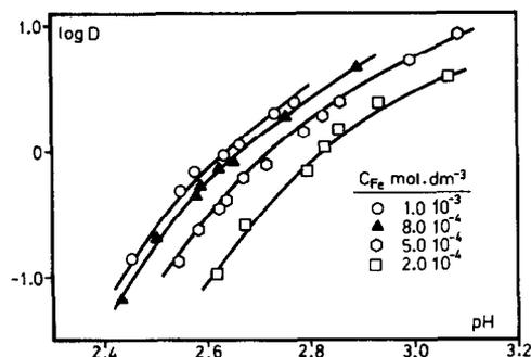
Fig. 2. The effect of total Fe(III) concentration on the extraction with *n*-dodecanoic acid at  $C_{\text{HA}} = 0.174 \times 10^{-3} \text{ mol dm}^{-3}$ . Continuous lines have been drawn using the equilibrium constants proposed in Table 2.
