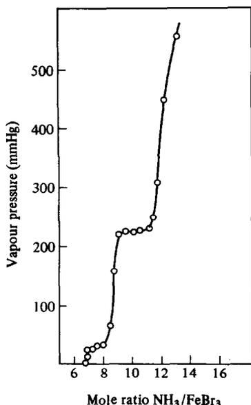
Fig. 2. Vapour pressure-composition isotherm for the  $\text{FeBr}_3\text{-NH}_3$  system at  $-36^\circ\text{C}$ .
