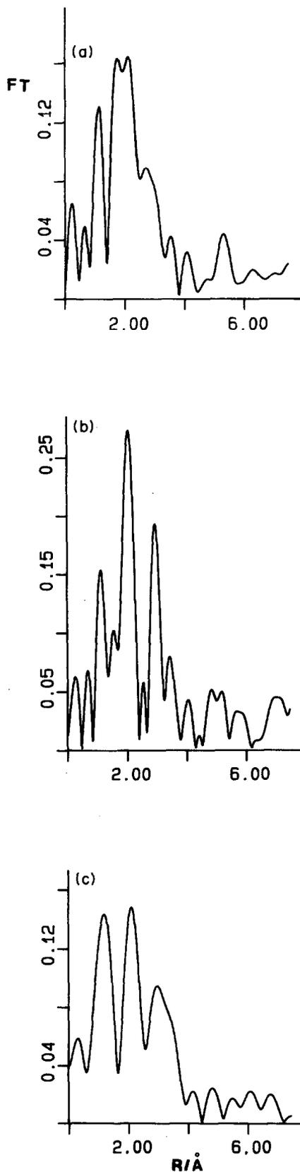
Fig. 4. Fourier transforms of EXAFS oscillations for: (a)  $\text{U}(\text{BH}_4)_4$ , (b)  $\text{U}_3(\text{BH}_4)_9(18\text{-crown-6})_2$ , and (c)  $\text{U}_3(\text{BH}_4)_9(\text{dbc})_2$ .
