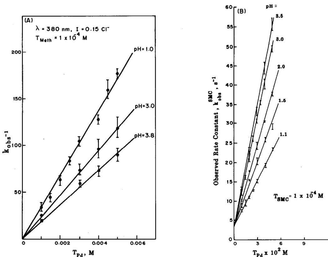
Fig. 2. Dependence of the observed rate constants on pH for: (A) the Pd(II)-Meth system, and (B) the Pd(II)-SMC system.
