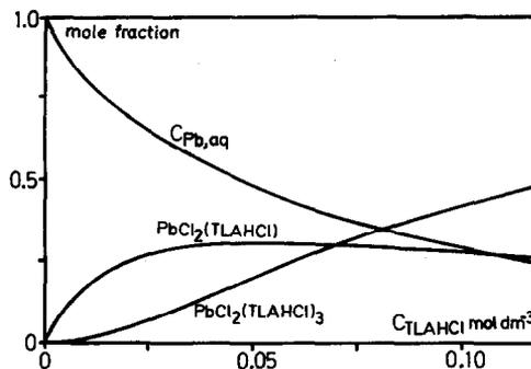
Fig. 7. Distribution diagram of Pb(II) species in the system Pb(II)-Cl<sup>-</sup>/TLAHCl-benzene at pH = 2.00.
