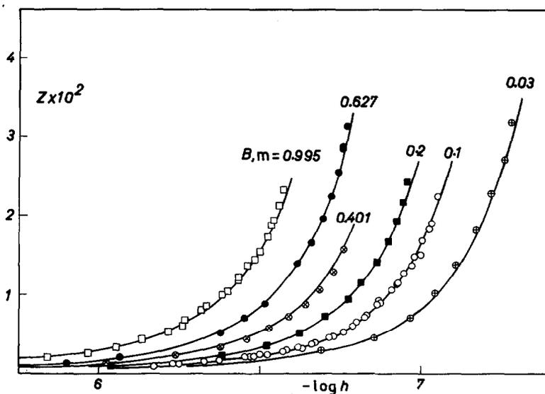
Fig. 1.  $Z$ , the average number of  $\text{OH}^-$  bound per lanthanum atom, as a function of  $\log h$ . The curves were calculated using the constants given in Table 3 and expressions (12) and (13) for medium changes.
