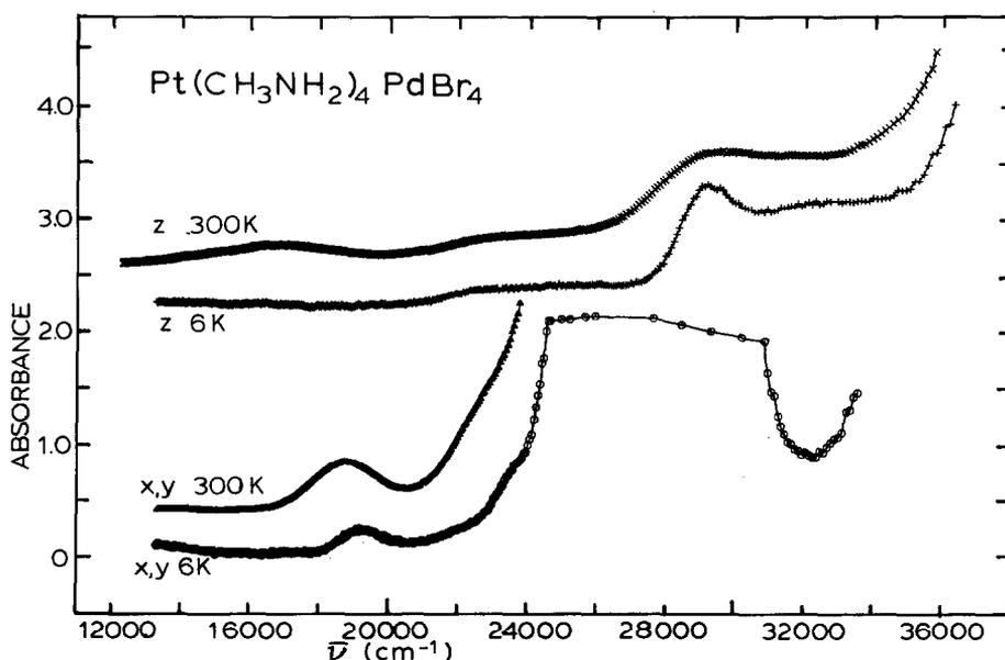
Fig. 21. Polarized spectra for  $\text{Pt}(\text{CH}_3\text{NH}_2)_4\text{PdBr}_4$  crystal, 3  $\mu\text{m}$  thick.
