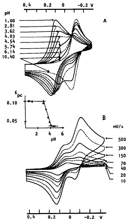
Fig. 4. Cyclic voltammograms of the ruthenium(III)/(II)-(edta) complexes of 2-mercaptopyridine (5 mM,  $I = 0.10 \text{ M}$  Lipts,  $25^\circ\text{C}$ ) at several pHs (scan rate =  $0.10 \text{ V s}^{-1}$ ) and at several potential scan rates (pH = 4.43). The internal plot illustrates a typical dependence of  $E_{1/2}$  versus pH for the red species.
