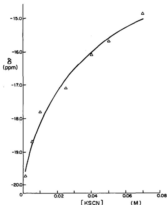
Fig. 2. K-39 chemical shifts as a function of the total KSCN concentration in nitromethane. The data points are experimental and the curve was calculated from the results of the non-linear regression analysis on eqns (2) and (3).  $K_p = 24$ ;  $\delta_p = -9.7$  ppm and  $\delta_f = -19.8$  ppm; RMS of the fit is equal to 0.3 ppm.
