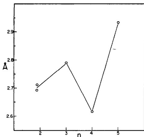
Fig. 4. M-M distances for a series of  $M_2Cl_6(\mu\text{-dppm})_2$  or  $M_2Cl_6(\mu\text{-dmpm})_2$  compounds covering  $d^n\text{-}d^n$  interactions from  $n$  from 2 to 5. The two points for  $n = 2$  are for Nb and Ta compounds.
