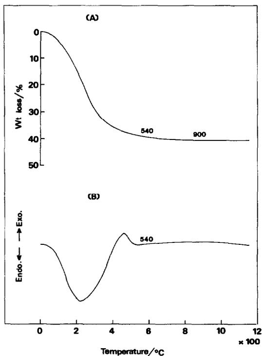
Fig. 3. (A) TG and (B) DTA curves for starting powder.
