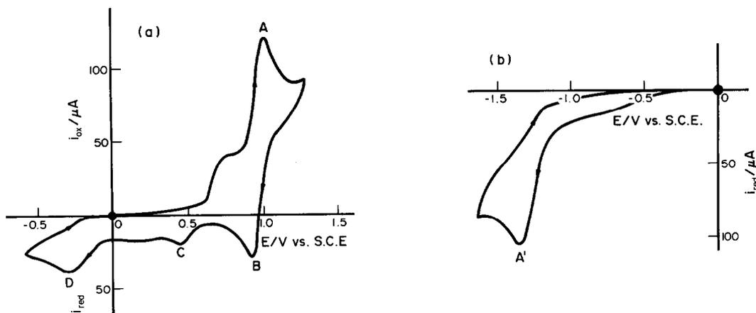
Fig. 1. Cyclic voltammograms recorded with a platinum working electrode on a  $4.8 \times 10^{-3}$  M  $n\text{Bu}_4\text{N} [\text{ReOCl}_3(\text{HOPhSal})]$ , 0.1 M tetraethylammonium tetrafluoroborate, MeCN solution. Potential scan rate  $0.2 \text{ V s}^{-1}$ . ●, Starting potential; (a) anodic direct scan; (b) cathodic direct scan.
