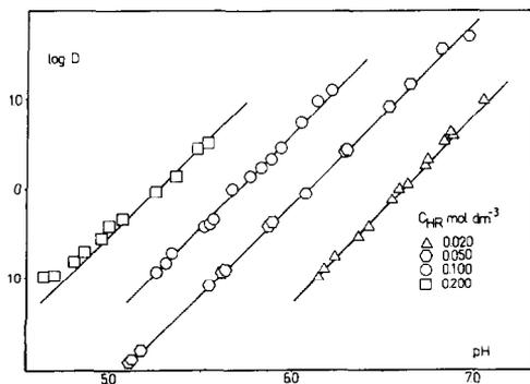
Fig. 1. Variation of the distribution coefficient of Ni(II) with pH at several total concentrations of di-*n*-octylphosphinic acid (HR). Continuous lines represent the normalized function  $\log D = f(\log V)_p$  in the best-fit position ( $p = 2$ ).
