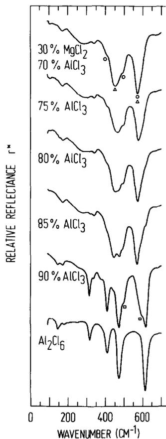
Fig. 4. IR reflectance spectra of molten mixtures in the  $\text{MgCl}_2$ - $\text{AlCl}_3$  system at 260–200°C. ( $\Delta$ )  $\text{AlCl}_4^-$  ( $C_{3v}$ ), ( $\circ$ )  $\text{AlCl}_4^-$  ( $C_{2v}$ ), and ( $\square$ )  $\text{Al}_2\text{Cl}_7^-$ .
