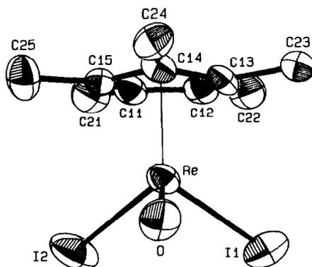
Fig. 7. The diiodo derivative ( $\eta^5\text{-C}_5\text{Me}_5$ )ReOI<sub>2</sub> (**3d**): ORTEP representation, with the thermal ellipsoids being at 50% probability. Selected bond lengths (pm) and angles (°): Re—O 168.7(3), Re—I(1) 268.1(<1), Re—I(2) 267.6(<1), Re—C(11) 253.5(4), Re—C(12) 251.7(4), Re—C(13) 223.7(4), Re—C(14) 218.6(4), Re—C(15) 225.4(4); I(1),Re,I(2), 88.8(<1), I(1),Re,O 99.4(1), I(2),Re,O 101.7(4). The sum of angles within the ReOI<sub>2</sub> core amounts to 289.9°.
