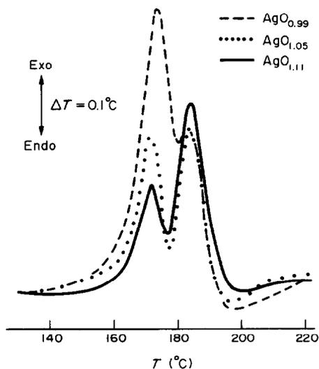
Fig. 3. Differential thermal analysis of tetragonal AgO. Samples weight, 46 mg; heating rate,  $6^\circ\text{C min}^{-1}$ ; atmosphere, static air.
