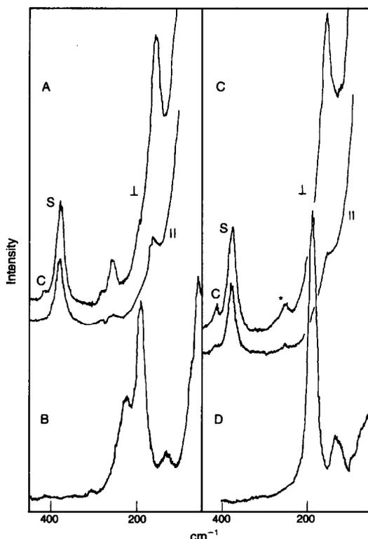
Fig. 2. Raman spectra of bromoselenate(II)s: (A)  $\text{Et}_4\text{NSeBr}_3$  in  $\text{CH}_3\text{CN}$  (0.09 M), (B) solid  $\text{Et}_4\text{NSeBr}_3$ , (C) 6 : 1  $\text{Et}_4\text{NBr}-\text{Et}_4\text{NSeBr}_3$  [ $C_{\text{Se(IV)}} = 0.09 \text{ M}$ ], and (D) solid  $(\text{Et}_4\text{N})_2\text{SeBr}_4$ . S = solvent band; c = cation band; \* =  $\text{SeBr}_3^-$  band.
