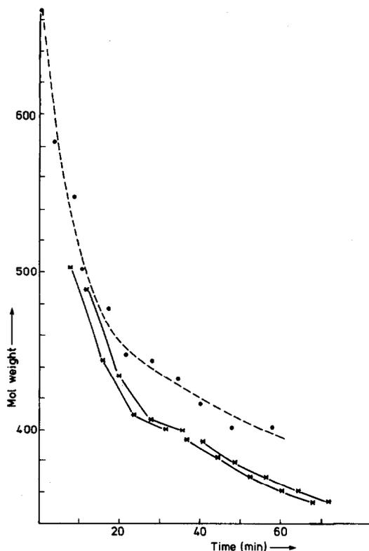
Fig. 4. The change in molecular weight in time of a solution of I in  $\text{CHCl}_3$  using VPO (\*) and in  $\text{CDCl}_3$  using  $^1\text{H-NMR}$  (●).
