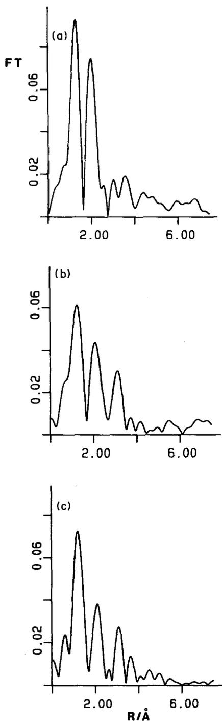
Fig. 3. Fourier transforms of EXAFS oscillations for: (a)  $\text{UO}_2(\text{CH}_3\text{COO})_3\text{Na}$ , (b)  $\text{UO}_2(18\text{-crown-6})(\text{ClO}_4)_2$  (solid), and (c)  $\text{UO}_2(18\text{-crown-6})(\text{ClO}_4)_2$  (solution in  $\text{CH}_3\text{CN}$ ).
