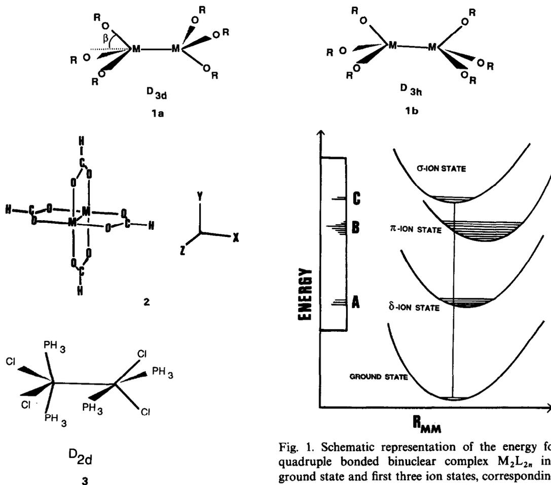
Fig. 1. Schematic representation of the energy for a quadruple bonded binuclear complex  $M_2L_{2n}$  in its ground state and first three ion states, corresponding to ionizations out of the  $\sigma$ ,  $\pi$  and  $\delta$  bonding orbitals, as a function of the metal-metal bond distance ( $R_{MM}$ ). Schematic representation of the three first PE bands with expected shapes are given as A, B and C, respectively.
