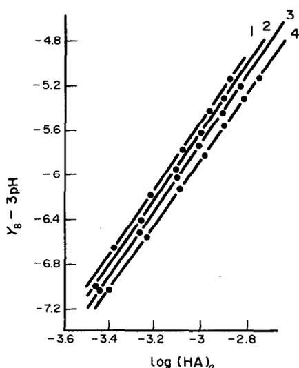
Fig. 4. Synergic extraction of Nd(III) with various  $C_{HA}$  and constant  $C_B$  in different organic solvents: (1) xylene, (2) toluene, (3) benzene, and (4) CCl<sub>4</sub>.  $C_B = 1 \times 10^{-4}$  M,  $Y_B = \log D - \log (B)_o$ .
