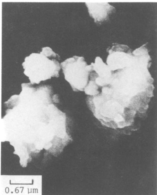
Fig. 7. Scanning electron micrograph for spinel powder.
