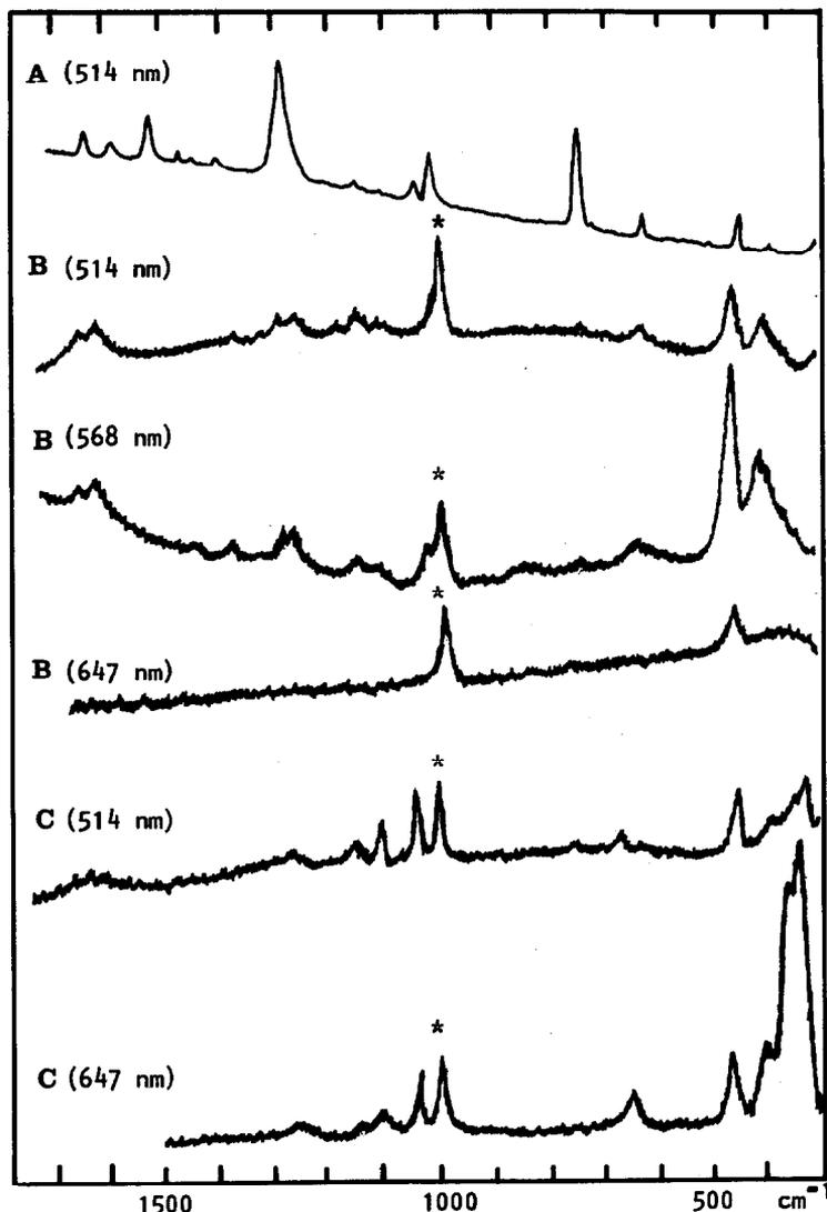
Fig. 3. (A) Raman spectra of the 2-mercaptopyridine ligand in the solid state, and (B) of aqueous solutions of the red (0.5 mM), and green Ru(III) complex (1 mM), at several excitation wavelengths, in the presence of 0.10 M sodium sulfate (\* = sulfate band).
