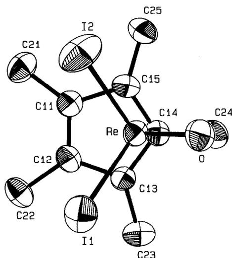
Fig. 9. Projection of compound **7a**'s molecular structure viewed down onto the best plane of the  $\pi$ -bonded pentamethylcyclopentadienyl ligand.
