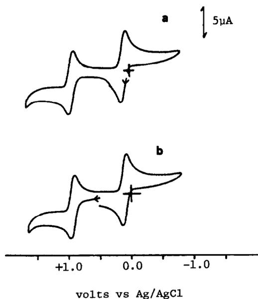
Fig. 1. Cyclic voltammograms (recorded at  $v = 200$   $\text{mV s}^{-1}$  using a Pt-bead electrode) for 0.1 M TBAH- $\text{CH}_2\text{Cl}_2$  solutions of: (a)  $\beta\text{-Re}_2\text{Cl}_4(\text{depe})_2$ , and (b)  $\beta\text{-[Re}_2\text{Cl}_4(\text{depe})_2\text{]PF}_6$ .
