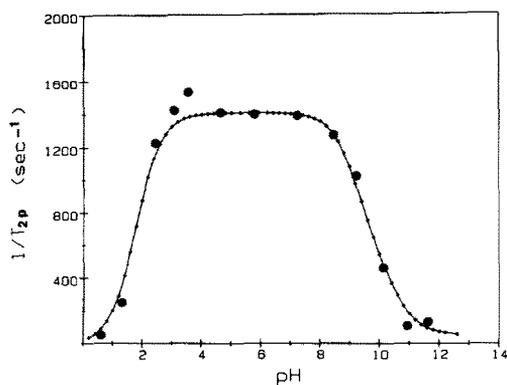
Fig. 13. Dependence of the  $^{17}\text{O}$  paramagnetic transverse relaxation rate of proline upon the measured pH of a solution containing 0.08 M proline and 0.34 mM  $\text{MnCl}_2$  (Solution I), at 300 K. The experimental points were recorded at 24.4 MHz and the dotted line is the least-squares fit of the experimental points to eq. (28), with the constants of Tables 5 and 6.
