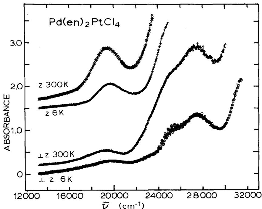
Fig. 7. Polarized spectra for  $\text{Pd}(\text{en})_2\text{PtCl}_4$  crystal,  $26 \mu\text{m}$  thick.
