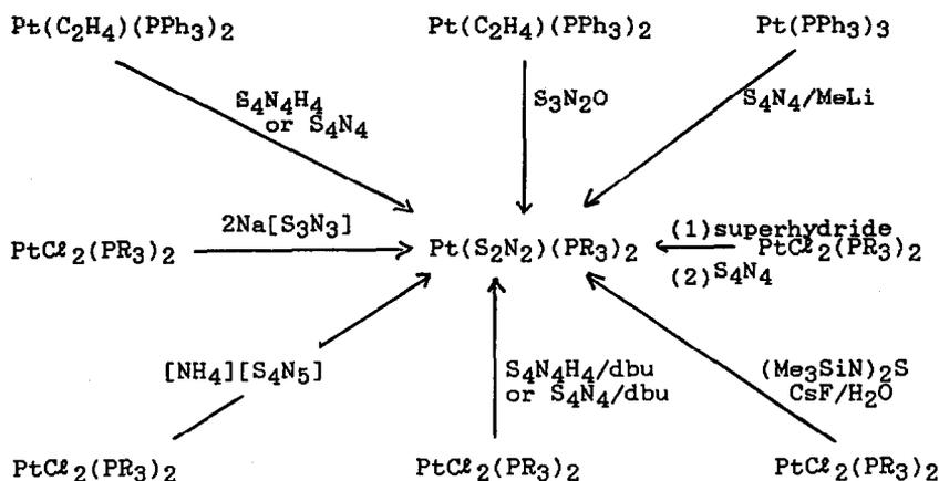
Scheme 1. Reactions in which  $\text{Pt}(\text{S}_2\text{N}_2)(\text{PR}_3)_2$  is a major product. Note that in some cases the results are from  $^{31}\text{P}$  NMR only.
