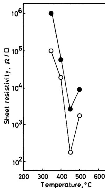
Fig. 2. Relation between sheet resistivities of ITO films prepared from  $\text{Bu}_2\text{In}(\text{O}_2\text{CCH}(\text{Et})(\text{CH}_2)_3\text{CH}_3)$  with or without  $\text{Bu}_2\text{SnO}$  and baking temperature; solvent was *p*-xylene and the dibutylindium octanoate concentration was kept at 5 wt %. The  $\text{Bu}_2\text{SnO}$  content varied between 0 (●) and 2 wt % (○), with respect to the indium compounds.
