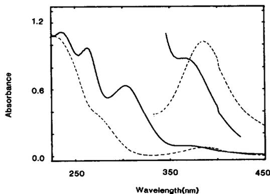
Fig. 3. Comparison of the electronic absorption spectra of  $Mo_2(CH_2Bu^t)_6$  (solid line) and  $W_2(CH_2Bu^t)_6$  (dashed line) in THF solutions, at  $5.7 \times 10^{-4}$  and  $5.7 \times 10^{-5}$  M.
