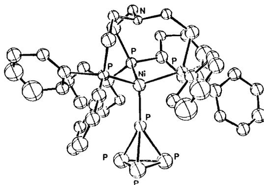
Fig. 2. Structure of the  $[(np_3)(\eta^1-P_4)]$  molecule.
