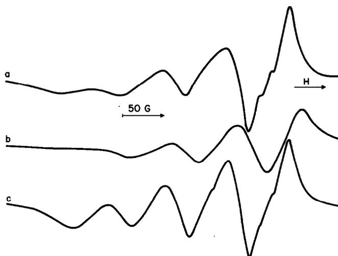
Fig. 1. ESR spectra of Cu(sal-glycine) at 295 K. (a) in 3 : 2 dioxane-H<sub>2</sub>O (*L*), (b) after addition of *L*<sub>1</sub> = pyridine (0.01 M) to the 3 : 2 dioxane-H<sub>2</sub>O (*L*) solution, (c) in pyridine (*L*).
