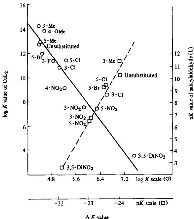
Fig. 2. Plot of calculated binding energies vs experimental proton ionization constants (pK) and stability constants (log K) for substituted salicylaldehydes and their bis complexes with copper.
