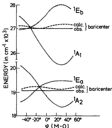
Fig. 5. Variation of energy levels with M–O torsional angle in *fac*- $\text{Co}(\beta\text{Ala})_3$  having  $C_3$  molecular symmetry. Zero torsional angle is defined for a conformation in which the  $p$ -orbital on the oxygen donor is perpendicular to the plane defined by the O, M and N of that ring.
