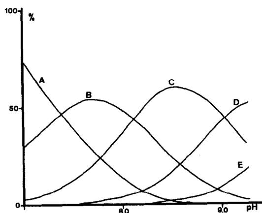
Fig. 1. Variation with pH of the distribution of the several species present in aqueous solution of Ni(II)-MEA  $I = 0.70$ : (A) Ni(II), (B) Ni-MEA, (C) Ni-(MEA)<sub>2</sub>, (D) Ni-(MEA)<sub>3</sub>, (E) Ni-(MEA)<sub>4</sub>.
