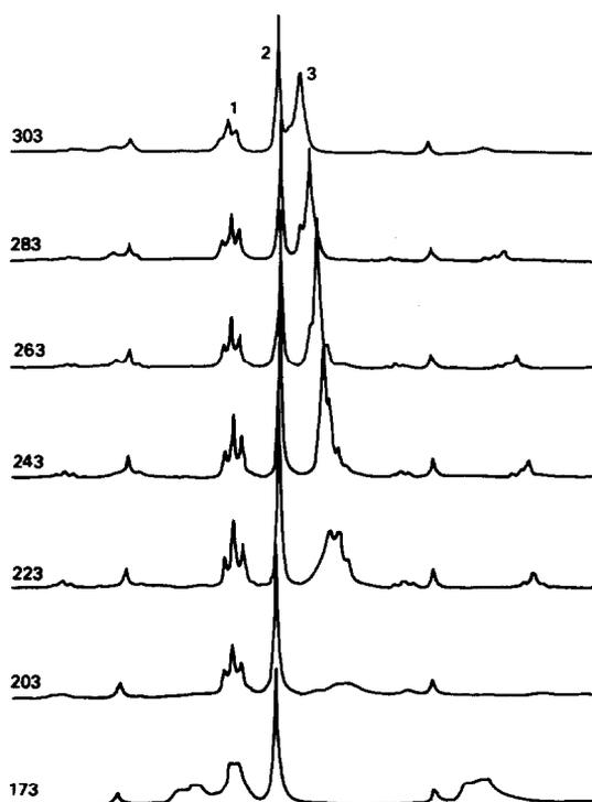
Fig. 1.  $^{31}\text{P}\{-^1\text{H}\}$  NMR spectra of a solution of  $[\text{Hg}(\text{Me}_2\text{SO})_6](\text{O}_3\text{SCF}_3)_2$ , dppm and dppe in a ratio of 1:1:1 in  $\text{CH}_2\text{Cl}_2$  at different temperatures (in K): (1) dppe part of  $[\text{Hg}(\eta^1\text{-dppm})(\eta^2\text{-dppe})]^{2+}$ , (2)  $[\text{Hg}(\eta^2\text{-dppe})_2]^{2+}$ , and (3) dppm part of  $[\text{Hg}(\eta^1\text{-dppm})(\eta^2\text{-dppe})]^{2+}$  and  $[\text{Hg}(\eta^1\text{-dppm})_2]^{2+}$ .
