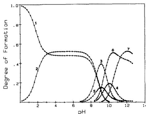
Fig. 14. Dependence of the relative concentration of all  $\text{Mn}^{2+}$  containing species upon pH, for Solution I, at 300 K. All curves were constructed with the stability constants of Table 5. 1 is the free  $\text{Mn}^{2+}$ , 2, 3, and 4 are the protonated complexes  $\text{MnHPro}^{2+}$ ,  $\text{MnHPro}_2^+$  and  $\text{MnHPro}_3$ , respectively, whereas 5, 6 and 7 are the bidentate complexes  $\text{MnPro}^+$ ,  $\text{MnPro}_2$  and  $\text{MnPro}_3^-$ , respectively.
