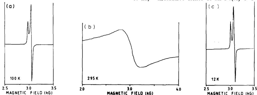
Fig. 7. Polycrystalline EPR spectra for [Fe(salophen)]NO. The sample temperatures are indicated.
