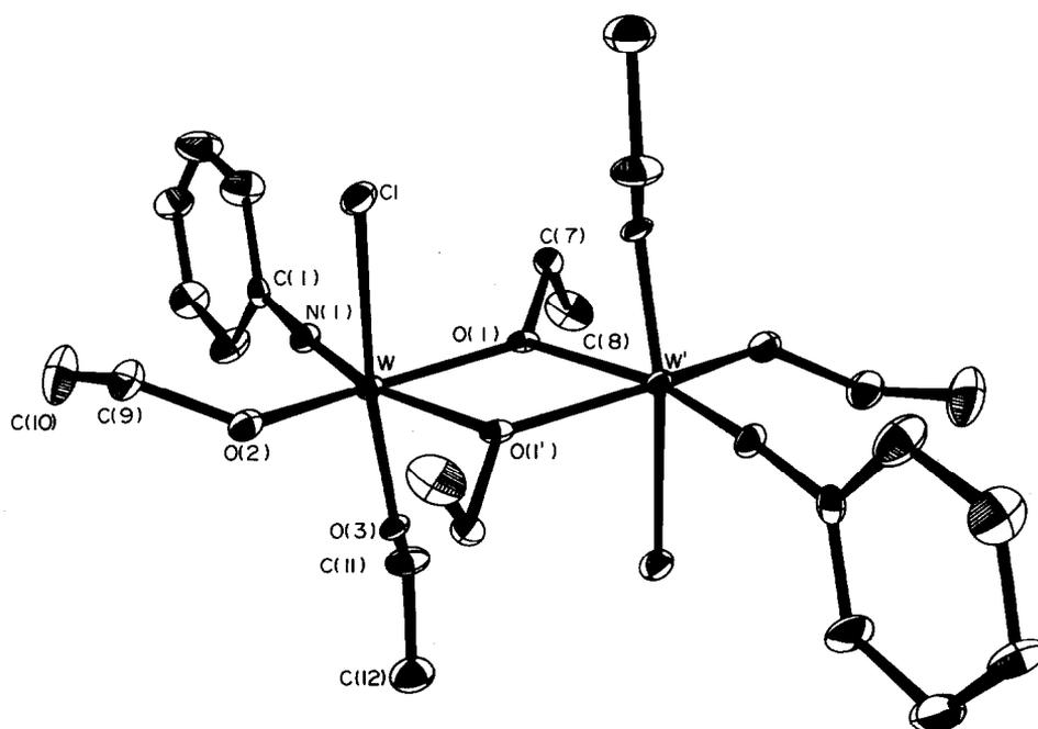
Fig. 1.  $[\text{W}(\text{NPh})(\mu\text{-OEt})(\text{OEt})_2\text{Cl}]_2$  molecule. Thermal ellipsoids have been drawn at the 50% probability level. Hydrogen atoms have been omitted for clarity.
