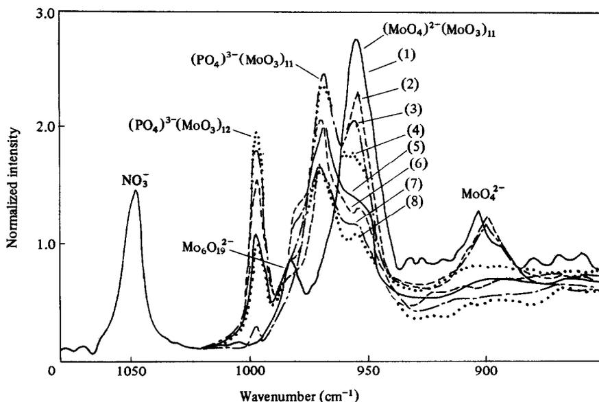
Fig. 1. The reaction of the acidified molybdate with the acidified phosphate solution on Raman spectra ( $[\text{P}] = 1.0 \times 10^{-2}$  M,  $[\text{Mo}] = 1.2 \times 10^{-1}$  M, pH 1). The reaction time: (1) 0 s, (2) 31 s, (3) 1 min 23 s, (4) 2 min 14 s, (5) 3 min 5 s, (6) 4 min 47 s, (7) 5 min 38 s, (8) 6 min 29 s.
