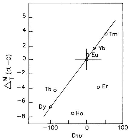
Fig. 1. A plot of the observed solution isotropic  $^{13}\text{C}$  NMR shifts at the  $\alpha$ -carbon of the cation,  $\Delta_T^M(\alpha\text{-C})$ , vs Bleaney factors  $D_{1M}$  for  $[(\text{C}_4\text{H}_9)_4\text{N}]_2\text{Ln}(\text{NO}_3)_5$  complexes. The data are taken from Table 1.
