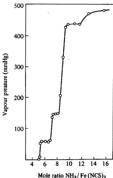
Fig. 1. Vapour pressure-composition isotherm for the  $\text{Fe}(\text{NCS})_2\text{-NH}_3$  system at  $-36^\circ\text{C}$ .
