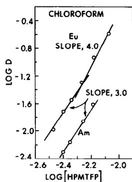
Fig. 3. Variation of  $\log D$  of trivalent Am and Eu as a function of HPMTPF concentration. Aqueous phase: pH 3.0 chloroacetate buffer. Org. phase: 0.0034–0.0085 M HPMTPF in chloroform.
