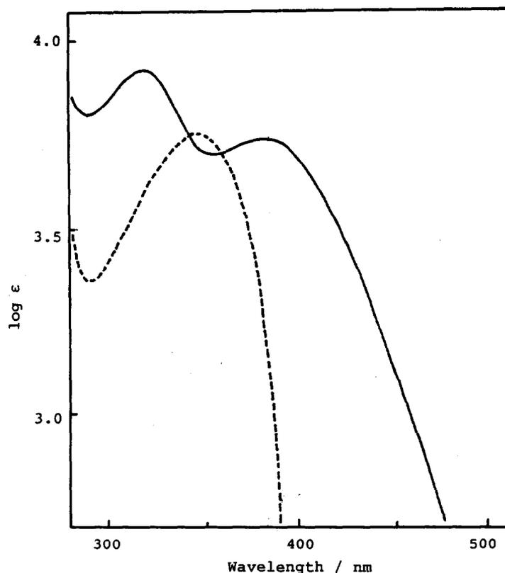
Fig. 2. Electronic absorption spectra of  $\text{ReBr(CO)}_3\text{Y}_p$  (—) in MeOH/EtOH (1:4 v/v) and of  $\text{Y}_p$  (---) in 2-MeTHF.
