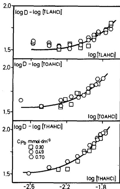
Fig. 6. Comparison between the experimental functions  $\log D - \log [R_3NHCl] = f(\log [R_3NHCl])$  and the theoretical  $\log Y = \log(1 + X^2) = f(\log X)$  in the best-fit positions.
