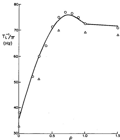
Fig. 4. K-39 transverse and longitudinal relaxation rates as a function of the ratio  $[DB30C10]/[KSCN]$  for  $[KSCN] = 0.025$  M.  $\circ$ : transverse relaxation data ( $i = 2$ );  $\triangle$ : longitudinal relaxation data ( $i = 1$ ). The data points are experimental and the curve was calculated following the values from Table 1.
