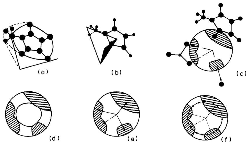
Fig. 1. Geometrical description of concepts of Cone Packing Model: (a) Solid Angle, (b) Fan Angle, (c) projection of ligands to the unit sphere, (d) hole among the ligands, (e) Coordination Vector ( $\vec{r}$ ), and (f) gap between two ligands.
