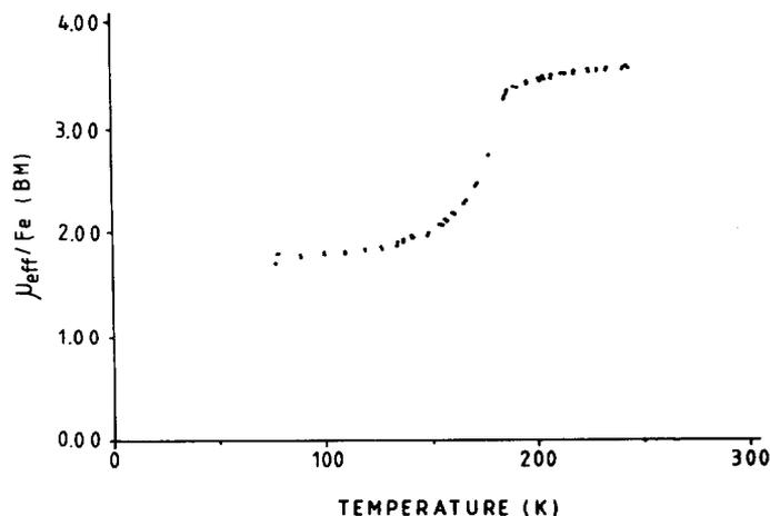
Fig. 2. Effective magnetic moment ( $\mu_{\text{eff}}$ ) for [Fe(salophen)NO] in the temperature range 80–300 K.
