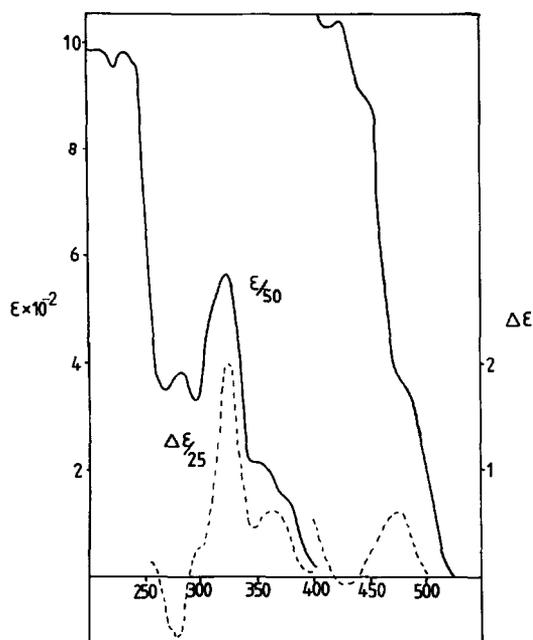
Fig. 1. Electronic absorption (—) and CD (----) spectra of [Crdbmpy<sub>3</sub>]<sup>3+</sup> in water.
