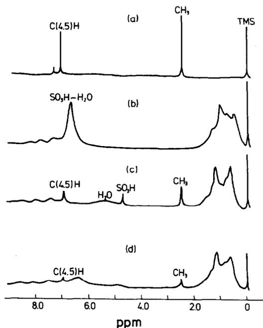
Fig. 7. NMR spectra. (a) 2MIm in CDCl<sub>3</sub>, (b) HD in CCl<sub>4</sub>, (c) organic phase after 2MIm in aqueous solution was extracted into HD in CCl<sub>4</sub>, (d) organic phase after 2MIm with HgCl<sub>2</sub> in aqueous solution was extracted into HD in CCl<sub>4</sub>.
