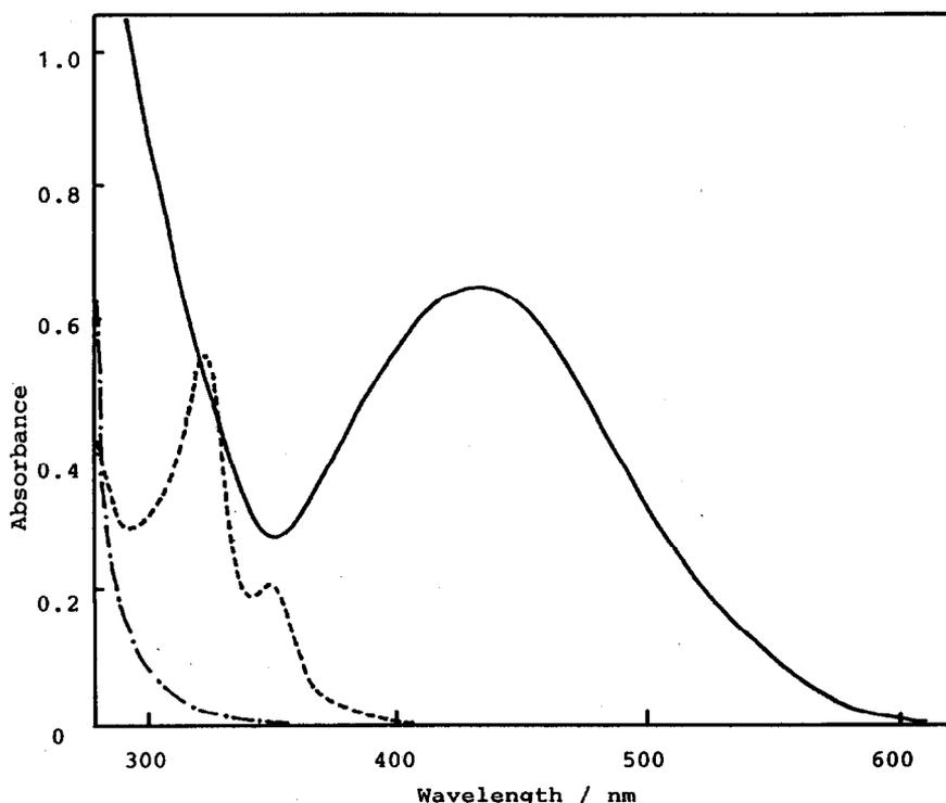
Fig. 1. Electronic absorption spectra of  $ReBr(CO)_3(2-AcPy)$  (—) in MeOH/EtOH (1:4 v/v),  $ReBr(CO)_5$  (---) and 2-AcPy (- · - ·) in MeCN at 298 K:  $3.0 \times 10^{-4}$  mol  $dm^{-3}$ .
