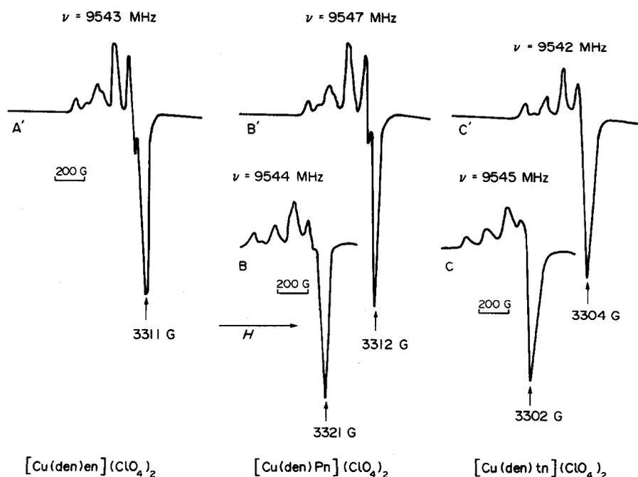
Fig. 2. ESR spectra of the mixed-ligand copper(II) complexes in frozen DMF (B and C) and pyridine (A', B' and C') solutions.
