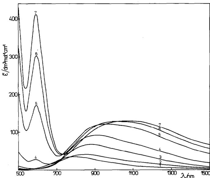
Fig. 1. Absorption spectra of Cu(ClO<sub>4</sub>)<sub>2</sub>-Et<sub>4</sub>NBr solutions in DMF at 25°C. The concentrations (mol dm<sup>-3</sup>) of Cu(ClO<sub>4</sub>)<sub>2</sub> and Et<sub>4</sub>NBr are, respectively: (1) 0.00519, 0.0; (2) 0.00513, 0.00247; (3) 0.00531, 0.00482; (4) 0.00556, 0.00729; (5) 0.00512, 0.00970; (6) 0.00513, 0.01213; (7) 0.00511, 0.01448.
