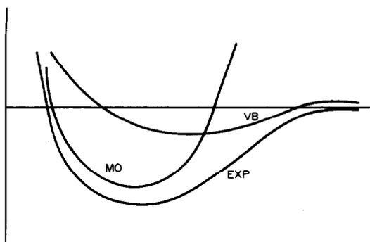
Fig. 1. Schematic potential energy curves are shown for a typical molecular orbital (MO) and valence bond (VB) wavefunction. In comparison with the "experimental" (EXP) curve, the MO wavefunction does not dissociate properly but parallels the EXP curve at short internuclear distances ( $R$ ), while the VB wavefunction dissociates properly but is too repulsive at shorter  $R$ .
