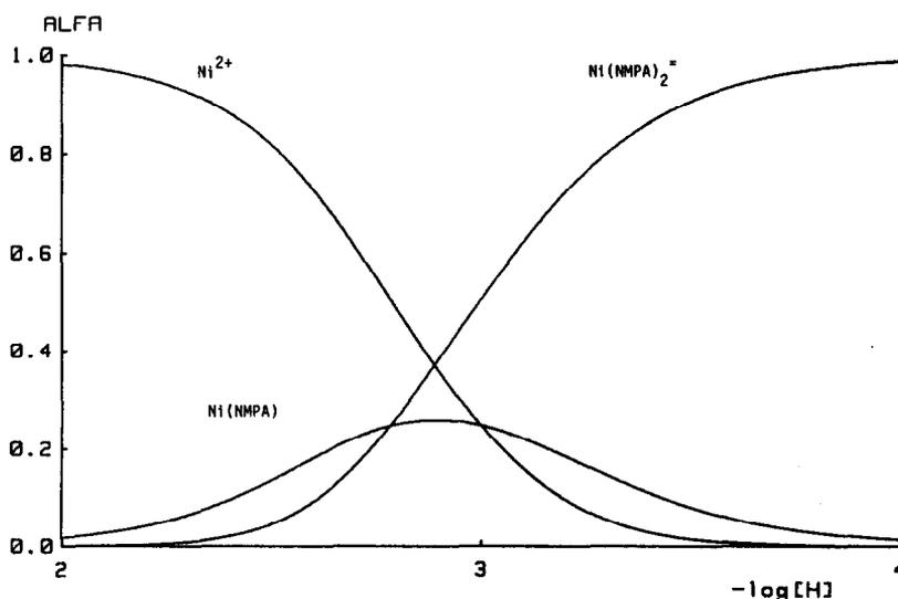
Fig. 4. Species distribution for Ni(II)-NMPA complexes.  $[Ni^{2+}] = 1 \text{ mM}$ ,  $[NMPA] = 3 \text{ mM}$ .
