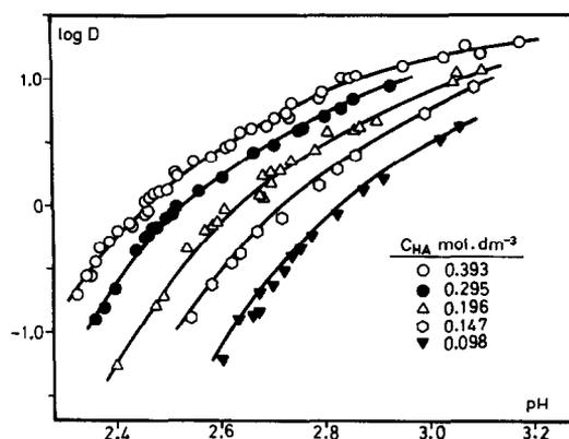
Fig. 1. Extraction of Fe(III) at various *n*-dodecanoic acid concentrations and  $C_{\text{Fe}} = 5.0 \times 10^{-4} \text{ mol dm}^{-3}$ . Continuous lines have been drawn using the equilibrium constants proposed in Table 2.
