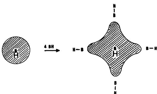
Fig. 2. Polarization of a BH unit's skeletal electron pair by four neighbouring skeletal boron atoms.
