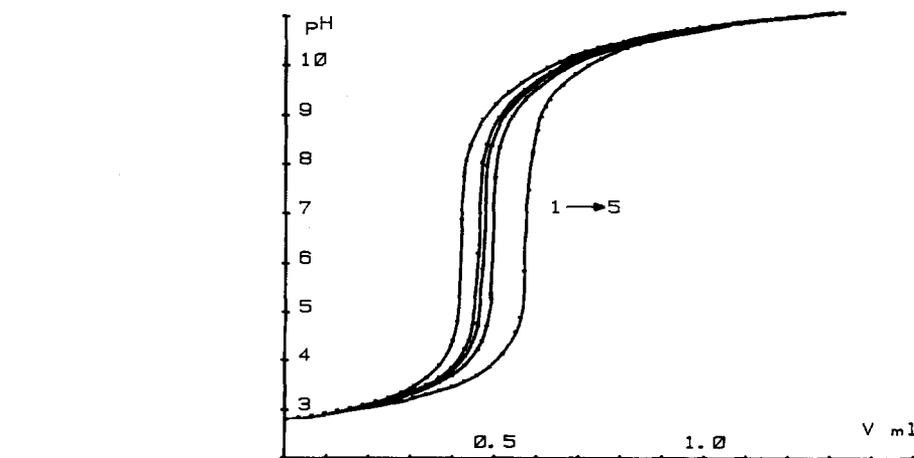
Fig. 2. Titration curves of PNML and PNML-Cu mixtures: 1, PNML; 2, PNML-Cu,  $R = 20$ ; 3, PNML-Cu,  $R = 15$ ; 4, PNML-Cu,  $R = 10$ ; 5, PNML-Cu,  $R = 5$ .
