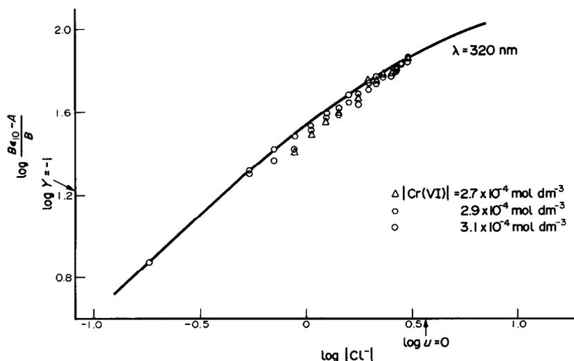
Fig. 1.  $-\log(B\epsilon_{10}-A)/B$  plotted vs  $\log[\text{Cl}^-]$  at  $\lambda = 320$  nm for different chromium(VI) concentration. The full drawn line gives  $\log Y$  as a function of  $\log u$  in the position of the best adjust.
