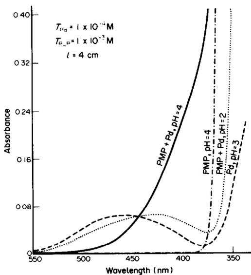
Fig. 5. Absorption spectra of Pd(II)-PMP system at various pH values.
