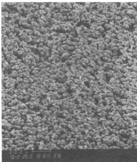
Fig. 4. Scanning electron microscope photography of tetragonal AgO.
