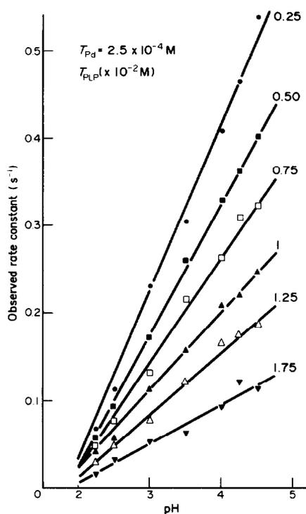
Fig. 2. Dependence of  $k_{\text{obs}}(\text{PLP})$  of Pd(II)-PLP system on pH at various  $T_{\text{PLP}}$  values.
