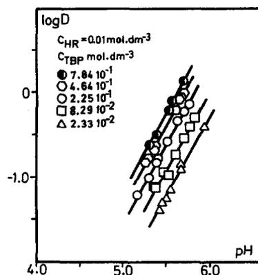
Fig. 1. log *D* vs pH for Cd(II) extraction at constant chelating reagent and different TOPO concentrations. Continuous lines were drawn using constants given in Table 1.
