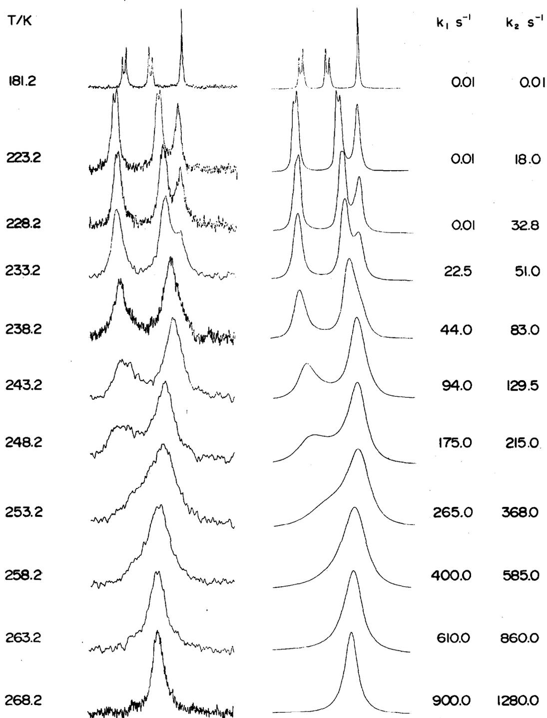
Fig. 4. Variable-temperature experimental and computer-simulated  $^{31}\text{P}$  NMR spectra of  $[\text{Pd}(\text{dppe})(\mu_2\text{-SMe})_2\text{PtBrMe}_3]$  showing the effects of pyramidal sulphur atom inversion.
