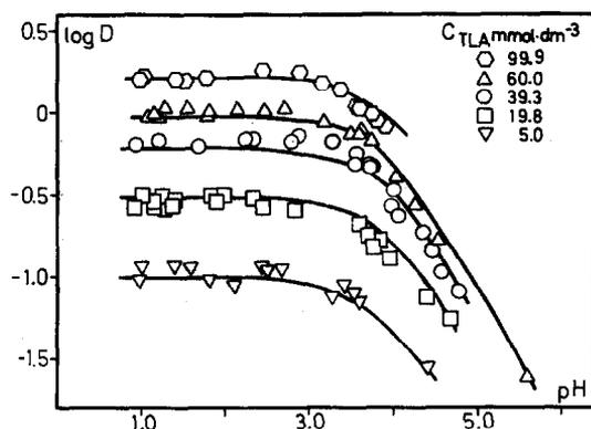
Fig. 1. Plot of  $\log D$  vs pH data for the different total concentration of TLA. The solid lines have been drawn using the proposed extraction constants.
