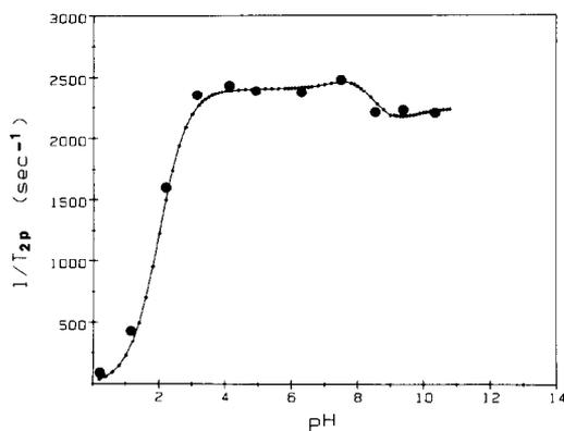
Fig. 12. Dependence of the  $^{17}\text{O}$  paramagnetic transverse relaxation rate of glycine upon the measured pH of a solution containing 0.20 M glycine and 0.6 mM  $\text{MnCl}_2$  (Solution I), at 300 K. The experimental points were recorded at 24.4 MHz and the dotted line is the least-squares fit of the experimental points to eqn (9), with the constants of Table 5.
