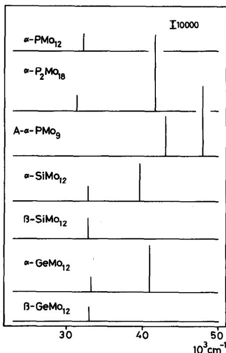
Fig. 5. Bar graphs of absorption maxima of a polyanion-group containing 'XM<sub>9</sub>O<sub>34</sub>' (X = P, Si, Ge) fragment. Height shows relative intensity and abscissa shows wavenumber.
