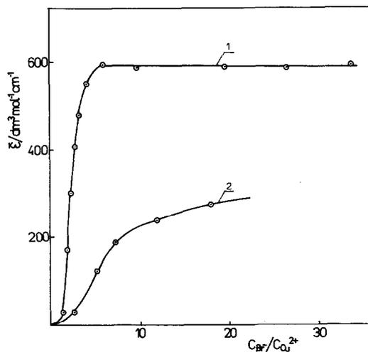
Fig. 3. Plots of the mean absorption coefficient of copper(II) against the  $C_{\text{Et}_4\text{NBr}}/C_{\text{Cu}(\text{ClO}_4)_2}$  ratio for  $\text{Cu}(\text{ClO}_4)_2\text{-Et}_4\text{NBr}$  solutions in DMF at  $25^\circ\text{C}$  for the isosbestic point at 587 nm. (1)  $C_{\text{Cu}(\text{ClO}_4)_2} = 0.005 \text{ mol dm}^{-3}$ , (2)  $C_{\text{Cu}(\text{ClO}_4)_2} = 0.00034$ .
