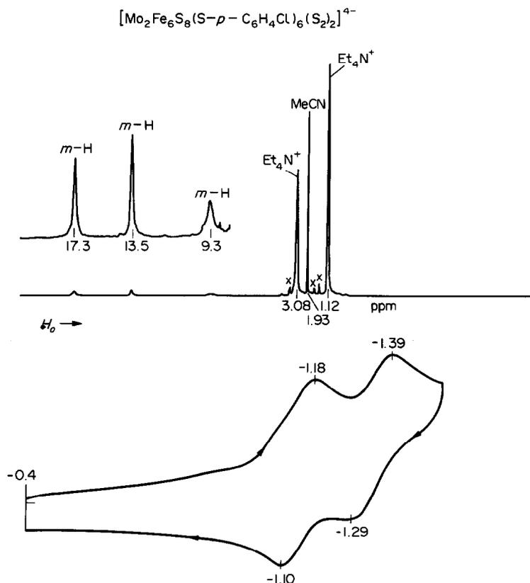
Fig. 4. Upper:  $^1\text{H}$  NMR spectrum (300 MHz) of  $[\text{Mo}_2\text{Fe}_6\text{S}_8(\text{S}_2)_2(\text{S}-p-\text{C}_6\text{H}_4\text{Cl})_6]^{4-}$  (**10**) in  $\text{CD}_3\text{CN}$  solution at 298 K. Lower: cyclic voltammogram of **10** in acetonitrile solution (0.1 M  $n\text{-Bu}_4\text{NCl}$  supporting electrolyte, 100  $\text{mV s}^{-1}$ , glassy carbon working electrode). Peak potentials vs SCE are given.
