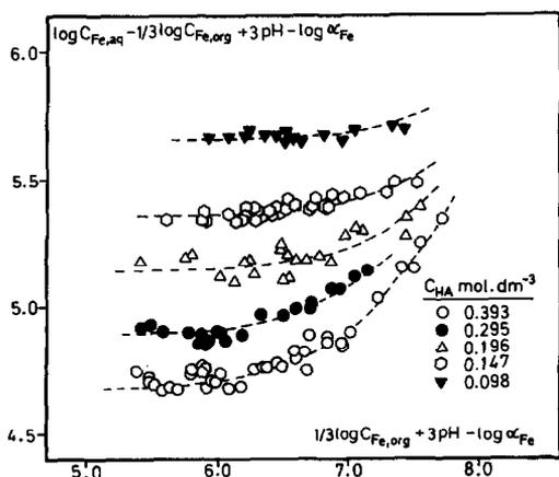
Fig. 5. Positions of best fit between the experimental function  $\log C_{\text{Fe,aq}} - (1/3) \log C_{\text{Fe,org}} + 3\text{pH} - \log \alpha_{\text{Fe}} = f((1/3) \log C_{\text{Fe,org}} + 3\text{pH} - \log \alpha_{\text{Fe}})$  and the theoretical  $\log Y = f(\log X)$ .
