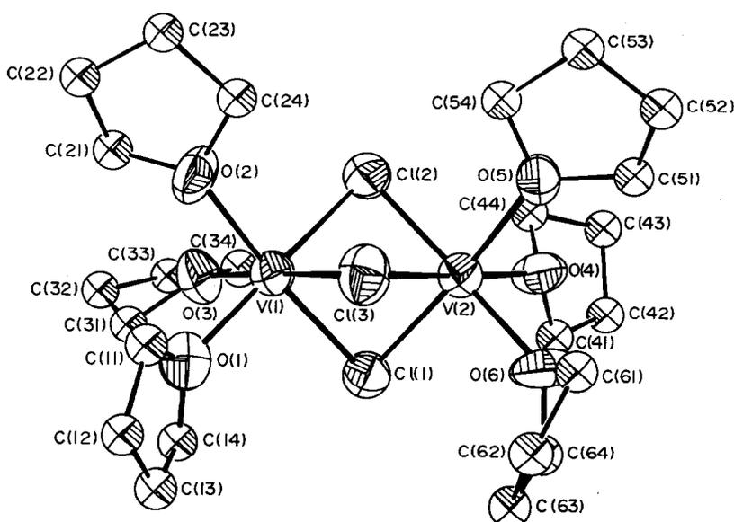
Fig. 1. ORTEP drawing (50% probability level) of the  $[V_2Cl_3(THF)_6]^+$  cation. The carbon atoms have been assigned the same isotropic thermal parameter for the sake of clarity.
