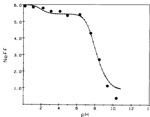
Fig. 14. Dependence of the effective coordination number of water upon pH, for Solution I. The experimental points were calculated from the ratio of the paramagnetic transverse relaxation rate of water in the presence and absence of glycine, respectively, and the dotted line is the theoretical prediction of eqn (14).
