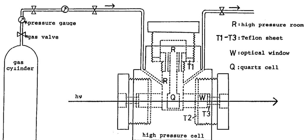
Fig. 1. Schematic diagram of the high-pressure cell system.
