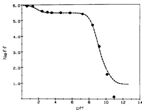
Fig. 15. Dependence of the effective coordination number of water upon pH, for Solution H. The experimental points were calculated from the ratio of the paramagnetic transverse relaxation rate of water in the presence and absence of proline, respectively, and the dotted line is the prediction of eq. (33).
