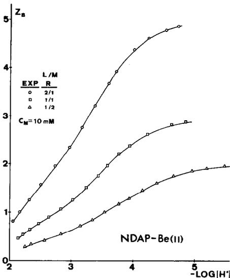
Fig. 2.  $Z_B$  vs  $-\log[H^+]$  curves for the NDAP-Be(II) system. Full curves have been calculated using the  $\beta_{pqr}$  constants in Table 2.
