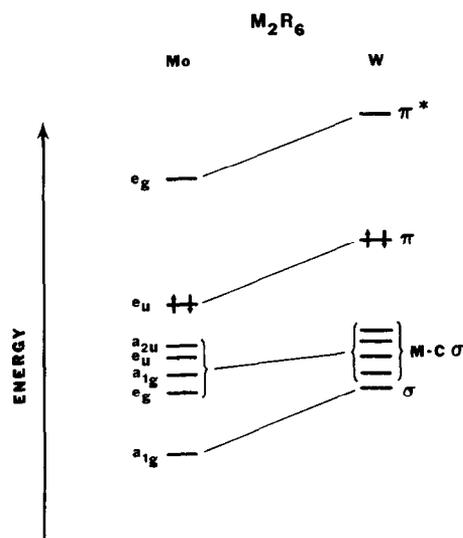
Fig. 5. Qualitative valence energy level diagram describing the differences between  $\text{Mo}_2(\text{R})_6$  and  $\text{W}_2(\text{R})_6$ .
