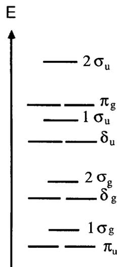
Fig. 2. Orbital-level diagram for  $M_2$ , with orbitals classified according to  $D_{\infty v}$ -symmetry.
