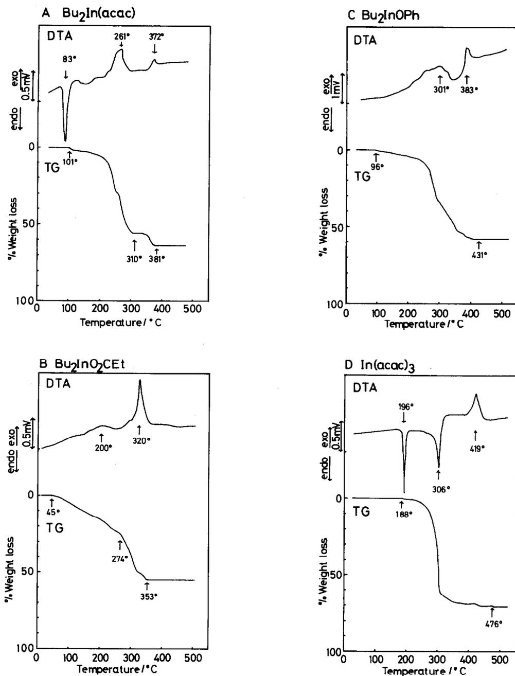
Fig. 1. Thermograms of organoindium compounds: (A)  $Bu_2In(acac)$ , (B)  $Bu_2In(O_2CET)$ , (C)  $Bu_2In(OPh)$ , and (D)  $In(acac)_3$ .
