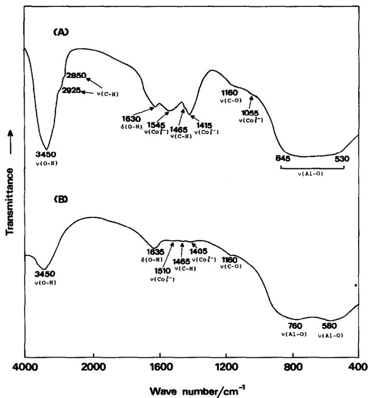
Fig. 2. Infrared spectra for (A) starting powder and (B)  $\gamma$ -Al<sub>2</sub>O<sub>3</sub>.
