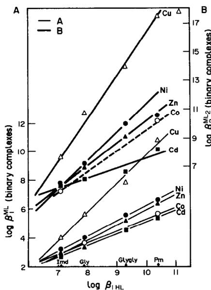
Fig. 1. Dependence of  $\log \beta_1^{ML}$  (scale A) and  $\log \beta_2^{ML_2}$  (scale B) on the basicity of the ligand exemplified by  $\log \beta_{1HL}$  for Co(II), Ni(II), Zn(II) and Cd(II) metal ions.
