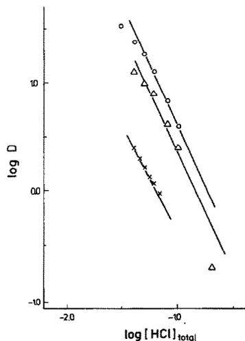
Fig. 6. Acid concentration dependency of the  $D$  of Hg(II) at  $[\text{HL}] > [\text{HCl}]$ ,  $[\text{HD}] = 1.05 \times 10^{-2}$  F. (○) [Im] = 0.25 M; (△) [2MIm] = 0.25 M; (×) [His] = 0.12 M.
