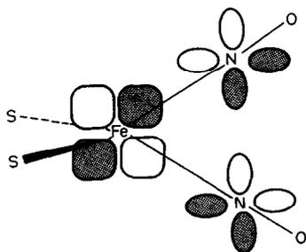
Fig. 2. The SOMO in complexes of types  $[\text{Fe}(\text{NO})_2(\text{SR})_2]^-$  and  $[\text{Fe}(\text{NO})_2(\text{S}_2\text{MoS}_2)]^-$ .
