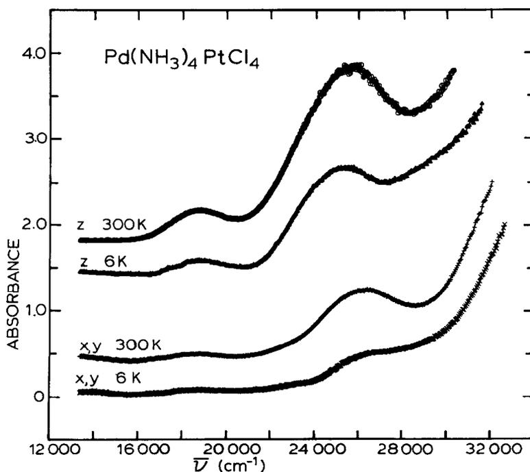
Fig. 6. Polarized spectra for  $\text{Pd}(\text{NH}_3)_4\text{PtCl}_4$  crystal,  $13 \mu\text{m}$  thick.
