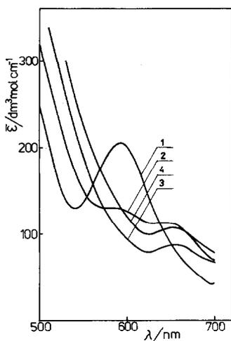
Fig. 7. Absorption spectra of copper(II) for  $\text{CuBr}_2$ -DMF-chlorobenzene solutions at  $25^\circ\text{C}$  for constant  $\text{CuBr}_2$  concentration ( $0.00512 \text{ mol dm}^{-3}$ ) and variable chlorobenzene mole fraction: (1) 0.0, (2) 0.638, (3) 0.862, (4) 0.945.
