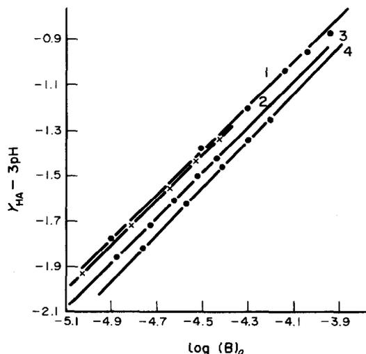
Fig. 5. Synergic extraction of Pr(III) with constant  $C_{HA}$  and various  $C_B$  in different organic solvents: (1) benzene, (2) toluene, (3) xylene, and (4) CCl<sub>4</sub>.  $C_{HA} = 5 \times 10^{-4}$  M,  $Y_{HA} = \log D - 3 \log (HA)_o$ .
