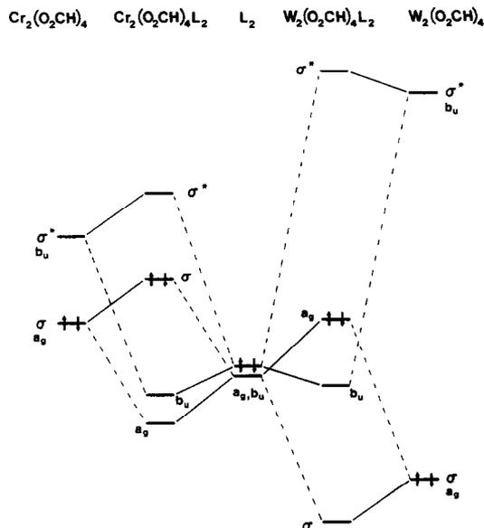
Fig. 4. Qualitative molecular-orbital diagram comparing the interaction of a neutral donor ligand L with  $Cr_2(O_2CH)_4$  and  $W_2(O_2CH)_4$ . Only the  $\sigma$  interactions are depicted for clarity.
