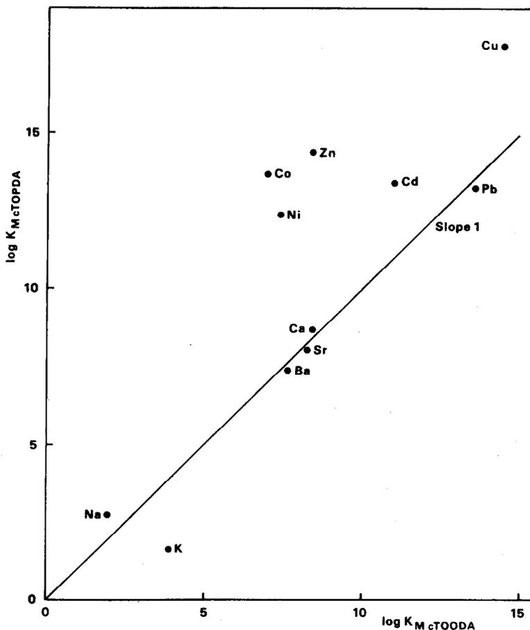
Fig. 3. Correlation of the stability constants ( $\log K_{ML}$ ) of the metal complexes of cTOPDA and cTOODA. A slope 1 straight line would correspond to equal stabilities for the complexes of the two ligands.
