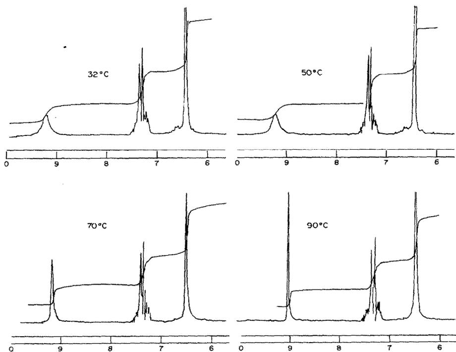
Fig. 3. <sup>1</sup>H-NMR spectra of spiroborate 5 at various temperatures (90 MHz).
