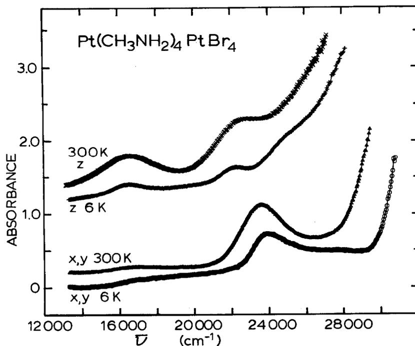
Fig. 9. Polarized spectra for  $\text{Pt}(\text{CH}_3\text{NH}_2)_4\text{PtBr}_4$  crystal,  $4.0 \mu\text{m}$  thick.
