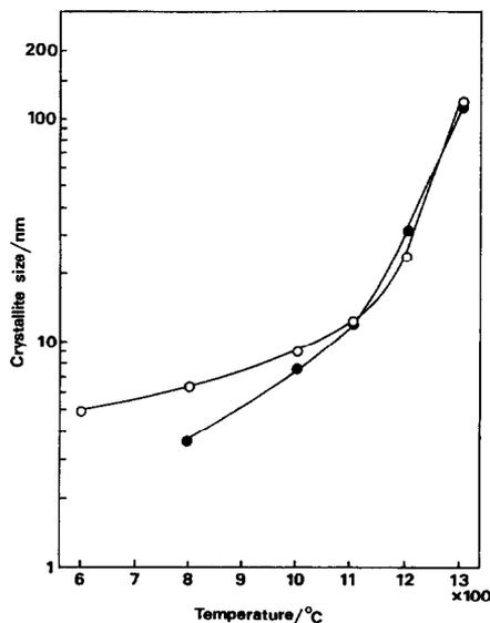
Fig. 5. Crystallite size of  $\text{MgO}$  and  $\text{MgAl}_2\text{O}_4$  in products obtained from starting powder B with increasing temperature. Phases:  $\circ$ ,  $\text{MgO}$ ;  $\bullet$ ,  $\text{MgAl}_2\text{O}_4$ . Heating rate is  $10^\circ\text{C}/\text{min}$ .
