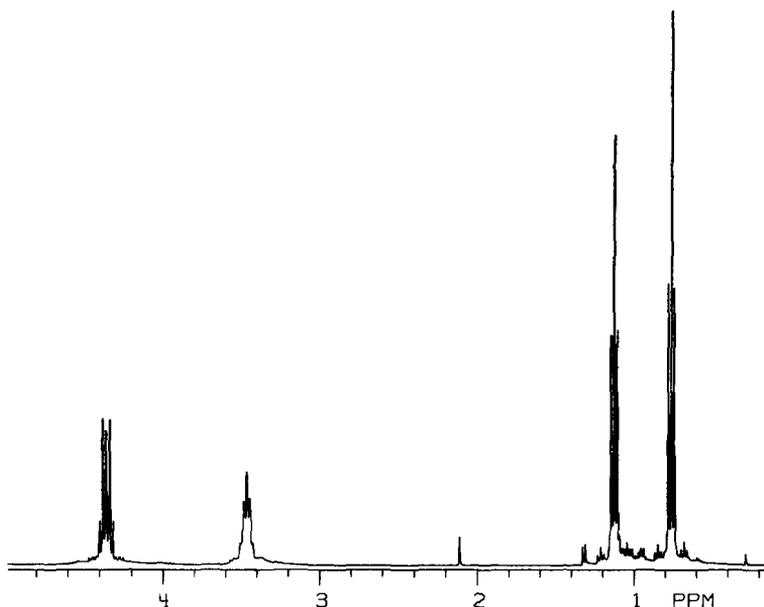
Fig. 1.  $^1\text{H}$  NMR spectrum of  $\text{W}_2\text{S}_2[\text{S}_2\text{P}(\text{OEt})_2]_4$  in benzene- $d_6$  at  $22^\circ\text{C}$  (360 MHz).
