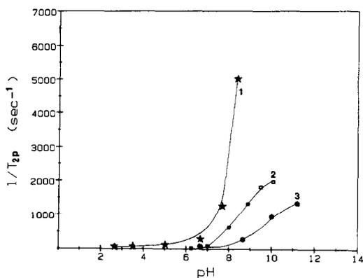
Fig. 7. Dependence of the  $^{14}\text{N}$  paramagnetic transverse relaxation rate of glycine upon pH, for Solutions D (1.0 M glycine and 0.01 M  $\text{CoCl}_2$ ), E (1.0 M glycine and 1.0 mM  $\text{CuCl}_2$ ), and F (1.0 M glycine and 1.0 mM  $\text{MnCl}_2$ ), at 300 K. The spectrometer frequency was 18.075 MHz.
