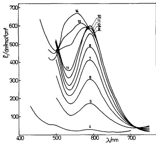
Fig. 2. Absorption spectra of  $\text{Cu}(\text{ClO}_4)_2\text{-Et}_4\text{NBr}^-$  solutions in DMF at  $25^\circ\text{C}$ . The concentrations ( $\text{mol dm}^{-3}$ ) of  $\text{Cu}(\text{ClO}_4)_2$  and  $\text{Et}_4\text{NBr}$  are, respectively: (4) 0.00556, 0.00729; (5) 0.00512, 0.00970; (6) 0.00913, 0.01213; (7) 0.00511, 0.01448; (8) 0.00518, 0.01675; (9) 0.00536, 0.02207; (10) 0.00534, 0.03218; (11) 0.00545, 0.05349; (12) 0.00540, 0.10837; (13) 0.00500, 0.13319; (14) 0.00511, 0.17235.
