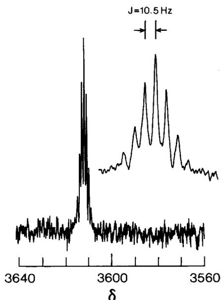
Fig. 1.  $^{183}\text{W}$  NMR spectrum of  $\text{W}(\text{CSiMe}_3)(\text{CH}_2\text{SiMe}_3)_3$  in  $d^6$ -benzene. The insert shows an expansion of the septet resonance. Acquisition parameters were: spectral width, 5 kHz; acquisition time, 1.638 s; digital resolution, 0.61 Hz (point) $^{-1}$ ; number of scans, 17,400.
