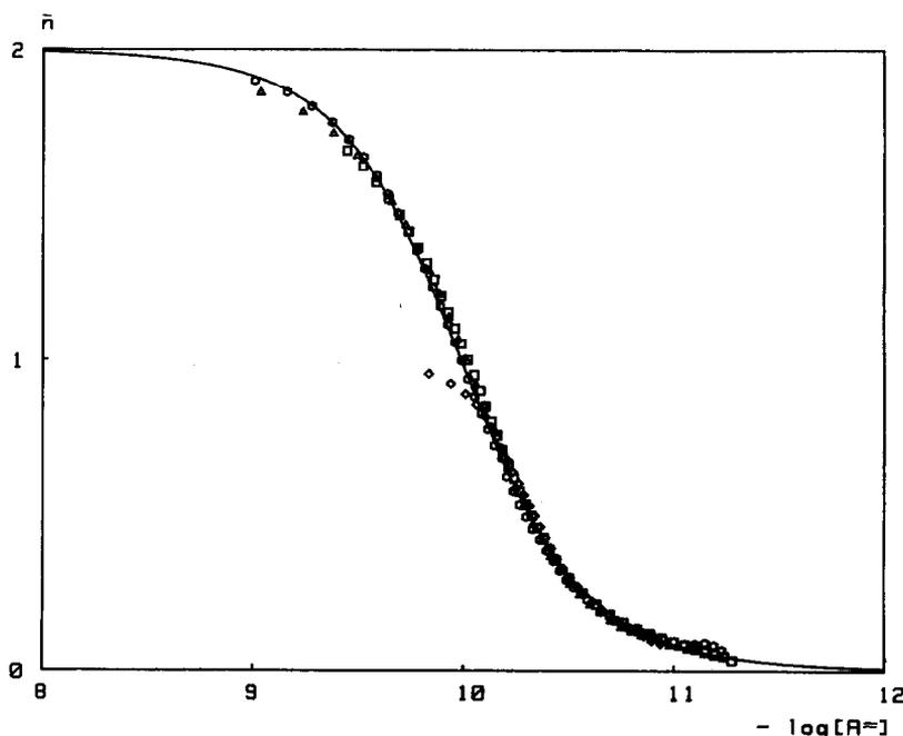
Fig. 1. Experimental formation curves for the Ni(II)–NMPA system. Symbols are: (○) titr. 4, (□) titr. 5, (△) titr. 6 and (◇) titr. 7. Solid line is the theoretical curve after the constants given in Table 2.
