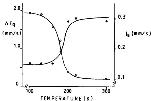
Fig. 5. Variation of quadrupole splitting ( $\Delta E_q$ ) (open circles) and isomer shift ( $I_s$ ) (closed circles) with temperature in the range 100–300 K.
