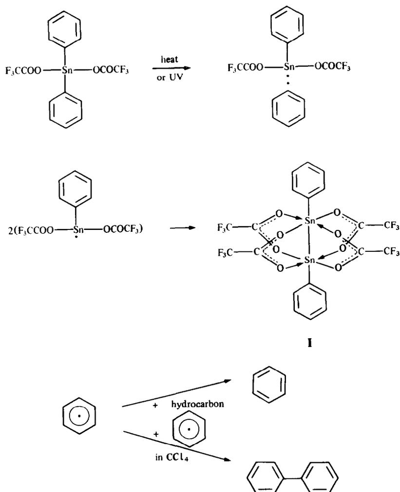
Fig. 1. Behaviour of  $\text{Ph}_2\text{Sn}(\text{OCOCF}_3)_2$  when heated in non-polar media and UV light.
