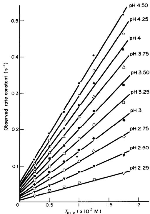
Fig. 3.  $k_{\text{obs}}(\text{PLP})$  as function of  $T_{\text{PLP}}$  at interpolated pH values.
