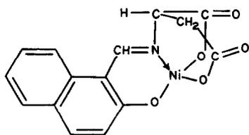
Fig. 3. Ni(II)-naphthylideneaspartic acid complex (square planar structure).
