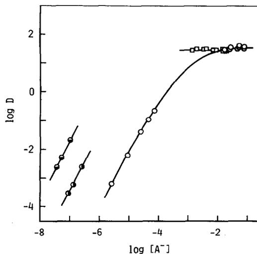
Fig. 1. Distribution ratio of nickel(II) vs concentration of chelating anion in the aqueous phase. Initial concentration of Htta: 0.08–0.11 M; pH 2.0–8.2. Initial concentration of Nadmdtc: 0.002–0.020 M; pH 6.0–8.5.  $\circ$  Htta–benzene;  $\bullet$  Htta–isobutylmethyl ketone;  $\bullet$  Htta–diisobutyl ketone;  $\square$  Nadmdtc–heptane.
