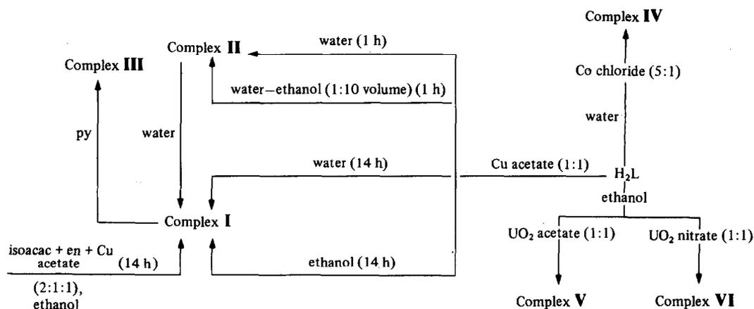
Fig. 1. Schematic representation for the reactions of the ligand with the metal ions and the reactivity of some of the Cu(II) complexes (isoacac, en, py and pip refer to isonitrosoacetylacetone, ethylenediamine, pyridine and piperidine, respectively).
