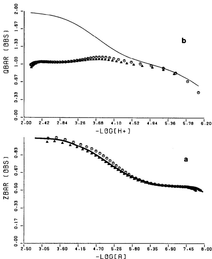
Fig. 2. (a) Experimental formation curves of  $\bar{Z}$  vs  $-\log$  (free ligand) for the aluminium(III) ATP system at 25°C and 0.15 mol dm<sup>-3</sup> (Na)[Cl]. The full line represents the theoretical curve obtained using the formation constants given in Table 1. (b) Experimental deprotonation curves of  $\bar{Q}$  vs pH. The full line represents the  $\bar{n}$  function. For clarity only selected points have been plotted.
