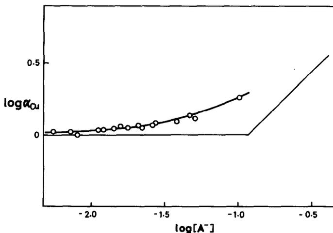
Fig. 2. Determination of the formation constant of copper(II)  $\alpha$ -bromovalerate complex in the aqueous solution. Ionic strength: 1.0 (Na,H)ClO<sub>4</sub>.  $\alpha_{\text{Cu}}$  was obtained from e.m.f. measurement by using a cupric ion selective electrode. The solid curve denotes the theoretical one calculated by using  $\log K_{\text{CuA}} = 1.50$ . The straight lines are the asymptotes for the curve.
