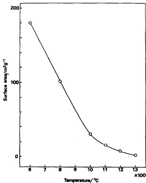
Fig. 6. Surface area of products obtained from starting powder B with increasing temperature. Heating rate is 10°C/min.
