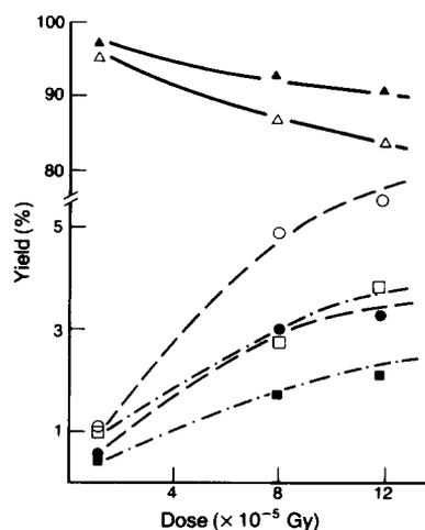
Fig. 1. Yields of GeH<sub>3</sub>T, HT and Ge<sub>2</sub>H<sub>5</sub>T at 6.7 kPa (light points) and at  $1.6 \times 10^2$  kPa (black points) as function of the absorbed dose: (—) GeH<sub>3</sub>T, (---) HT, and (-·-) Ge<sub>2</sub>H<sub>5</sub>T.
