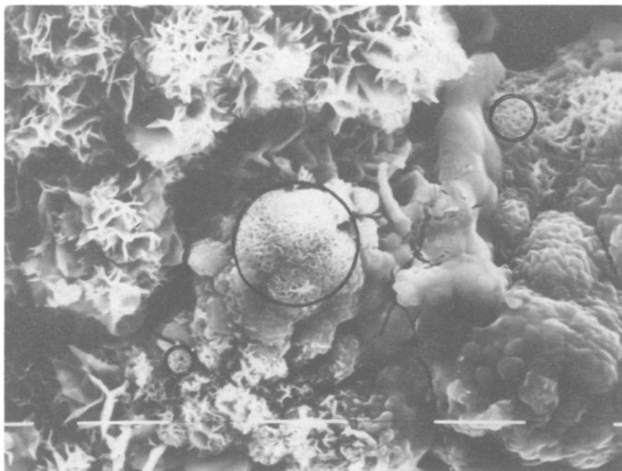
Fig. 2. SEM picture ( $1700\times$ ) of the pyrolysis ( $700^\circ\text{C}$ ) product of  $\text{Co}_3[\text{Fe(CN)}_5\text{nide}]_2 \cdot 9\text{H}_2\text{O}$ . Circles indicate Co-rich regions according to EDAX; other regions are Fe-rich.
