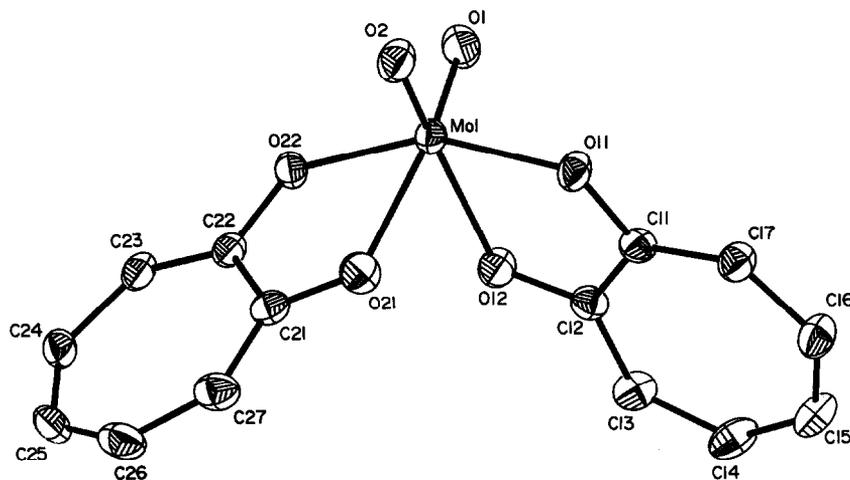
Fig. 1. Molecular structure of  $\text{MoO}_2(\text{trop})_2$ . Thermal vibration ellipsoids are scaled to enclose 50% probability.
