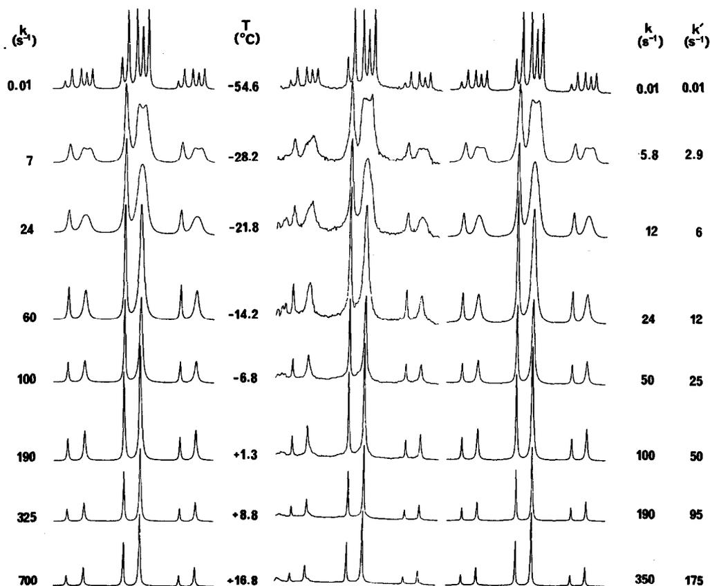
Fig. 5. Experimental and computer synthesised variable temperature  $^1H$  NMR spectra of  $[PtMe_3(MeSCH_2CH_2)_2S]^+I^-$  in the Pt—Me region.
