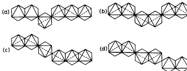
Fig. 2. Inorganic polymers containing both edge and corner sharings produced by "scissoring" of I. There is one path in (b) and (c), but no path in (a) and (d).
