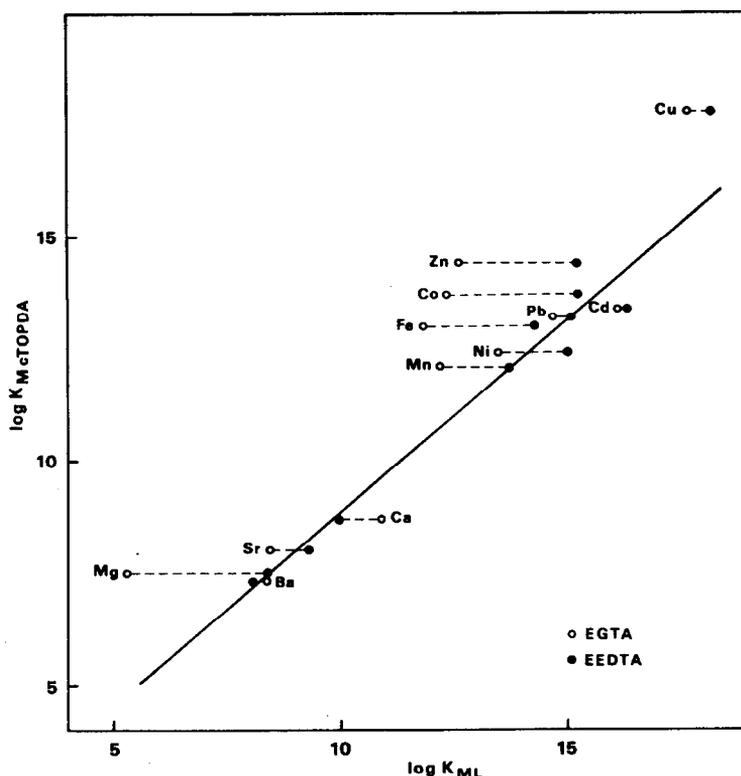
Fig. 4. Correlation of the stability constants ( $\log K_{ML}$ ) of the complexes of cTOPDA and EEDTA (●), showing the shifts when EGTA (○) is considered instead of the latter ligand.
