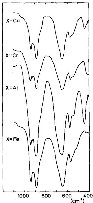
Fig. 1. Solid IR spectra of Anderson-type  $[\text{X}(\text{III})\text{Mo}_6\text{O}_{24}\text{H}_6]^{3-}$  polyanions.
