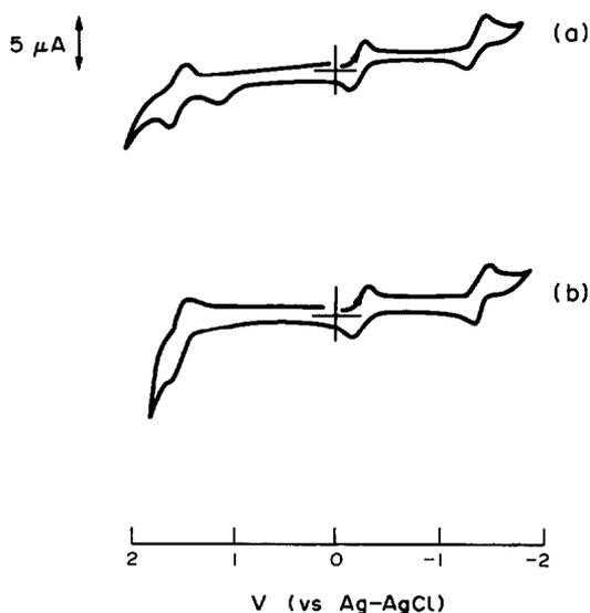
Fig. 1. Cyclic voltammograms (recorded at  $\nu = 200\text{ mV s}^{-1}$  using a Pt-bead electrode) for 0.1 M TBAH- $\text{CH}_2\text{Cl}_2$  solutions of: (a)  $[\text{ReCl}_2(\text{dppee})_2]\text{Cl} \cdot 4\text{H}_2\text{O}$ , and (b)  $[\text{ReCl}_2(\text{dppee})_2]\text{ClO}_4$ .
