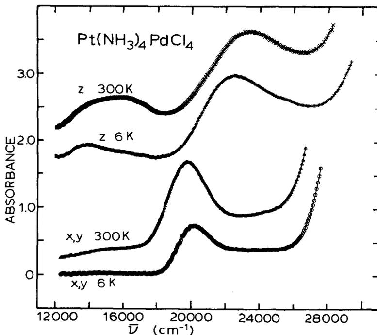
Fig. 13. Polarized spectra for  $\text{Pt}(\text{NH}_3)_4\text{PdCl}_4$  crystal,  $9 \mu\text{m}$  thick.
