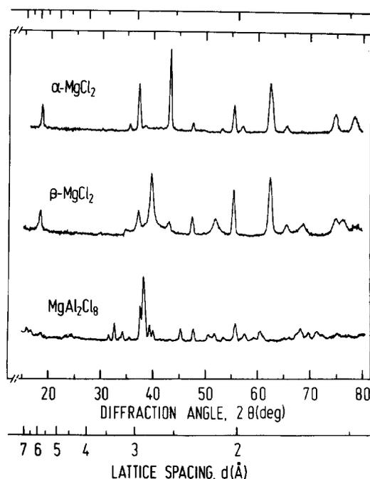
Fig. 2. Neutron powder diffraction patterns of the two crystal modifications of  $\text{MgCl}_2$  and  $\text{MgAl}_2\text{Cl}_8$ .
