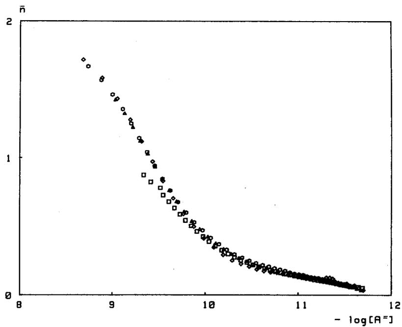
Fig. 2. Experimental formation curves for the Zn(II)-NMPA-H system. Symbols: ( $\diamond$ ) titr. 8, ( $\circ$ ) titr. 9, ( $\triangle$ ) titr. 10 and ( $\square$ ) titr. 11.
