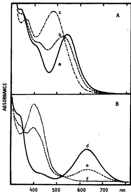
Fig. 5. Spectroelectrochemistry of the ruthenium(III)/(II)-(edta) complexes of 2-mercaptopyridine at (A) pH 2.8, and (B) pH 9.2,  $I = 0.10$  M Lipts. Applied potentials. (a) 0.22, (b) 0.32, (c) 0.42, (d) 0.12, (e)  $-0.13$  and (f)  $-0.28$  V versus NHE.
