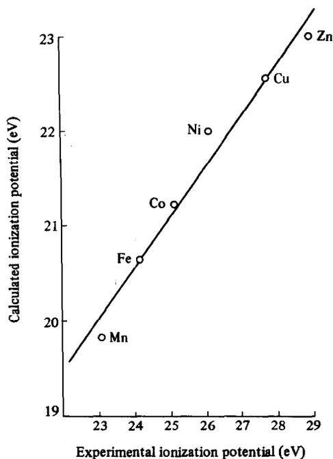
Fig. 1. Plot of calculated vs experimental ionization potentials of transition elements ( $M \rightarrow M^{2+}$ ).
