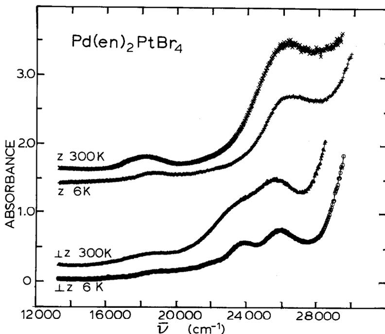
Fig. 12. Polarized spectra for  $\text{Pd}(\text{en})_2\text{PtBr}_4$  crystal, 8  $\mu\text{m}$  thick.
