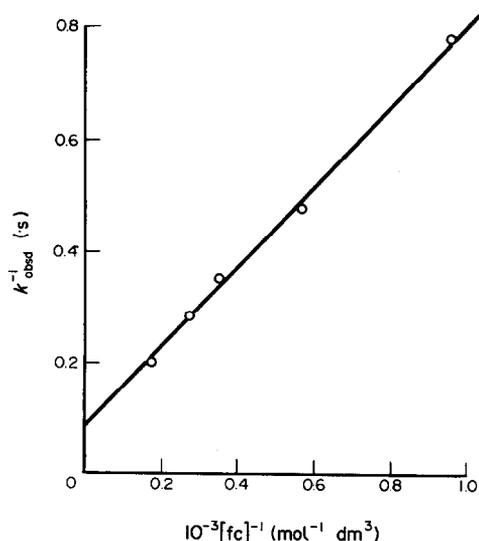
Fig. 2. Plot of  $k_{\text{obsd}}^{-1}$  against  $[\text{fc}]^{-1}$  for the reaction of complex 1 with fc in acetonitrile at 25°C.
