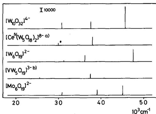
Fig. 3. Bar graphs of absorption maxima of a polyanion-group containing 'M<sub>5</sub>O<sub>18</sub>' (M = W and Mo) fragment. Height shows relative intensity and abscissa shows wavenumber. The data of (a) and (b) are reported in Refs 14 and 15, respectively. Asterisked peak indicates a CT band of ligand-to-Ce(IV).
