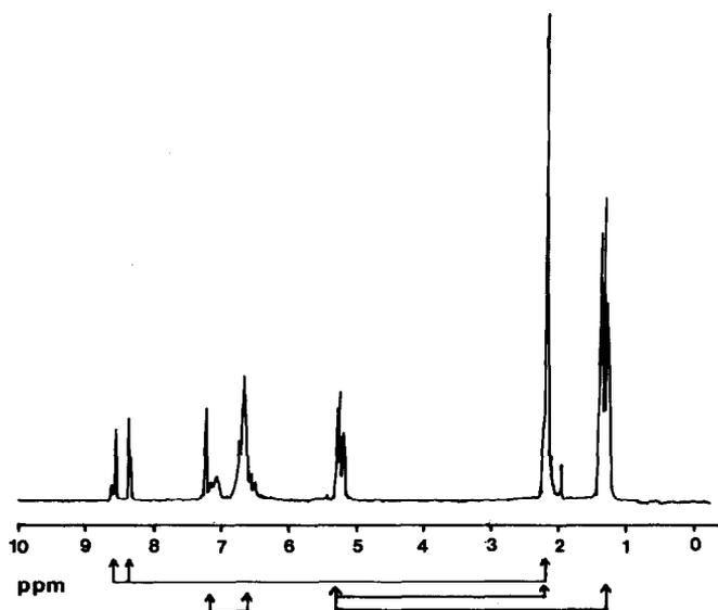
Fig. 1.  $^1\text{H}$ -NMR spectrum of a freshly prepared sample of **I** in  $\text{CDCl}_3$ ; the connectivities indicated at the bottom are NOE interactions as measured with a mixing time of 1.4 s.
