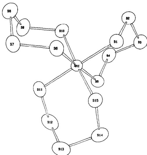
Fig. 1. Ortep drawing of  $\text{Rh}(\text{S}_5)_3^{3-}$  anion showing the labelling scheme.
