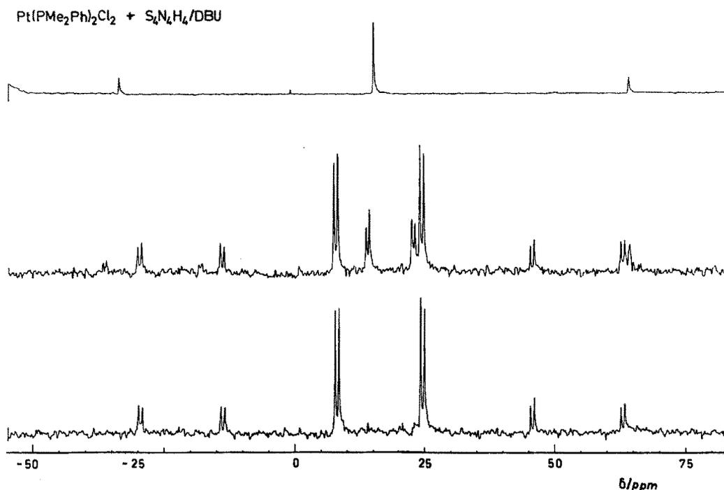
Fig. 1.  $^{31}P\{-^1H\}$  NMR of the reaction of *cis*- $PtCl_2(PMe_2Ph)_2$  with  $S_4N_4H_4$  and dbu. Upper trace shows starting material, middle trace shows  $Pt(S_2N_2)(PMe_2Ph)_2$  and intermediate believed to be *cis*- $PtCl(dbu)(PMe_2Ph)_2$ , lower trace is after addition of additional dbu.
