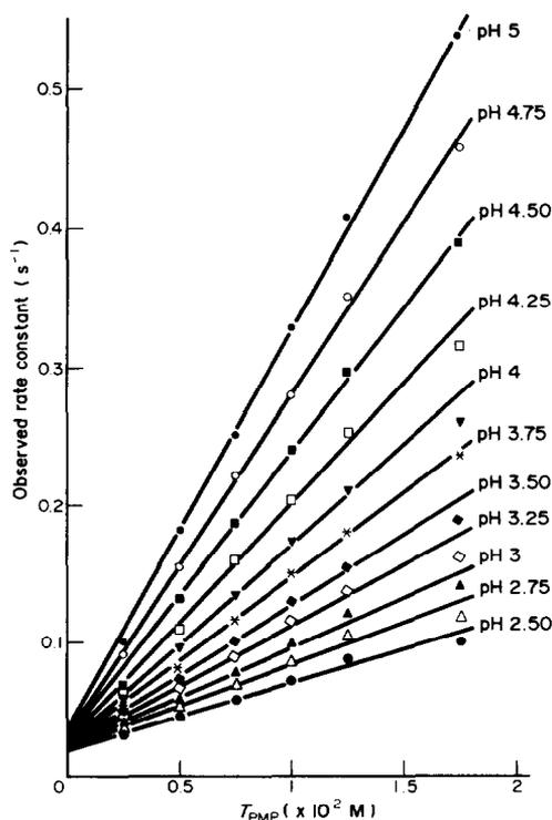
Fig. 7.  $k_{obs}(PMP)$  as function of  $T_{PMP}$  at interpolated pH values.
