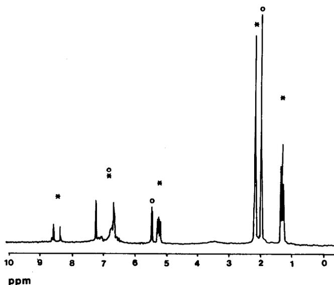
Fig. 3.  $^1\text{H}$ -NMR spectrum of a sample of I in  $\text{CDCl}_3$  after 2 h storing at room temperature; the resonances indicated with \* correspond to dimer and with O to monomer.
