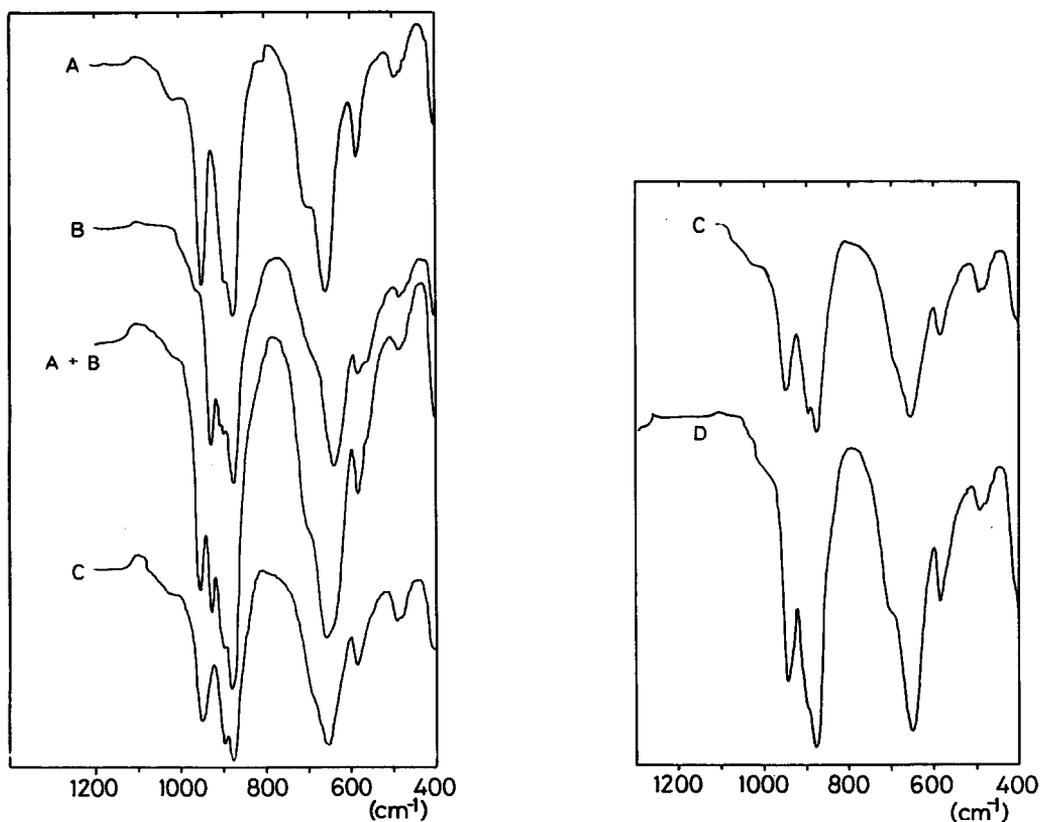
Fig. 4. Solid IR spectra of  $[\text{Ni(II)Mo}_{6-x}\text{W}_x\text{O}_{24}\text{H}_6]^{4-}$  polyanions;  $x = 6$  (A) and  $0$  (B) compounds, equimolar mixture (A + B) of them, and  $x = 3$  compounds obtained by methods 1 (C) and 2 (D).
