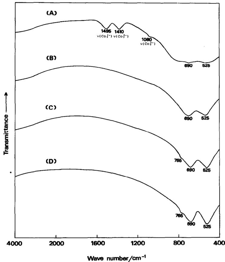
Fig. 5. Infrared spectral patterns for specimens heated at (A) 700, (B) 1000, (C) 1100 and (D) 1250°C.
