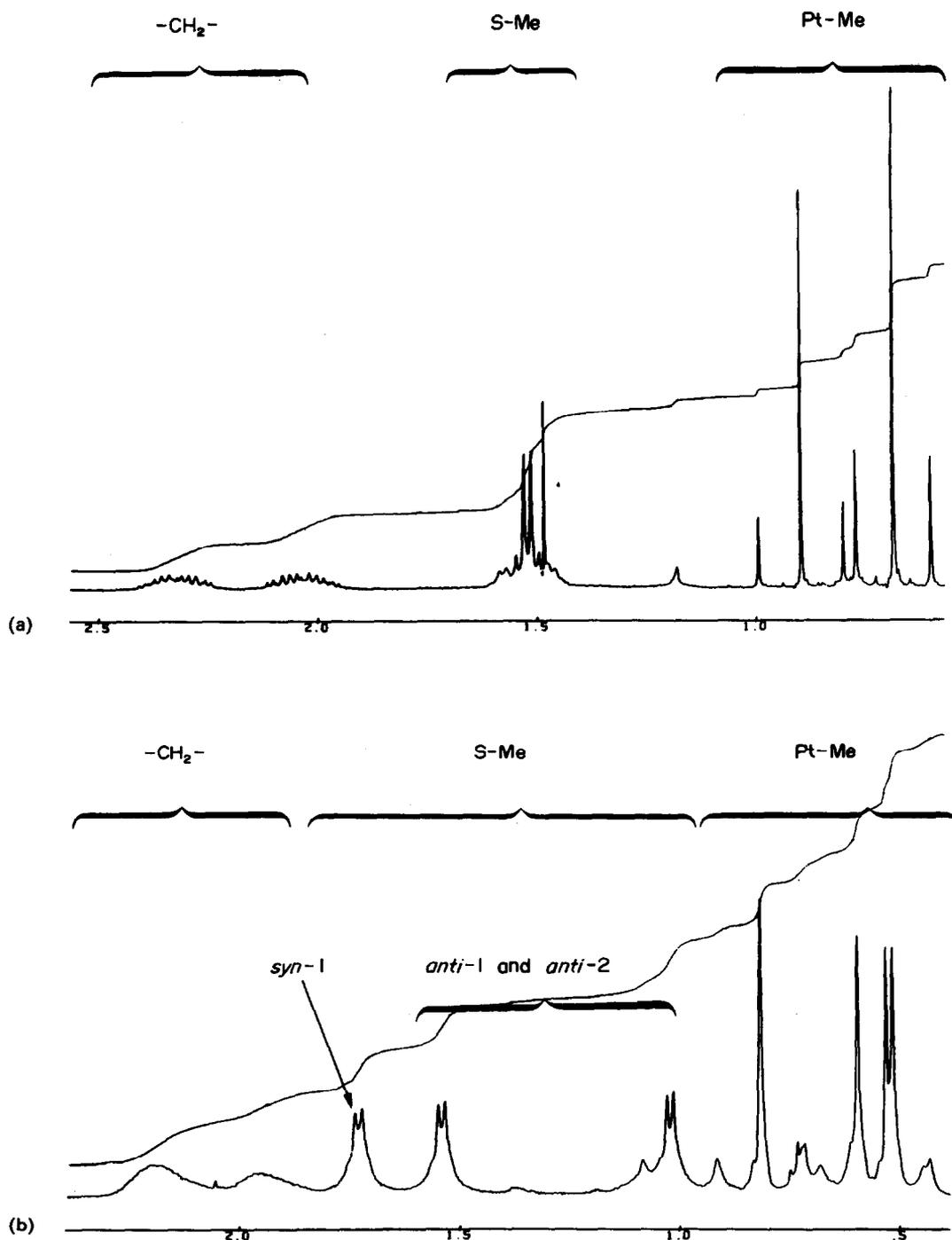
Fig. 2.  $^1\text{H}$  NMR spectra of  $[\text{Pt}(\text{dppe})(\mu_2\text{-SMe})_2\text{PtClMe}_3]$  at: (a)  $25^\circ\text{C}$ , and (b)  $-105^\circ\text{C}$ .
