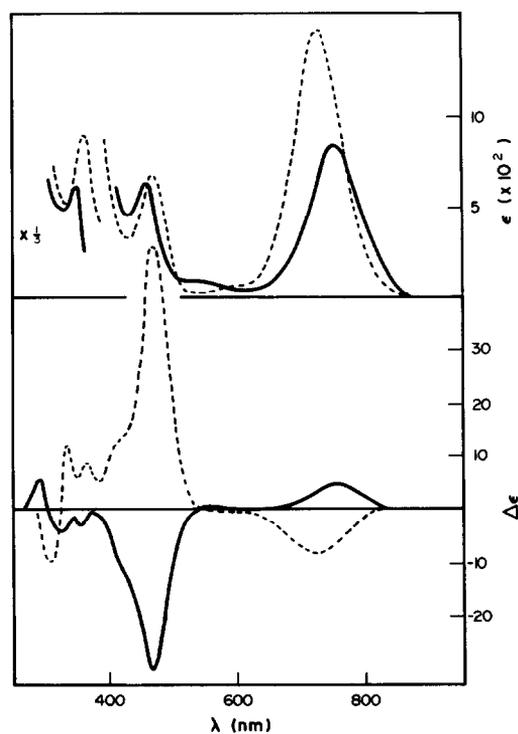
Fig. 9. Absorption and CD spectra of  $\Delta$ -[Mo<sub>2</sub>Cl<sub>4</sub>(R-dppp)<sub>2</sub>] (full line) and  $\Lambda$ -[Mo<sub>2</sub>Cl<sub>4</sub>(S,S-dppb)<sub>2</sub>] (dashed line), both in dichloromethane solution.
