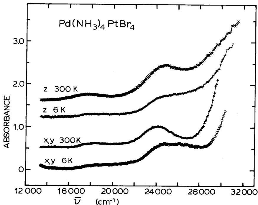
Fig. 11. Polarized spectra for  $\text{Pd}(\text{NH}_3)_4\text{PtBr}_4$  crystal, 6  $\mu\text{m}$  thick.
