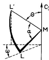
Fig. 2. Definition of bite ( $\alpha$ ), twist ( $\omega$ ) and tilt ( $\theta$ ) angles in an octahedral trigonal tris(bidentate) structure.
