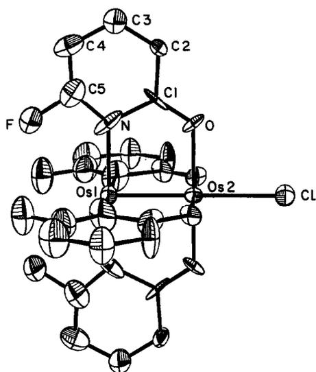
Fig. 2. ORTEP drawing of the Os<sub>2</sub>(fhp)<sub>4</sub>Cl molecule with the atom-labelling scheme. Atoms are represented by their thermal vibration ellipsoids at the 50% level.
