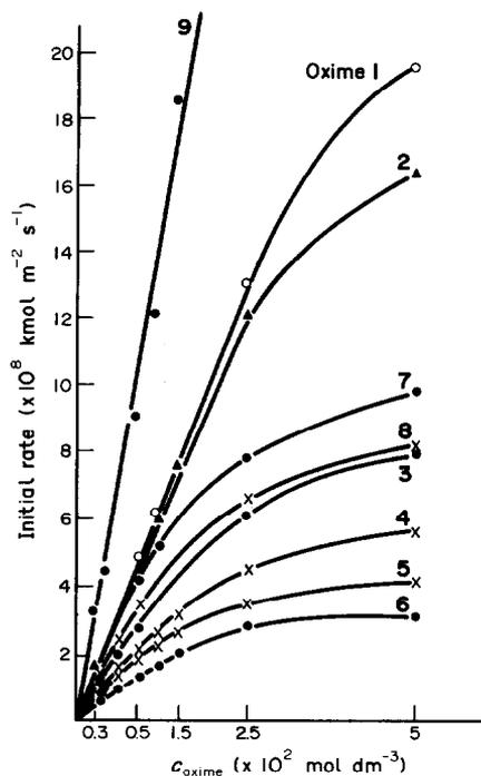
Fig. 3. Influence of the structure of the oxime upon the initial extraction rate (xylene).
