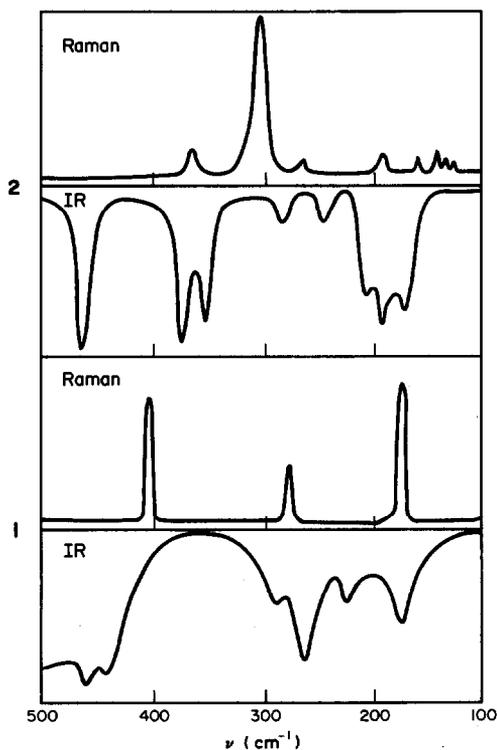
Fig. 1. Vibrational spectra of thiodiacetic acid ( $\text{H}_2\text{L}$ ) (1) and of the complex  $[(\text{H}_2\text{L})_2\text{PdCl}_2]$  (2).
