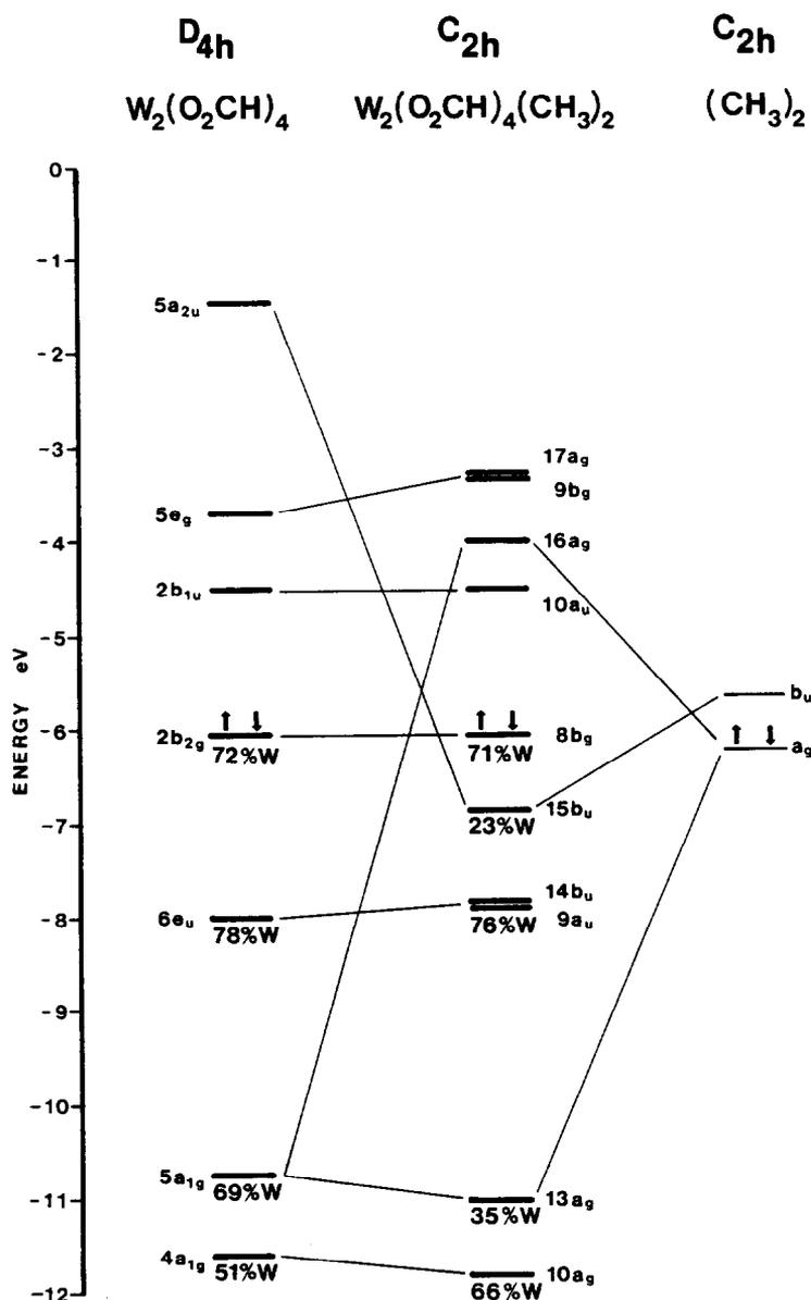
Fig. 5. Results of relativistic SCF-X $\alpha$ -SW calculations on  $W_2(O_2CH)_4(CH_3)_2$ . This diagram shows the correlation of the orbitals of  $W_2(O_2CH)_4(CH_3)_2$  to those of  $W_2(O_2CH)_4$  and  $(CH_3)_2$ . Only those levels involved in W-W bonding or antibonding are shown. The highest occupied orbitals are depicted with arrows. Adapted from Ref. 10.
