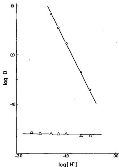
Fig. 1. Acid concentration dependency of  $D$  at  $[\text{HD}] = 1.05 \times 10^{-2}$  F. (O) Zn(II), ( $\Delta$ ) Hg(II).
