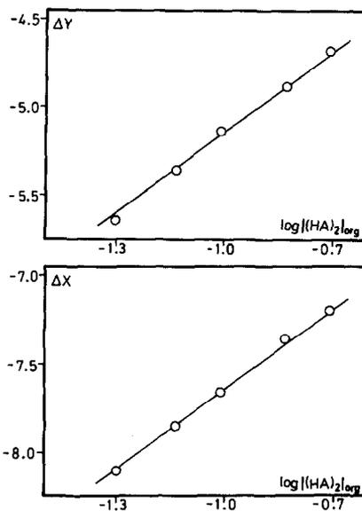
Fig. 6. Plots of the differences  $\Delta Y$  and  $\Delta X$  as a function of free  $n$ -dodecanoic acid concentration.
