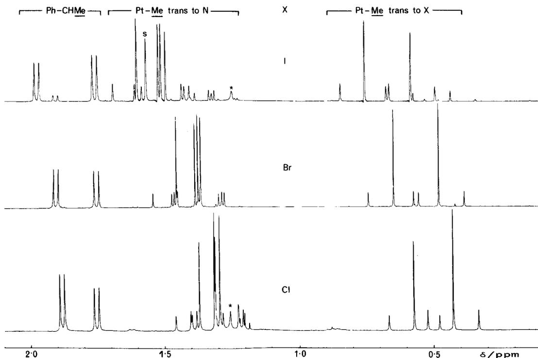
Fig. 2. 400-MHz  $^1\text{H}$  NMR spectra of complexes IA-C in the region 0–2.0 ppm showing the Pt—Me (right) and Ph—CMe signals and the isomer populations (S = solvent, \* = impurity).
