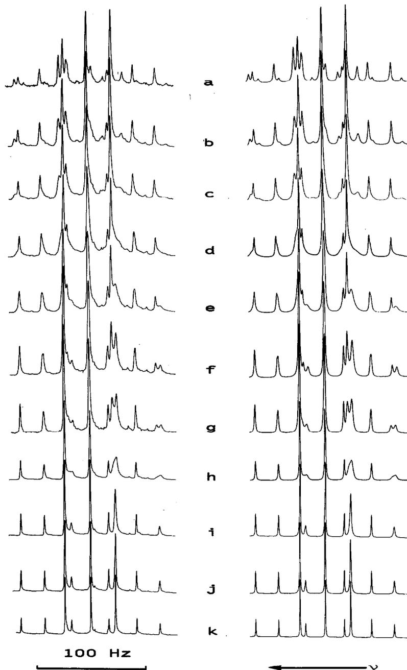
Fig. 9. Experimental and computer synthesised variable temperature  $^1\text{H}$  NMR spectra of  $[\text{PtMe}_3(\text{MeSCH}_2\text{CH}_2\text{S})_2]^+\text{BF}_4^-$  showing the effects of sulphur inversion of the Pt—Me signals.
