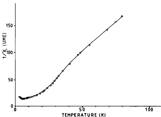
Fig. 3. Reciprocal magnetic susceptibility ( $1/\chi$ ) for  $[\text{Fe}(\text{salophen})\text{NO}]$  in the temperature range 2–80 K.
