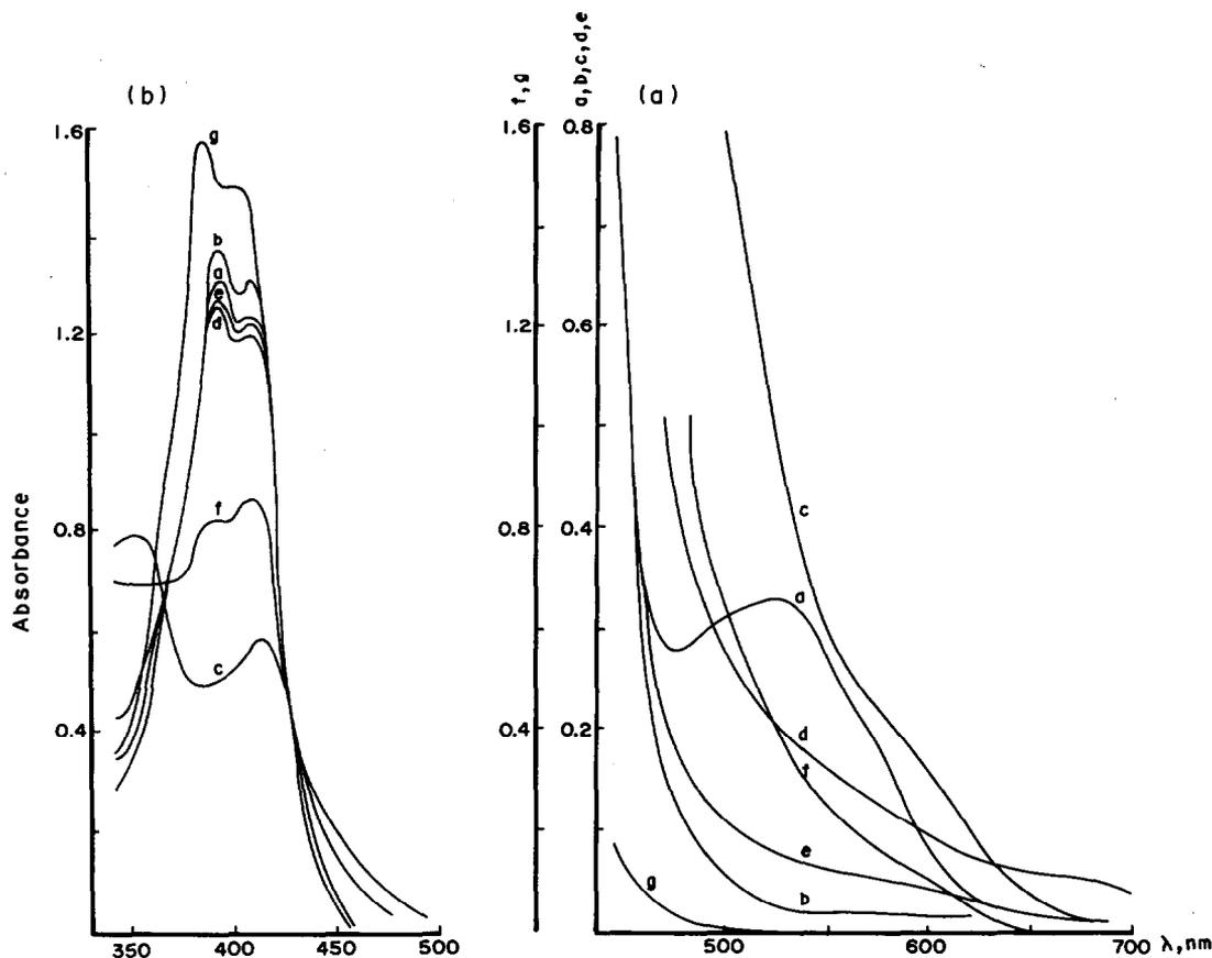
Fig. 1. Visible electronic absorption spectra of  $2 \times 10^{-3}$  M (700–500 nm) (a) and  $1 \times 10^{-4}$  M (500–340 nm) (b) Ni(II)-*N*-naphthylideneamino acid complexes in DMF: (a) gly, (b) ala, (c) val, (d) leu, (e) isoleu, (f) norleu, and (g) ser.
