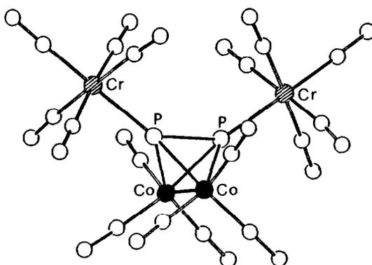
Fig. 8. Structure of the tetranuclear complex  $[[\text{Co}(\text{CO})_3]_2(\mu, \eta^2\text{-P}_2)]\{\text{Cr}(\text{CO})_5\}_2$ .Table 3. Bond distances in the tetrahedrane clusters containing the  $\text{P}_2$  unit<sup>a</sup>
