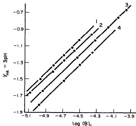
Fig. 6. Synergic extraction of Nd(III) with constant  $C_{HA}$  and various  $C_B$  in different organic solvents: (1) xylene, (2) toluene, (3) benzene, and (4) CCl<sub>4</sub>.  $C_{HA} = 5 \times 10^{-4}$  M,  $Y_{HA} = \log D - 3 \log (HA)_o$ .
