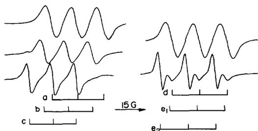
Fig. 2. ESR spectra in chloroform at 240 K of: (a)  $\text{Fe}(\text{NO})(\text{tox})_2$ , (b)  $\text{Fe}(\text{NO})(\text{tox})(\text{Et-xant})$ , (c)  $\text{Fe}(\text{NO})(\text{Et-xant})_2$ , (d)  $\text{Fe}(\text{NO})(\text{tox})_2$ , (e<sub>1</sub>)  $\text{Fe}(\text{NO})(\text{tox})(\text{Et}_2\text{dtc})$ , and (e<sub>2</sub>)  $\text{Fe}(\text{NO})(\text{Et}_2\text{dtc})_2$ .
