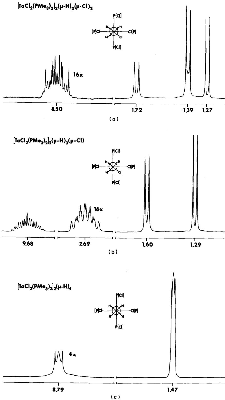
Fig. 3. 360-MHz  $^1\text{H}$  NMR spectra of: (a)  $\text{Ta}_2\text{Cl}_6(\text{PMe}_3)_4\text{H}_2$ , (b)  $\text{Ta}_2\text{Cl}_5(\text{PMe}_3)_4\text{H}_3$ , and (c)  $\text{Ta}_2\text{Cl}_4(\text{PMe}_3)_4\text{H}_4$ .
