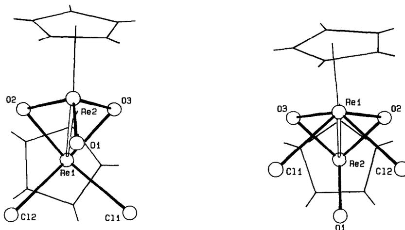
Fig. 3. Schematic drawings of compound 5's molecular structure. *Right*: Projection view onto the  $C_5Me_5$  ring of the  $(C_5Me_5)ReO_3$  core. *Left*: Projection view onto the  $C_5Me_5$  ring of the  $(C_5Me_5)ReO_2Cl_2$  core; this picture shows out-of-centroid distortion of the  $\pi$ -bonding between the metal atom and the five-membered ring ligand.
