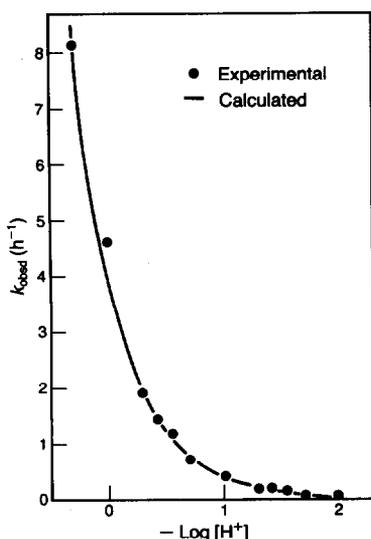
Fig. 3. Hydrolysis rate constants of cyclo-triphosphate at various acid strengths at 40°C.
