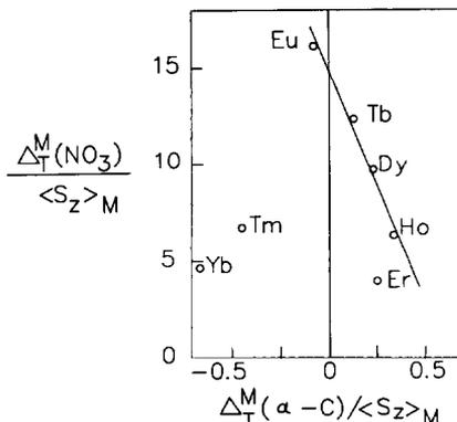
Fig. 3. A plot of  $\Delta_T^M(\text{NO}_3)/\langle S_z \rangle_M$  vs  $\Delta_T^M(\alpha\text{-C})/\langle S_z \rangle_M$  for the  $\text{Ln}(\text{NO}_3)_3^-$  complexes.  $\Delta_T^M(\text{NO}_3)$  is the observed solution isotropic <sup>14</sup>N NMR shift at coordinated nitrate,  $\Delta_T^M(\alpha\text{-C})$  is the solution <sup>13</sup>C isotropic shift at the cation  $\alpha$ -carbon, and  $\langle S_z \rangle_M$  is the effective spin magnetisation. The data are taken from Table 2.
