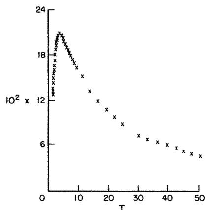
Fig. 4. Plot of the magnetic susceptibility of  $Co_2(OH_2)(CCl_3CO_2)_4(tmen)_2$  as a function of temperature.
