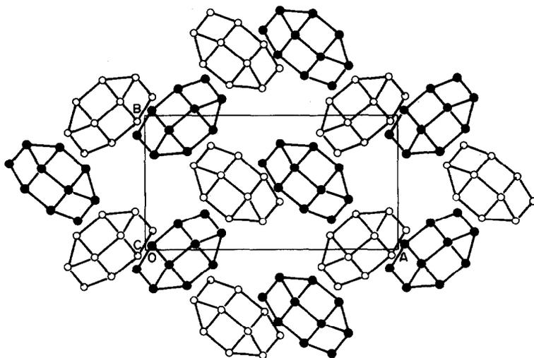
Fig. 4. Packing of anions (represented by their heavy-atom frameworks) in **II**. Filled and open circles denote anions lying on mirror planes at  $z = \frac{1}{4}$  and  $z = \frac{3}{4}$ , respectively. The view is down the  $c$ -axis.
