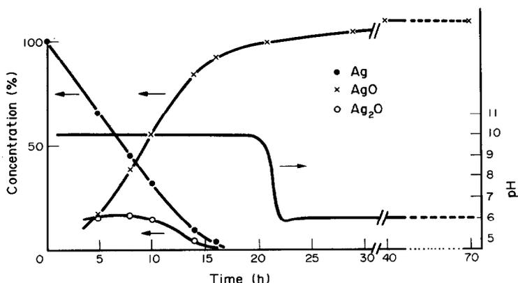
Fig. 1. Evolution of the concentrations and pH during the synthesis. Total flow ( $O_2 + O_3$ ),  $150 \text{ l h}^{-1}$ ; flow of  $O_3$ ,  $2.6 \text{ g h}^{-1}$ ; temperature,  $20^\circ\text{C}$ ; reaction mixture, 100 g of Ag in 10 l of water.
