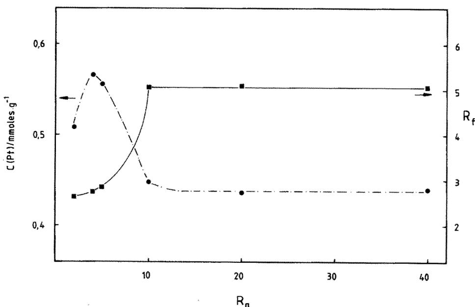
Fig. 2. Variation of the maximum sorptive capacity  $[C(\text{Pt})]$  of polyurethane foam [prepared from polypropylene oxide (MW 3400) and an 80:20 (v/v) mixture of 2,4- and 2,6-toluene diisocyanate] toward Pt(II) in 1.0 mol dm<sup>-3</sup> HCl at 298 K as a function of the Sn(II) : Pt mole ratio ( $R_a$ ). Also shown is the Sn : Pt mole ratio, as observed on the foam ( $R_f$ ).
