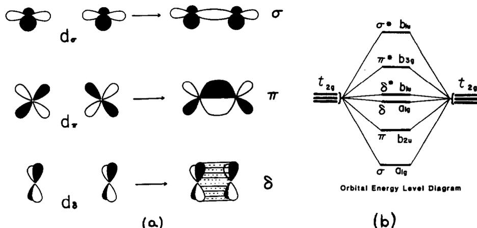
Fig. 3. (a)  $d$ - $d$  overlaps giving rise to M-M bonding orbitals of  $\sigma$ ,  $\pi$  and  $\delta$  types. (b) Pattern of energy levels expected purely on the basis of relative orbital overlaps.
