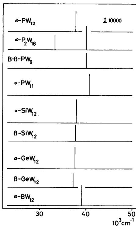
Fig. 6. Bar graphs of absorption maxima of a polyanion-group containing 'XW<sub>9</sub>O<sub>34</sub>' (X = P, Si, Ge, B) fragment. Height shows relative intensity and abscissa shows wavenumber.
