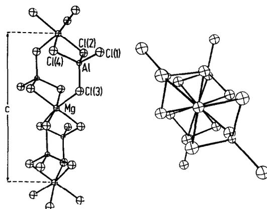
Fig. 5. The repeating part, C, of the infinite chain in  $\text{MgAl}_2\text{Cl}_8$ . The right drawing is turned  $90^\circ$  compared to the left and lacks the three upper and the three lower chlorine atoms for clarity.
