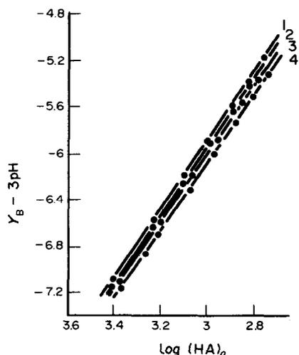
Fig. 3. Synergic extraction of Pr(III) with various  $C_{HA}$  and constant  $C_B$  in different organic solvents: (1) benzene, (2) toluene, (3) xylene, and (4) CCl<sub>4</sub>.  $C_B = 1 \times 10^{-4}$  M,  $Y_B = \log D - \log (B)_o$ .
