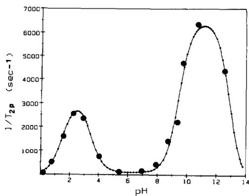
Fig. 9. Dependence of the  $^{17}\text{O}$  paramagnetic transverse relaxation rate of glycine upon the measured pH of a solution containing 0.29 M glycine and 0.2 mM  $\text{CuCl}_2$  (Solution G). The experimental points were recorded at 24.4 MHz, 300 K, and the dotted line is the least-squares best fit of the experimental points to eqn (9), with the constants of Tables 3 and 4.
