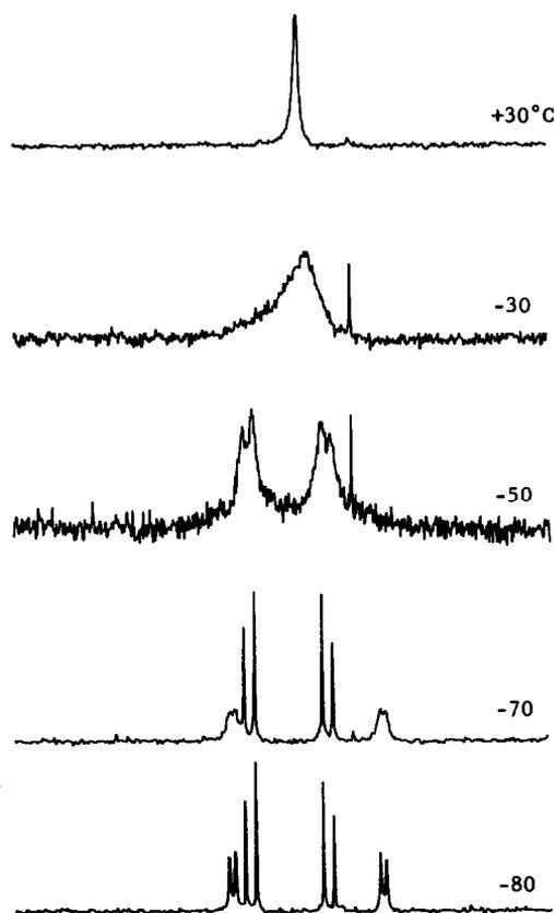
Fig. 4. Variable temperature  $^{31}\text{P}\{-^1\text{H}\}$  NMR spectra of  $\text{Mo}(\text{CO})_3\text{I}_2(\text{Ph}_2\text{PCH}_2\text{PPh}_2)$ .
