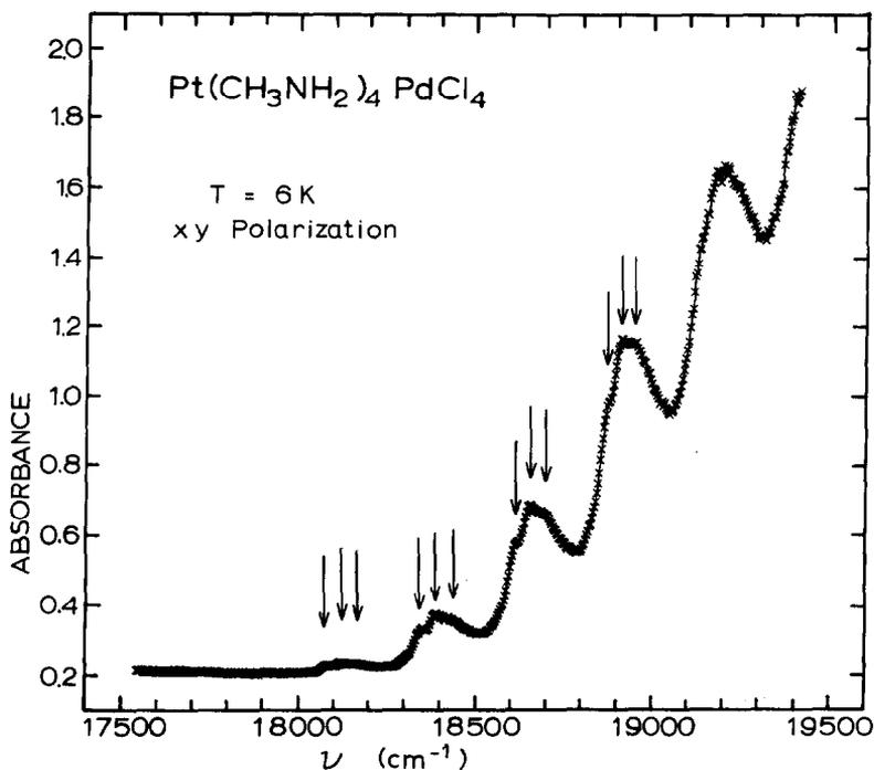
Fig. 15. Spectrum in  $x,y$  polarization at 6 K for  $\text{Pt}(\text{CH}_3\text{NH}_2)_4\text{PdCl}_4$  crystal,  $70\ \mu\text{m}$  thick.
