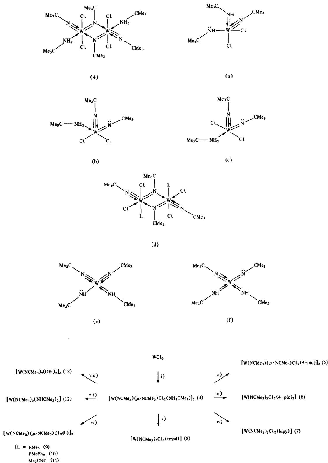
Scheme 1. (i) 4 equivs  $\text{Me}_3\text{SiNHCMe}_3$  or 7 equivs  $\text{Me}_3\text{CNH}_2$ , (ii) 2 equivs 4-picoline, (iii) 4 equivs 4-picoline, (iv) 2 equivs 2,2'-bipyridyl, (v) 2 equivs *N,N,N',N'*-tetramethylethylenediamine, (vi) 2 equivs L, (vii) 4 equivs  $\text{Me}_3\text{CNH}_2$ , (viii) 2 equivs each of EtOH and  $\text{Me}_3\text{CNH}_2$ .
