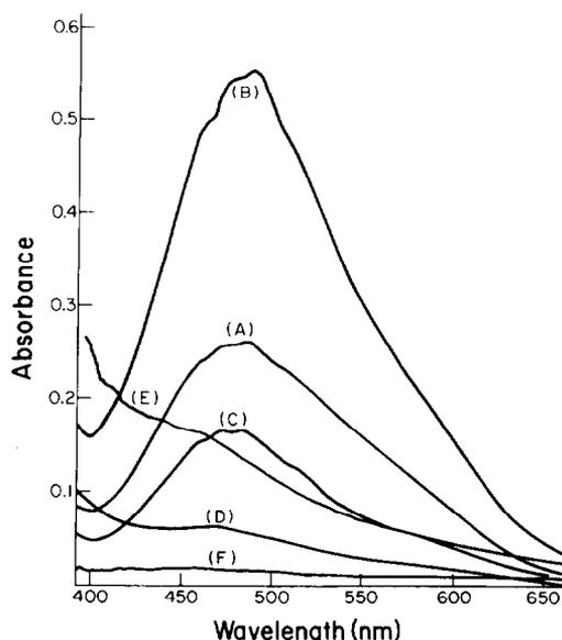
Fig. 3. Absorption spectra recorded after 15 min of mixing  $[MnY]_{aq}$  with hydrogen peroxide. (A)  $[MnY]_{aq} = 10 \text{ mM}$  ( $pH = 6.31$ ); (B)  $[MnY]_{aq} = 6 \text{ mM}$  ( $pH = 7.12$ ); (C)  $[MnY]_{aq} = 4 \text{ mM}$  ( $pH = 7.88$ ); (D)  $[MnY]_{aq} = 2 \text{ mM}$  ( $pH = 10.03$ ); (E)  $[MnY]_{aq} = 2.5 \text{ mM}$  ( $pH = 10.67$ ); and (F)  $[MnY]_{aq} = 2.5 \text{ mM}$  (no peroxide).
