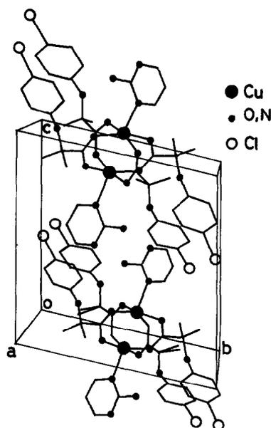
Fig. 2. Packing of (1) in the unit cell.
