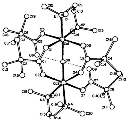
Fig. 2. Drawing of the structure and labeling of atoms of  $\text{Co}_2(\text{OH}_2)(\text{CCl}_3\text{CO}_2)_4(\text{tmen})_2$ . Distances and angles are given in Table 3.
