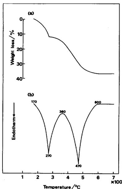
Fig. 1. (a) Thermogravimetry and (b) differential thermal analysis curves for starting powder B.
