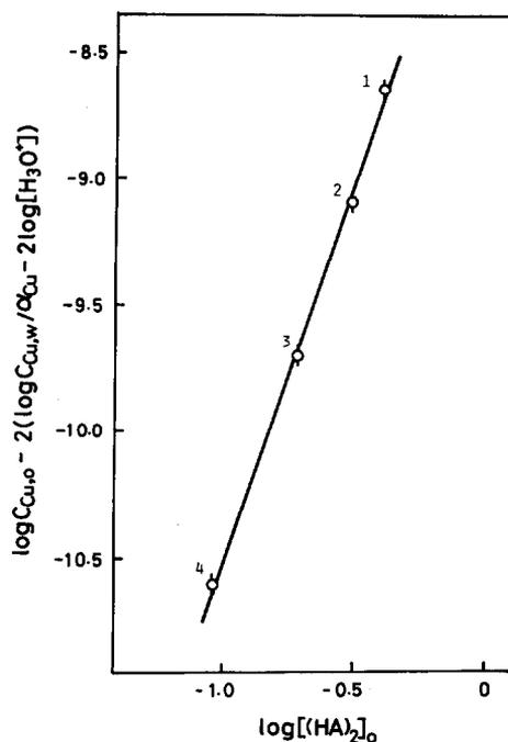
Fig. 4. Determination of the number of  $\alpha$ -bromovaleric acid involved in the extracted species. Labelling as in Fig. 3.
