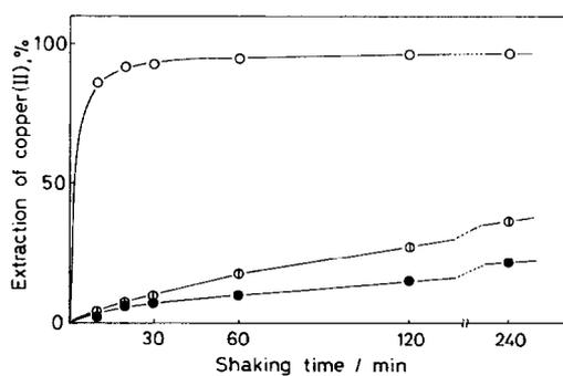
Fig. 3. Effect of shaking time on extraction of copper(II) ( $1 \times 10^{-4}$  M) by  $L^1$ ,  $L^2$  and  $L^3$  ( $1 \times 10^{-3}$  M) at pH 6.7. (●)  $L^1$ , (○)  $L^2$ , and (⊙)  $L^3$ .
