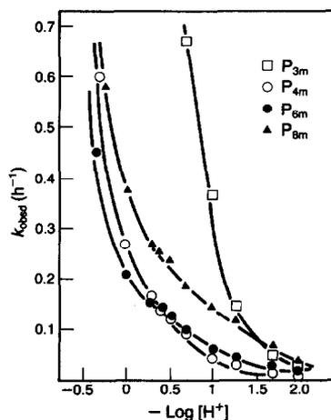
Fig. 2. Hydrolysis rate constants for cyclophosphates at various acid strengths at  $40^\circ\text{C}$ .
