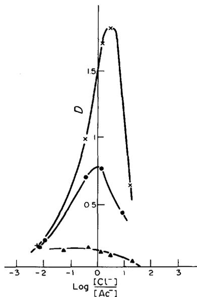
Fig. 2. Uranyl extraction by mixed substrates of different total concentrations: (x) 2.0 N, (●) 1.0 N, and (▲) 0.2 N.  $\text{UO}_2^{2+} = 9.94 \times 10^{-4} \text{ mol dm}^{-3}$ .
