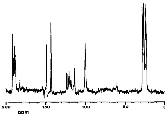
Fig. 2.  $^{13}\text{C}$ -NMR spectrum of **I** in the solid state using CP/MASS.
