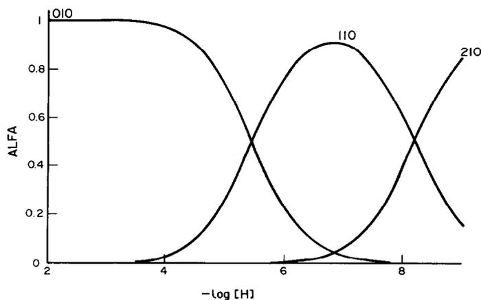
Fig. 2. Distribution plot of the species which contain copper(II). In the figure 010, 110 and 210, refer respectively to Cu(II), Cu(hnca) and Cu(hnca)<sub>2</sub>. ALFA is the ratio of each species concentration to the total copper(II) concentration.
