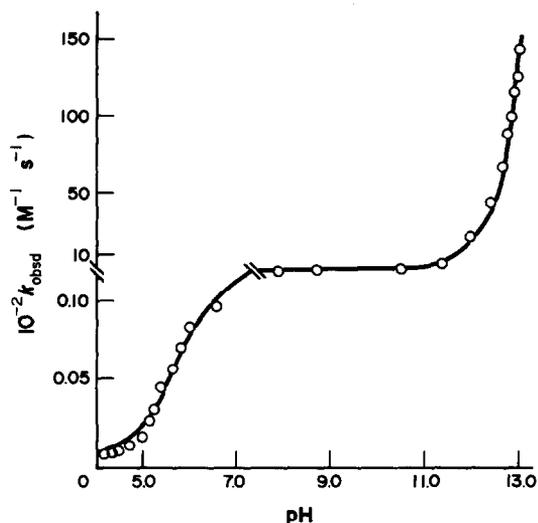
Fig. 1. pH dependence of the oxidation of hydroxylamine by  $W(CN)_8^{3-}$ :  $[W(CN)_8^{3-}] = 5 \times 10^{-4} M$ ,  $[NH_2OH] = 5 \times 10^{-3} M$ ,  $\mu = 0.1 M$  (NaCl),  $T = 25^\circ C$ . The solid curve is the computer fit.
