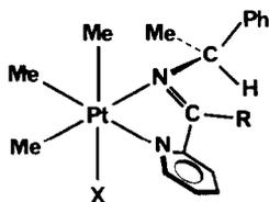
Fig. 1. Structure of the Schiff base complexes [IA, R = H, X = Cl; IB, R = H, X = Br; IC, R = H, X = I; IIA, R = Me, X = Cl; IIB, R = Me, X = Br; IIC, R = Me, X = I].
