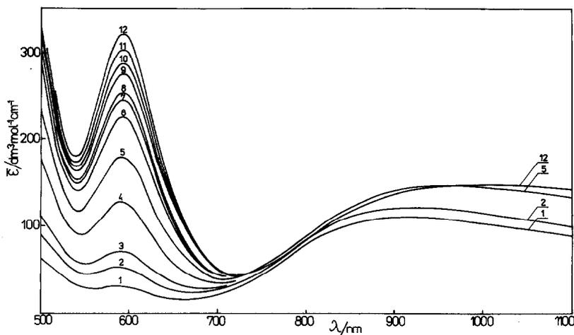
Fig. 4. Visible absorption spectra of  $\text{CuBr}_2$  solutions in DMF at  $25^\circ\text{C}$ . The molar concentrations of  $\text{CuBr}_2$  are: (1) 0.0004834, (2) 0.0007023, (3) 0.0009793, (4) 0.001953, (5) 0.003644, (6) 0.007327, (7) 0.01022, (8) 0.01319, (9) 0.02021, (10) 0.02682, (11) 0.04020, (12) 0.05536.
