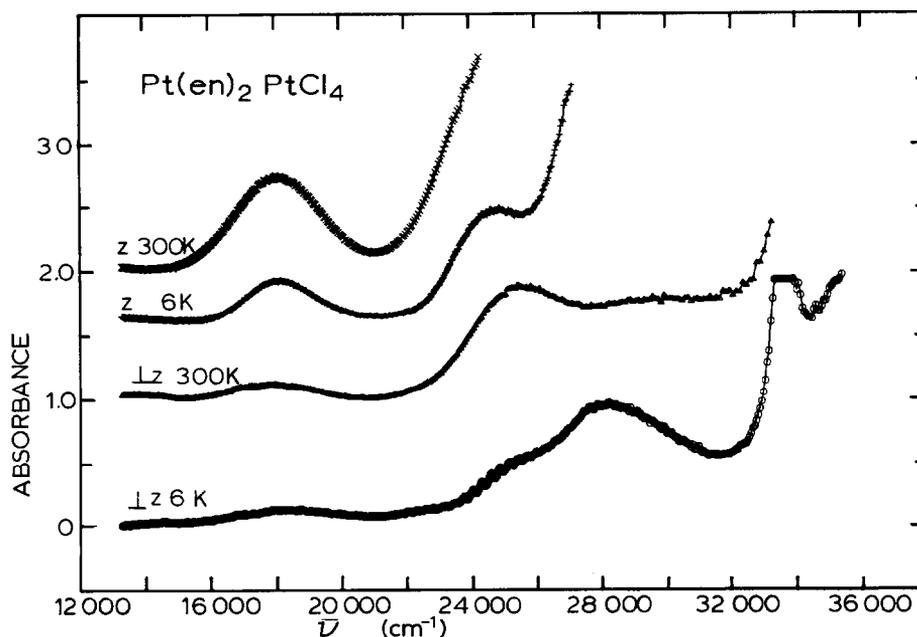
Fig. 5. Polarized single-crystal spectra for  $\text{Pt}(\text{en})_2\text{PtCl}_4$  crystal,  $16 \mu\text{m}$  thick.
