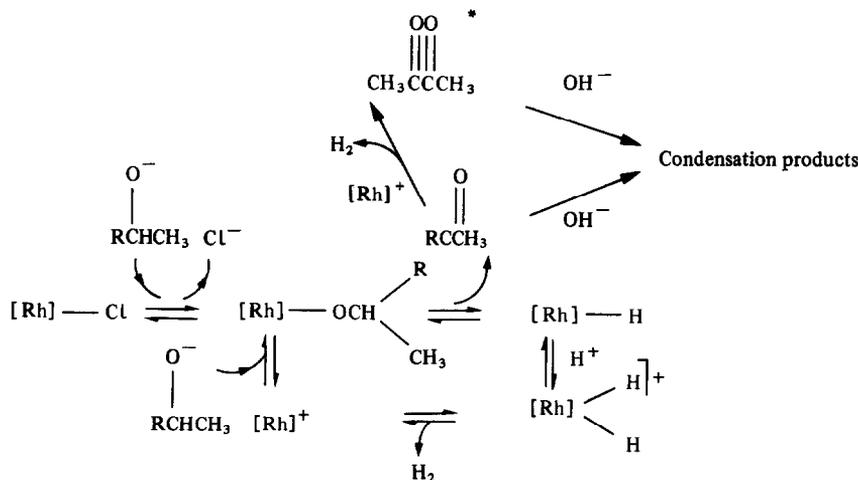
Scheme 1. Proposed mechanism for hydrogenation of secondary alcohols catalyzed by [RhCl(PPh<sub>3</sub>)<sub>3</sub>][Rh] = [Rh(PPh<sub>3</sub>)<sub>2</sub>], R = Me or MeCH(OH). Similar mechanisms can be proposed for the other catalysts employed in this study. \* R = CH<sub>3</sub>CH(OH)<sup>-</sup>.
