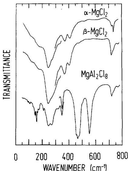
Fig. 3. IR spectra of the two crystal modifications of  $\text{MgCl}_2$  and  $\text{MgAl}_2\text{Cl}_8$ .
