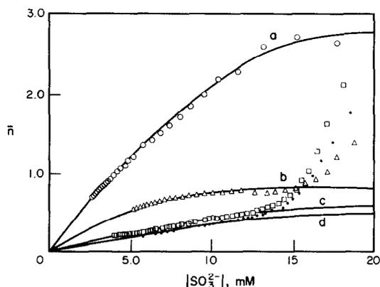
Fig. 1. Formation curves for the solutions measured. The relationship between  $C_{\text{SO}_3^{2-}}/C_{\text{HSO}_3^-}$  were: a = 100:1, b = 40:1, c = 20:1, d = 10:1.
