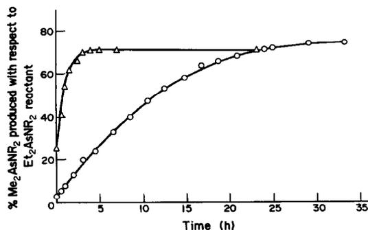
Fig. 2. Percentage of  $\text{Me}_2\text{AsNR}_2$  formed as a function of time at 24°C: (O)  $\text{Me}_2\text{AsAsMe}_2$ – $\text{Et}_2\text{AsNMe}_2$  system, (Δ)  $\text{Me}_2\text{AsAsMe}_2$ – $\text{Et}_2\text{AsNET}_2$  system.
