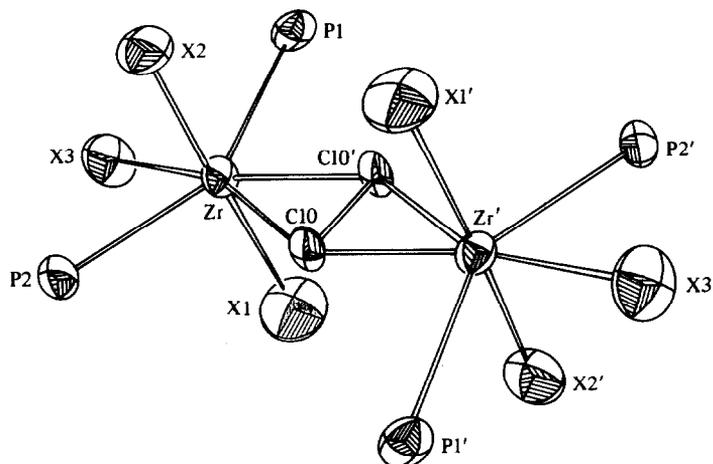
Fig. 1. ORTEP drawing of  $[\text{ZrX}_3(\text{PR}_3)_2]_2(\text{CH}_2\text{CH}_2)$  molecule with the atom-labelling scheme. The carbon atoms of the  $\text{PR}_3$  ligands are removed for clarity. Atoms are represented by their ellipsoids at the 50% probability level.
