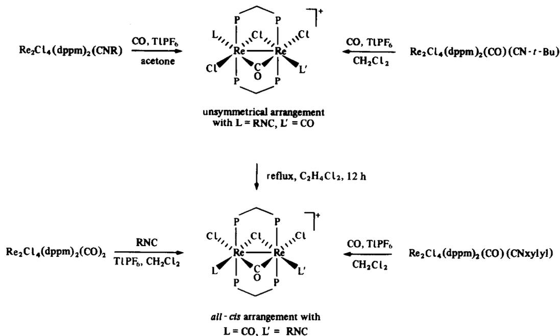
Scheme 2. Synthesis and isomerization of  $[\text{Re}_2\text{Cl}_3(\text{dppm})_2(\text{CO})_2(\text{CNR})]\text{PF}_6$  ( $\text{R} = t\text{-Bu}$  or xylyl).
