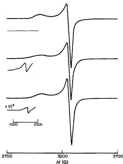
Fig. 1. Polycrystalline X-band ESR spectra of complexes A, C and E at room temperature. (frequency = 9.435 GHz).
