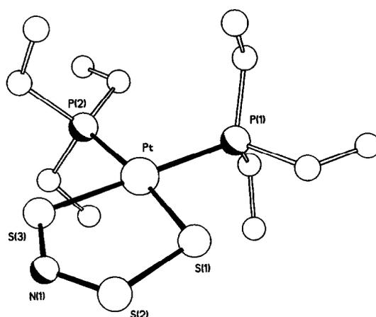
Fig. 1. The X-ray crystal structure of the cation in (2a); selected bond lengths and angles S(1)—S(2) 2.034(5), S(2)—N(1) 1.502(11), N(1)—S(3) 1.632(10), Pt—S(1) 2.287(3), Pt—S(3) 2.290(3), Pt—P(1) 2.321(3), Pt—P(2) 2.319(3) Å, S(1)—Pt—S(3) 89.8(1), Pt—S(1)—S(2) 103.6(1), S(1)—S(2)—N(1) 111.7(4), S(2)—N(1)—S(3) 124.8(7), N(1)—S(3)—Pt 110.1(4)°.
