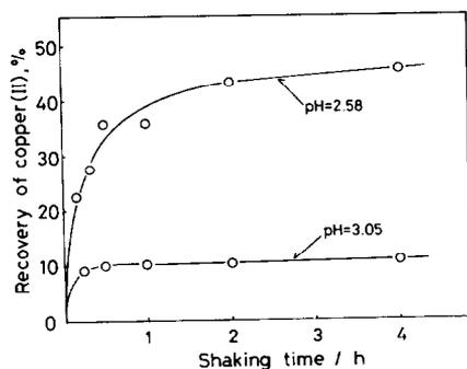
Fig. 5. Back-extraction of copper(II) ( $1 \times 10^{-4}$  M) with acidic solutions after complete extraction by  $L^2$  ( $1 \times 10^{-3}$  M).
