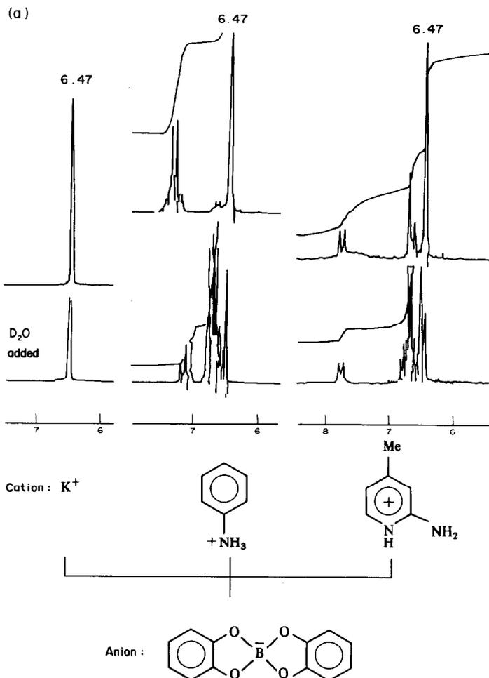
Fig. 2. (a) <sup>1</sup>H-NMR spectra of spiroborates 2, 5 and 7 (90 MHz) (deuterium oxide was added in the spectra below). (b) <sup>1</sup>H-NMR spectra of spiroborate 8 (90 MHz). (c) <sup>1</sup>H-NMR spectra of spiroborate 11 (60 MHz).
