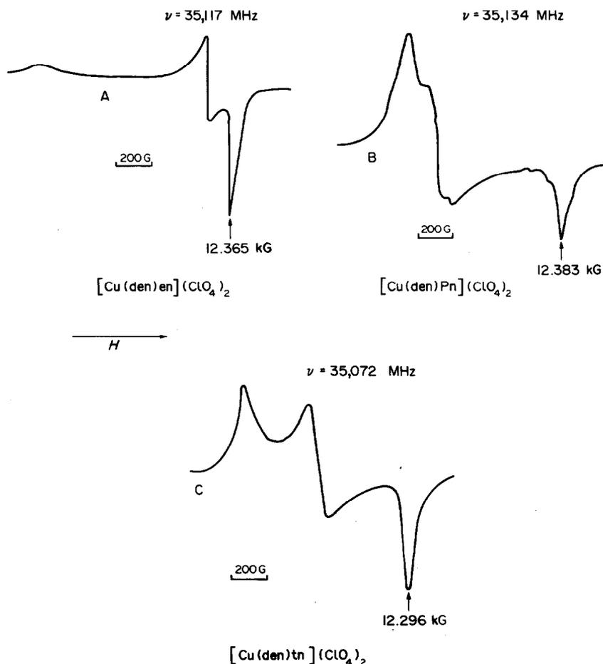
Fig. 1. ESR spectra of the polycrystalline mixed-ligand copper(II) complexes at Q-band (A, B and C) microwave frequencies.
