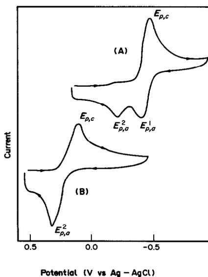
Fig. 2. Cyclic voltammograms of: (A) Fe(acac)<sub>3</sub>, and (B) Fe(tfp)<sub>3</sub>, in dimethylsulphoxide solution. Scan rate 100 mV s<sup>-1</sup>.
