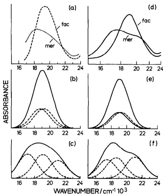
Fig. 4. Comparison of the experimental band shape for the  ${}^1T_{1g} \leftarrow {}^1A_{1g}$  transition of: (a) *fac*- and *mer*-Co(Gly) $_3$  (Refs 2 and 11), and (d) *fac*- and *mer*-Co( $\beta$ Ala) $_3$  (Ref. 7), with the simulated band shape for: (b) *fac*- and (c) *mer*-Co(Gly) $_3$ ; and (e) *fac*-, and (f) *mer*-Co( $\beta$ Ala) $_3$ . Note the nonlinearity of the wavenumber scale in (d) (Ref. 7).
