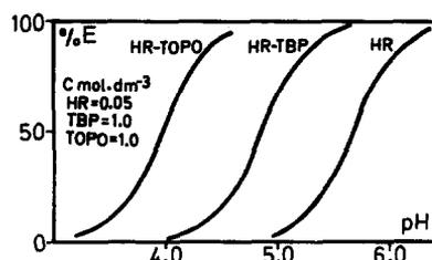
Fig. 5. Percentage extraction of Cd(II) as a function of pH with the chelating reagent and the synergic mixtures.
