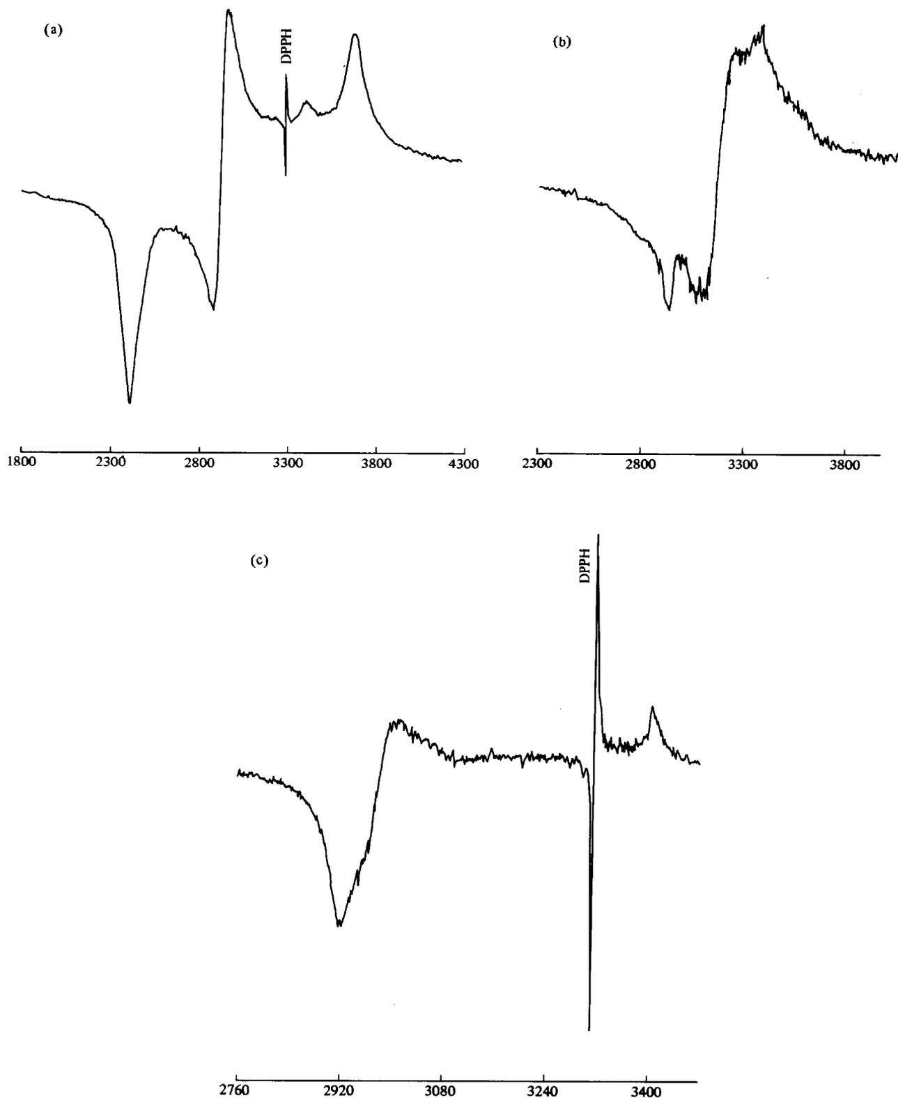
Fig. 1. Solid-state ESR spectra at 293 K (field  $H$  in Gauss): (a)  $[\text{RuL}_2\text{Cl} \cdot \text{DMF}]$ , (b)  $[\text{RuL}_2\text{Cl}(\text{py})] \cdot \text{H}_2\text{O}$ , and (c)  $[\text{RuLCl}_2(o\text{-phen})] \cdot \text{H}_2\text{O}$ .
