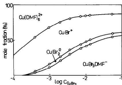
Fig. 9. Formation diagram for the copper(II) complexes in DMF solutions of  $\text{CuBr}_2$  at  $25^\circ\text{C}$ .
