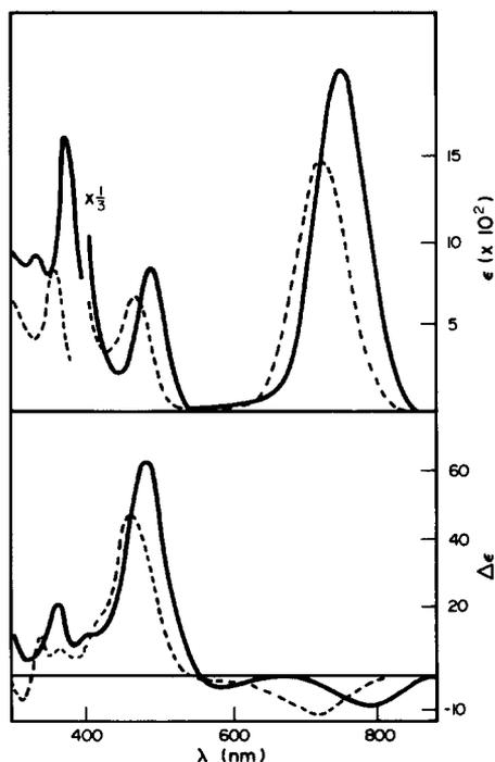
Fig. 8. Absorption and CD spectra of  $\Lambda$ -[Mo<sub>2</sub>Br<sub>4</sub>(S,S-dppb)<sub>2</sub>] (full line) and  $\Lambda$ -[Mo<sub>2</sub>Cl<sub>4</sub>(S,S-dppb)<sub>2</sub>] (dashed line), both in dichloromethane solution.
