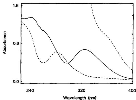
Fig. 4. Comparison of the electronic absorption spectra of  $\text{Mo}_2(\text{NMe}_2)_6$  (solid line) and  $\text{W}_2(\text{NMe}_2)_6$  (dashed line) in THF solutions, at  $3.5 \times 10^{-5}$  M.
