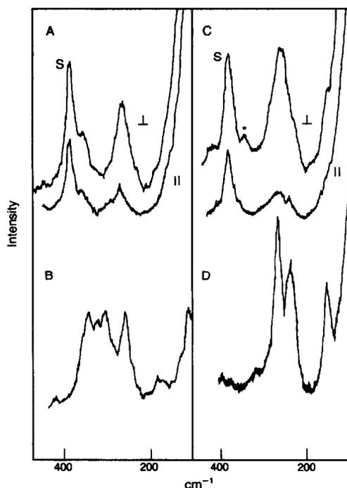
Fig. 1. Raman spectra of chloroselenate(II)s: (A)  $\text{Et}_4\text{NSeCl}_3$  in  $\text{CH}_3\text{CN}$  (0.25 M), (B) solid  $\text{Et}_4\text{NSeCl}_3$ , (C)  $(\text{Et}_4\text{N})_2\text{SeCl}_4$  in  $\text{CH}_3\text{CN}$  (0.25 M), and (D) solid  $(\text{Et}_4\text{N})_2\text{SeCl}_4$ . S = solvent band; \* =  $\text{SeCl}_3^-$  band.
