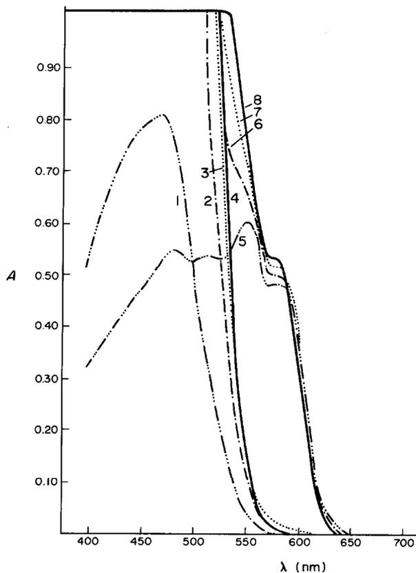
Fig. 2. pH influence on the spectra of DAB and its Pd(II) complex extracted with isoamlic alcohol.  $[DAB] = 27.8 \times 10^{-5} \text{ M}$ ;  $[Pd(II)] = 2.8 \times 10^{-5} \text{ M}$ . Curves 1, 2, 3 and 4: DAB reagent at pH 2.1, 3.2, 4.0 and 5.1. Curves 5, 6, 7 and 8: DAB-Pd(II) complex at pH 2.1, 3.2, 4.0 and 5.1.
