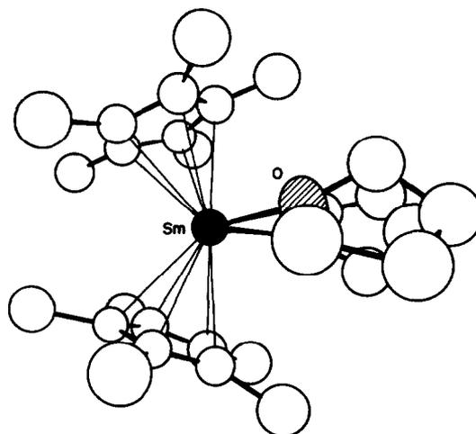
Fig. 3. Side view of the structure of  $(C_5Me_5)_2Sm(thf)_2$ . The two thf molecules overlap such that only one oxygen atom can be seen from this perspective.
