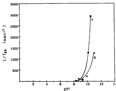
Fig. 9. Dependence of the  $^{14}\text{N}$  paramagnetic transverse relaxation rate of proline upon pH, for Solution E (1.5 M proline and 0.02 M  $\text{CoCl}_2$ ) and Solution F (1.0 M proline and 1.0 mM  $\text{CuCl}_2$ ), at 300 K. The spectrometer frequency was 18.075 MHz.
