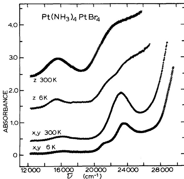
Fig. 8. Polarized spectra for  $\text{Pt}(\text{NH}_3)_4\text{PtBr}_4$  crystal,  $8 \mu\text{m}$  thick.
