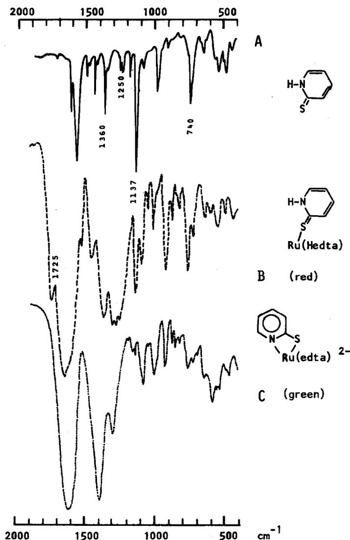
Fig. 2. IR spectra of the 2-mercaptopyridine ligand (A), and of the red (B) and green (C) complexes with Ru(III)(edta) in KBr pellets.
