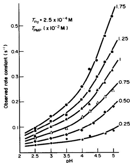
Fig. 6. Dependence of  $k_{\text{obs}}(\text{PMP})$  on pH at various  $T_{\text{PMP}}$  values.
