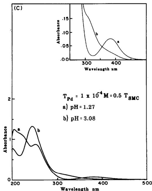
Fig. 1. Spectra of Pd(II)–Meth and Pd(II)–SMC systems at representative pH values. (A) Spectra of Pd(II) at the indicated pH values. (B) Spectra of Pd(II)–Meth at the indicated pH values. (C) Spectra of Pd(II)–SMC at the indicated pH values.
