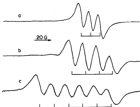
Fig. 4. Typical ESR spectra obtained during the interaction of  $\text{Fe(NO)} \cdot \text{L}_2$  with Lewis acids in ethanol at 298 K: (a)  $\text{Fe(NO)(Et-xant)}_2$ , (b)  $\text{Fe(NO)}_2 \cdot \text{Br} \cdot \text{L}$ , and (c)  $\text{Fe(NO)}_2 \cdot \text{I} \cdot \text{L}$ . L is coordinated Et-xant.
