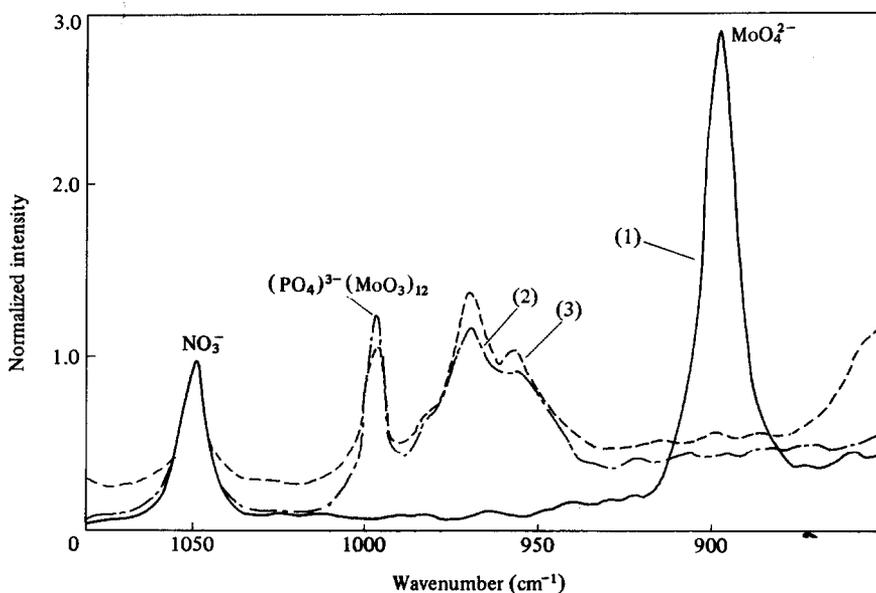
Fig. 3. The acidification of the mixed solution of molybdate and phosphate ( $[\text{P}] = 1.0 \times 10^{-2}\text{ M}$ ,  $[\text{Mo}] = 1.2 \times 10^{-1}\text{ M}$ , pH 1). The reaction time: (1) 0 s, (2) 31 s, (3) 20 min 30 s.
