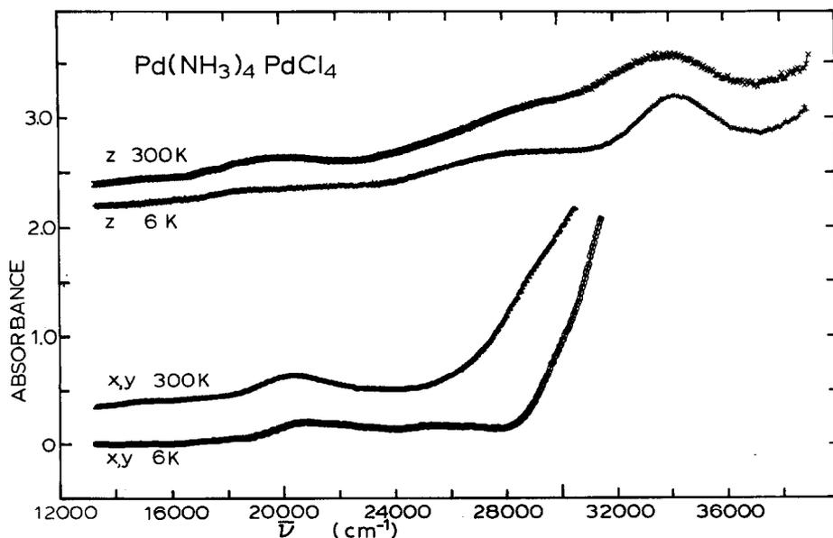
Fig. 17. Polarized spectra for  $\text{Pd}(\text{NH}_3)_4\text{PdCl}_4$  crystal,  $3.1\ \mu\text{m}$  thick.
