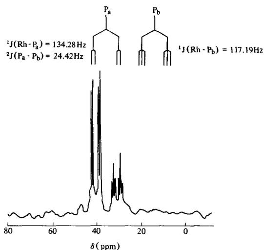
Fig. 1.  $^3\text{1P}\{^1\text{H}\}$  NMR spectrum of  $[\text{Rh}(\text{DPEA})(\text{PPh}_3)]\text{BPh}_4$ .
