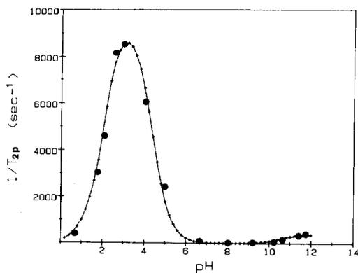
Fig. 10. Dependence of the  $^{17}\text{O}$  paramagnetic transverse relaxation rate of proline upon the measured pH of a solution containing 0.25 M proline and 0.3 mM  $\text{CuCl}_2$  (Solution G). The experimental points were recorded at 24.4 MHz, and 300 K, and the dotted line is the least-squares fit of the experimental points to eq. (28), with the constants of Tables 3 and 4.
