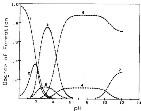
Fig. 11. Dependence of the relative concentration of all  $\text{Cu}^{2+}$ -containing species upon pH, for Solution F. All curves were constructed with the stability constants of Table 3. 1 is the free  $\text{Cu}^{2+}$ , 2, 3 and 4 are the protonated complexes  $\text{CuHPro}^{2+}$ ,  $\text{CuHPro}_2^+$  and  $\text{CuHPro}_3$ , respectively, and 5, 6 and 7 are the bidentate complexes  $\text{CuPro}^+$ ,  $\text{CuPro}_2$  and  $\text{CuPro}_3^-$ , respectively.
