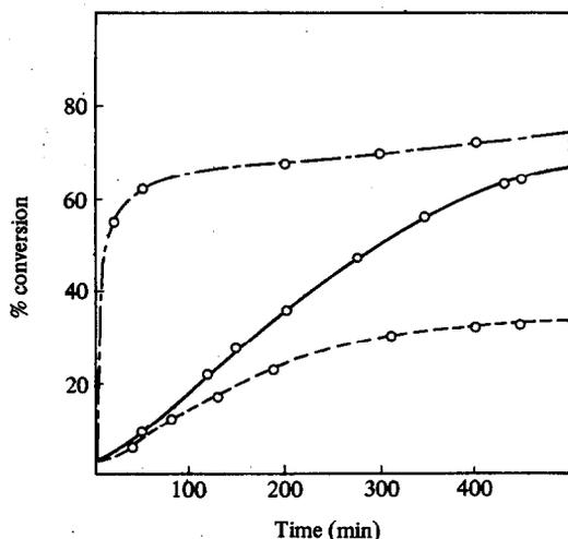
Fig. 1. Conversion of 1-heptene as function of the time catalyzed by  $[\text{Rh}(\text{COD})(\text{Ph}_3\text{PS})_2](\text{ClO}_4)$  (○—○),  $[\text{Rh}(\text{NBD})(\text{Ph}_3\text{PS})_2](\text{ClO}_4)$  (○---○) and  $[\text{Ir}(\text{COD})(\text{Ph}_3\text{PS})_2](\text{ClO}_4)$  (○-·-·-○).
