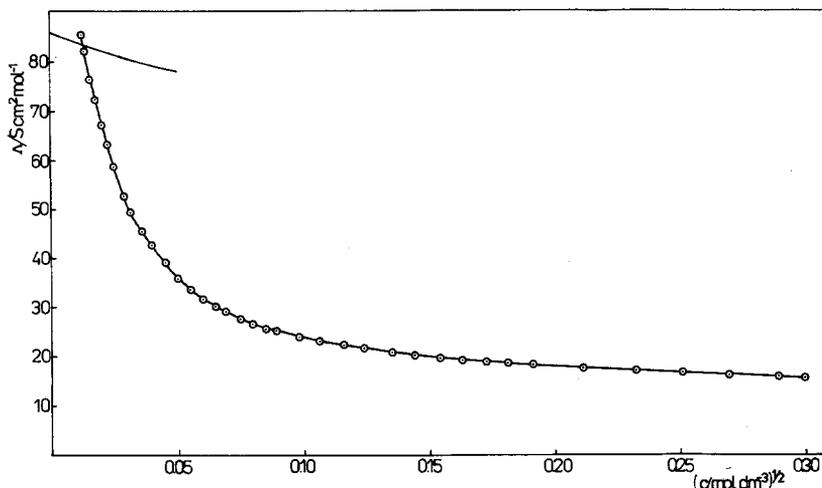
Fig. 6. Plot of the molar conductance of  $\text{CuBr}_2$  in DMF solutions against the square of concentration at  $25^\circ\text{C}$ . The solid line represents the conductometric curve predicted for the 1:1-type  $\text{CuBr}^+ \cdot \text{Br}^-$  complex electrolyte.
