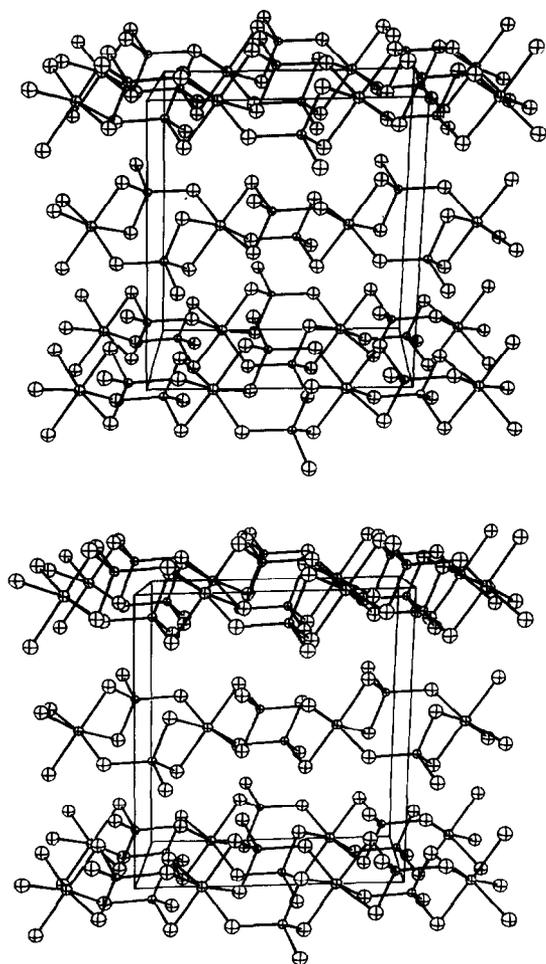
Fig. 6. A stereographic plot of the unit cell of  $\text{MgAl}_2\text{Cl}_8$ . The viewer looks along the  $b$ -axis, and the  $a$ -axis points upwards in the paper plane.
