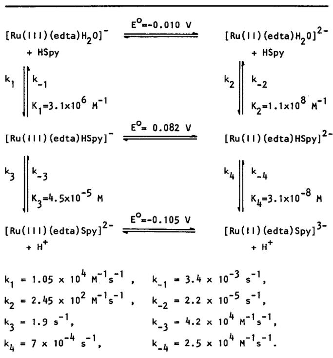
Fig. 6. Thermodynamic cycle for the ruthenium(III)/(II)-(edta) complexes of 2-mercaptopyridine ( $25^{\circ}\text{C}$ ,  $I = 0.10$  M Lipts, pH 4.54 acetate buffer).
