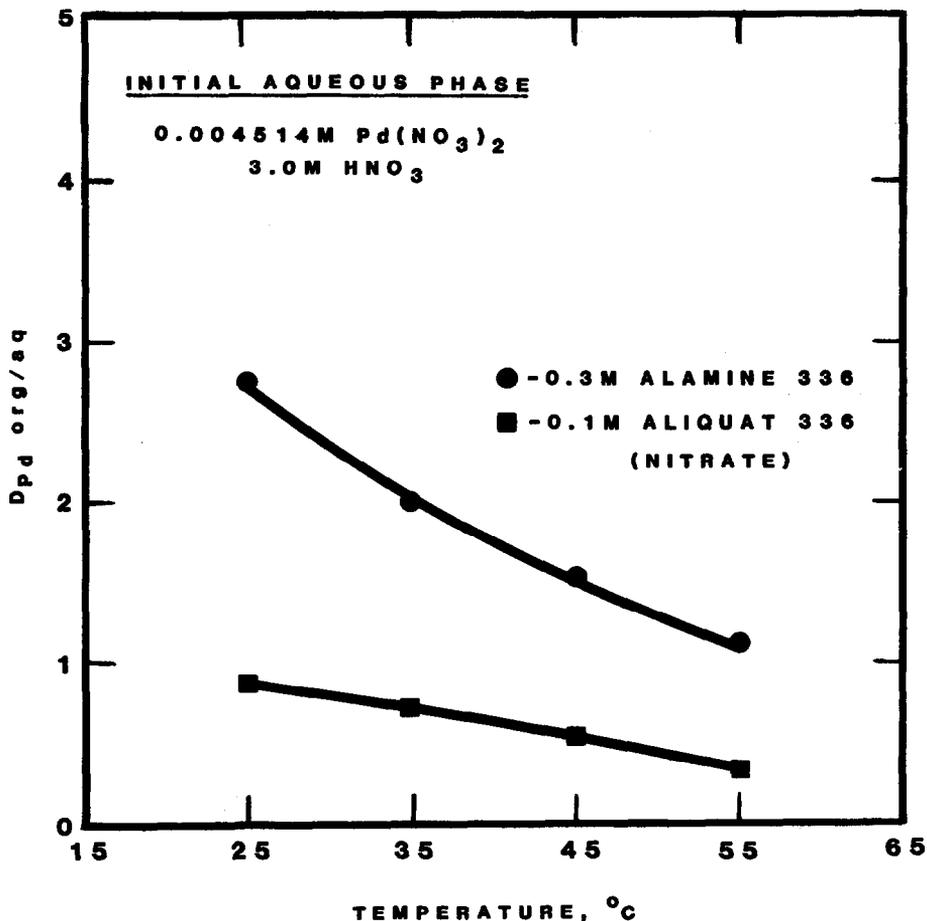
Fig. 3. Pd distribution coefficients as a function of temperature using an extracting solution containing either 0.3 M Alamine 336 or 0.1 M Aliquat 336 (nitrate) with a TBP/kerosene volumetric ratio of 0.667.
