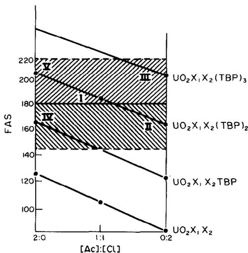
Fig. 1.  $\text{UO}_2^{2+}$ -Ac-Cl-TBP packing diagram.  $\text{X}_1 = \text{Ac}^-$ ,  $\text{X}_2 = \text{Cl}^-$ .
