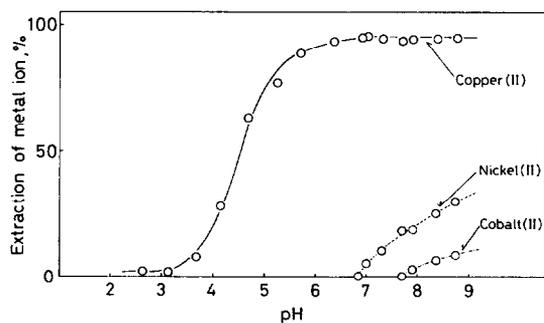
Fig. 4. pH dependence of extraction of metal ions ( $1 \times 10^{-4}$  M) by  $L^2$  ( $1 \times 10^{-3}$  M). Shaking time 2 h.
