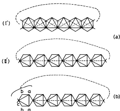
Fig. 4. (a) Cyclic polymers derived from I and II and path; I' with general formula of  $M_nO_{4n}$  and II' with that of  $M_nO_{5n}$ . They have an identical Euler's characteristic;  $\chi = n$ . (b) Connectivity and path in cyclic polymer II'. Only when the cyclization is completed at point *c* does one closed linkage exist.
