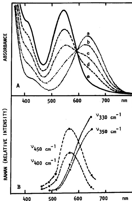
Fig. 1. (A) Electronic spectra of the Ru(III)(edta) complex with 2-mercaptopyridine at pH (a) 6.2; (b) 5.1; (c) 4.4; (d) 4.1; (e) 3.2. (B) Resonance Raman profiles for the most enhanced vibrational bands of the red complex ( $400, 450\text{ cm}^{-1}$ ) and of the green complex ( $330, 350\text{ cm}^{-1}$ ).
