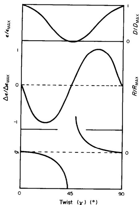
Fig. 6. Variation of dipole strength ( $D$ ) (and  $\epsilon$ ), rotational strength ( $R$ ) (and  $\Delta\epsilon$ ) and  $g$  value with twist angle  $\chi$  (for the  $\delta_{xy} \rightarrow \delta_{xy}^*$  transition of a complex with the  $\Lambda$  absolute configuration).
