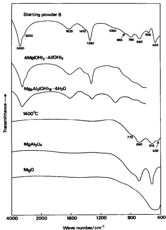
Fig. 3. Infrared absorption spectra for starting powder B,  $4\text{Mg}(\text{OH})_2 \cdot \text{Al}(\text{OH})_3$ ,  $\text{Mg}_6\text{Al}_2(\text{OH})_{18} \cdot 4\text{H}_2\text{O}$ , specimen quenched after heating B to  $1300^\circ\text{C}$ ,  $\text{MgAl}_2\text{O}_4$ , and  $\text{MgO}$ .
