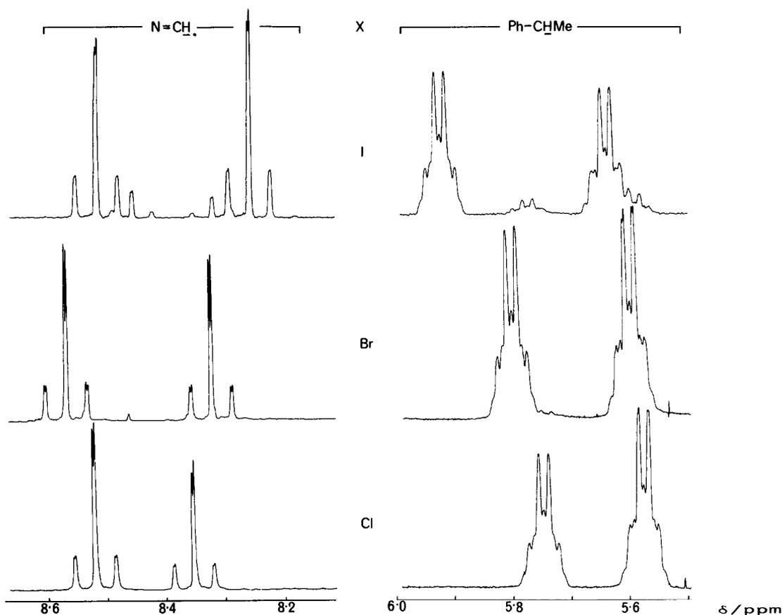
Fig. 3. 400-MHz  $^1\text{H}$  NMR spectra of complexes IA-C showing the  $\text{N}=\text{CH}$  (left) and  $\text{Ph}-\text{CH}$  (right) proton signals.
