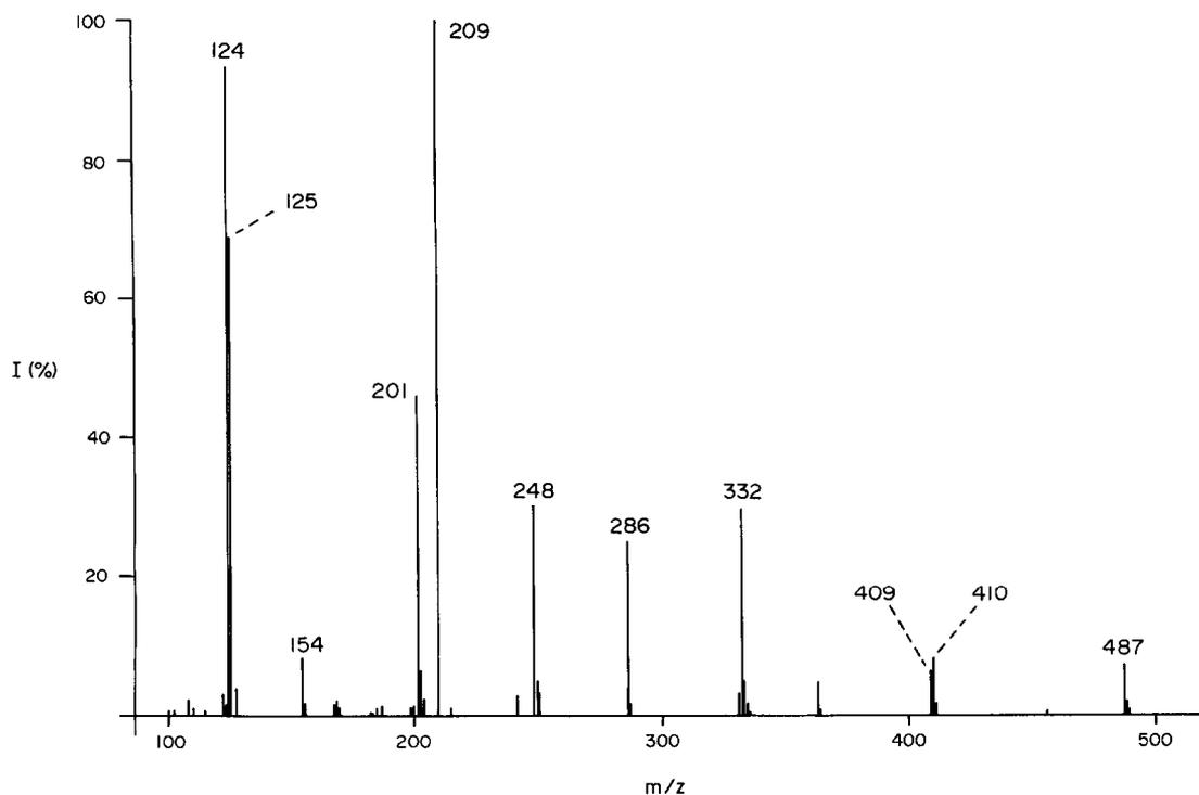
Fig. 3. Mass spectrum of IV, EI, 70 eV, 170°C, int.  $\geq 0.2\%$ ,  $m/z \geq 100$ .
