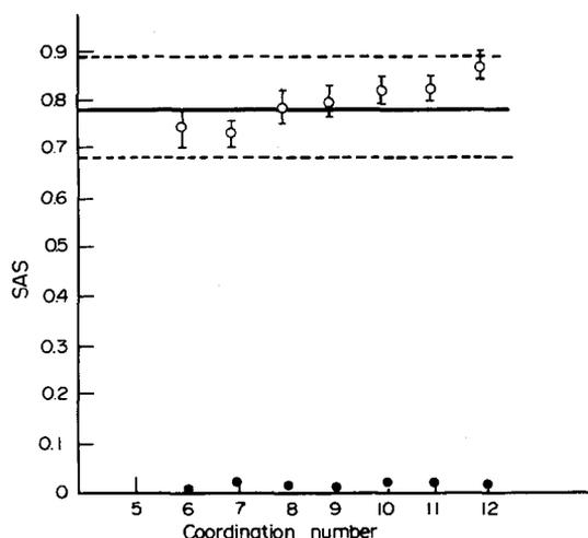
Fig. 3. The Packing Saturation Rule and the Packing Centre Rule. The stable region is described with a centre line at the SAS equal to the average steric crowding and two border lines of either gain or loss of one ligand with an SAF of 0.1.
