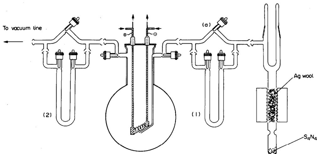
Fig. 1. Apparatus used for the preparation and reaction of  $S_2N_2$  with nickel vapour.
