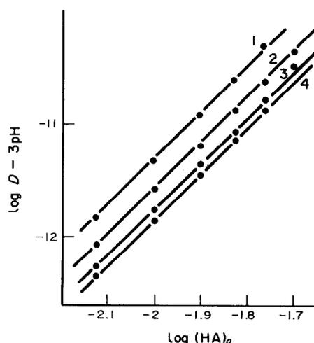
Fig. 2. Extraction of Nd(III) with various  $C_{HA}$  in different organic solvents: (1)  $CCl_4$ , (2) benzene, (3) toluene, and (4) xylene.
