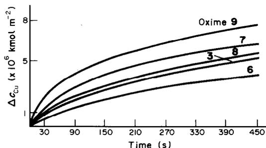
Fig. 1. Influence of the structure of oxime upon the amount of copper transferred into xylene phase (pH = 3.0,  $c_{\text{Cu}^{2+}} = 0.015 \text{ mol dm}^{-3}$ ,  $c_{\text{oxime}} = 0.025 \text{ mol dm}^{-3}$ ).
