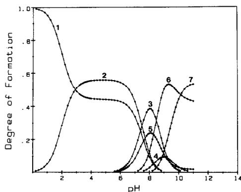
Fig. 13. Dependence of the relative concentration of all  $\text{Mn}^{2+}$  containing species upon pH, for Solution I, at 300 K. All curves were constructed with the stability constants of Table 5. (1) Is the free  $\text{Mn}^{2+}$ , (2), (3) and (4) are the protonated complexes  $\text{MnHG}^{2+}$ ,  $\text{MnHG}_2^+$  and  $\text{MnHG}_3$ , respectively, whereas (5), (6) and (7) are the bidentate complexes  $\text{MnG}^+$ ,  $\text{MnG}_2$  and  $\text{MnG}_3^-$ , respectively.
