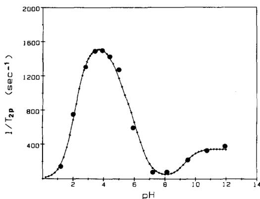
Fig. 1. Dependence of the <sup>17</sup>O paramagnetic transverse relaxation rate of glycine upon the measured pH of a solution containing 0.31 M glycine and 5.0 mM CoCl<sub>2</sub> (Solution A). The experimental points were recorded at 24.4 MHz, 300 K, and the dotted line is the least-squares best fit of the experimental points to eqn (9), with the constants of Tables 1 and 2.
