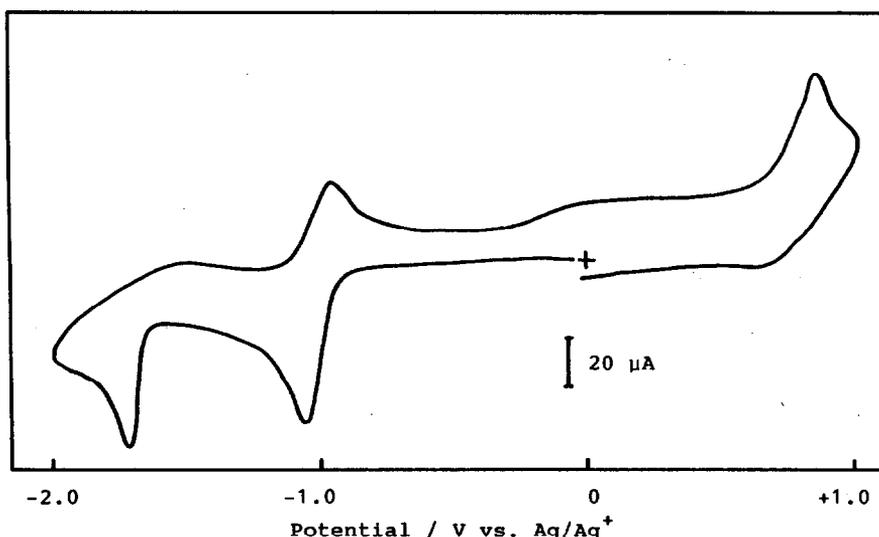
Fig. 6. Cyclic voltammogram of  $\text{ReBr}(\text{CO})_3\text{Y}_{\text{N-CN}}$  in MeCN containing  $[\text{NBU}_4^+]\text{ClO}_4$  ( $0.05 \text{ mol dm}^{-3}$ ), measured with a scan rate of  $0.1 \text{ V s}^{-1}$ .
