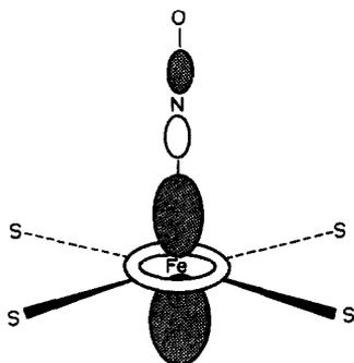
Fig. 1. The SOMO in the square pyramidal complexes  $[\text{Fe}(\text{NO})(\text{SH})_4]^{2-}$ ,  $[\text{Fe}(\text{NO})(\text{S}_2\text{CNMe}_2)_2]$  and  $[\text{Fe}(\text{NO})(\text{S}_2\text{MoS}_2)_2]^{2-}$ .
