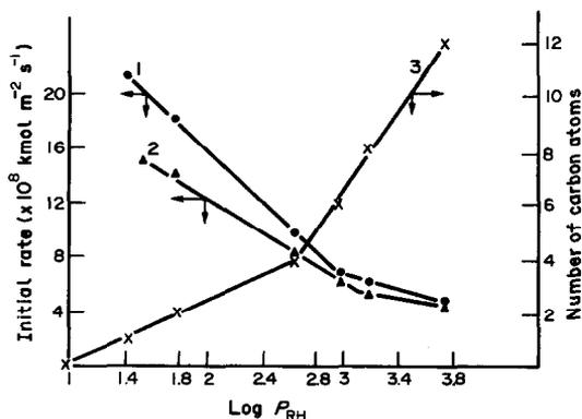
Fig. 6. Relationship between copper extraction rate and the distribution coefficient of the oximes (xylene, curves 1 and 2 =  $c_{\text{oxime}} = 0.05$  and  $0.025 \text{ mol dm}^{-3}$ , respectively; curve 3 = relationship between the distribution coefficient and the number of carbon atoms in the alkyl).
