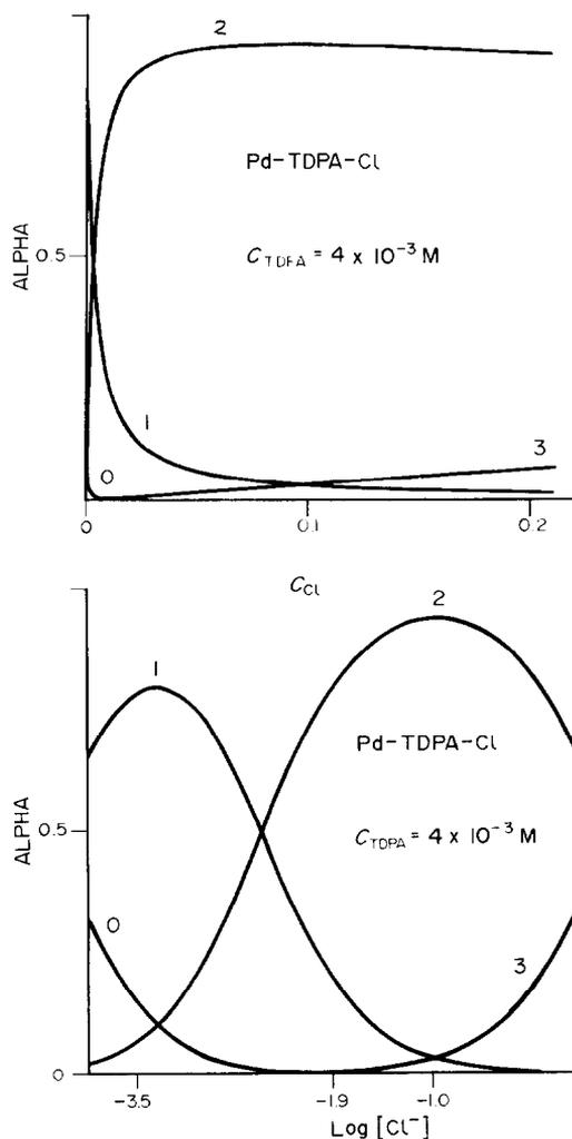
Fig. 3. Species distribution diagrams of Pd–TDPA–Cl system calculated by the Haultfall program: (0)  $[\text{Pd}(\text{TDPA})_2]$ , (1)  $\text{Pd}(\text{TDPA})_2\text{Cl}$ , (2)  $[\text{Pd}(\text{TDPA})_2\text{Cl}_2]$ , (3)  $[\text{Pd}(\text{TDPA})\text{Cl}_3]$ .
