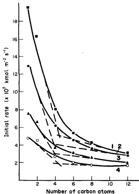
Fig. 5. Influence of the number of carbon atoms in the alkyl upon the initial extraction rate (xylene, curves 1, 2, 3 and 4 =  $c_{\text{oxime}} = 0.05, 0.025, 0.015$  and  $0.009 \text{ mol dm}^{-3}$ , respectively).
