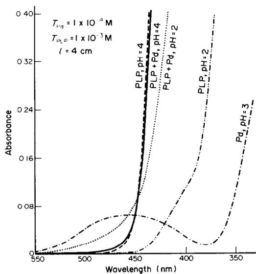
Fig. 1. Absorption spectra of Pd(II)-PLP system at various pH values.
