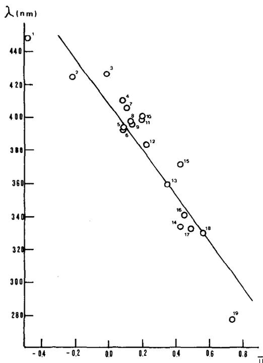
Fig. 2. Dependence from the  $\pi$ -acceptor capacity of  $\lambda_{\text{max}}$  for  $\text{Cr}(\text{CO})_5\text{L}$ .
