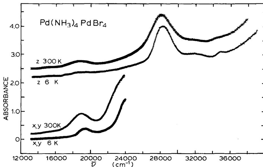
Fig. 23. Polarized spectra for  $\text{Pd}(\text{NH}_3)_4\text{PdBr}_4$  crystal,  $3.1 \mu\text{m}$  thick.
