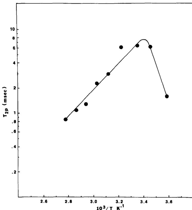
Fig. 11. Dependence of the  $^{17}\text{O}$  paramagnetic relaxation time of glycine upon inverse temperature, in a solution containing 0.19 M glycine and 1.0 mM  $\text{CuCl}_2$  (Solution H), at pH 7.3. The spectrometer frequency was 33.926 MHz.
