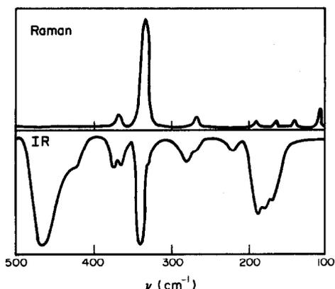
Fig. 2. Vibrational spectra of the complex  $[(\text{H}_2\text{L})_2\text{PtCl}_2]$ .
