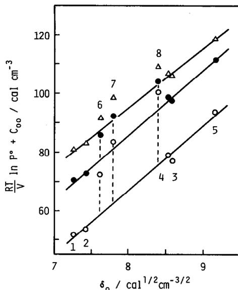
Fig. 3. Evaluation of partition coefficients with eqn (2). The numbers correspond to those in Table 2. ○ Ni(tta)<sub>2</sub>; ● Cu(tta)<sub>2</sub>;<sup>9</sup> △ Htta(enol).<sup>9</sup>
