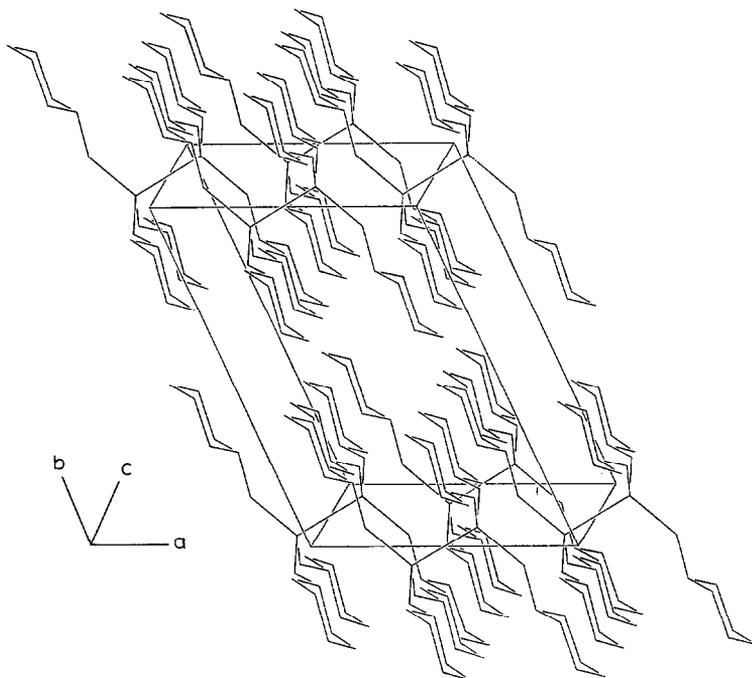
Fig. 6. A view of the unit cell of  $W_2(OCy)_6$  showing chains of the  $W_2$  units propagated along the  $a$  axis.
