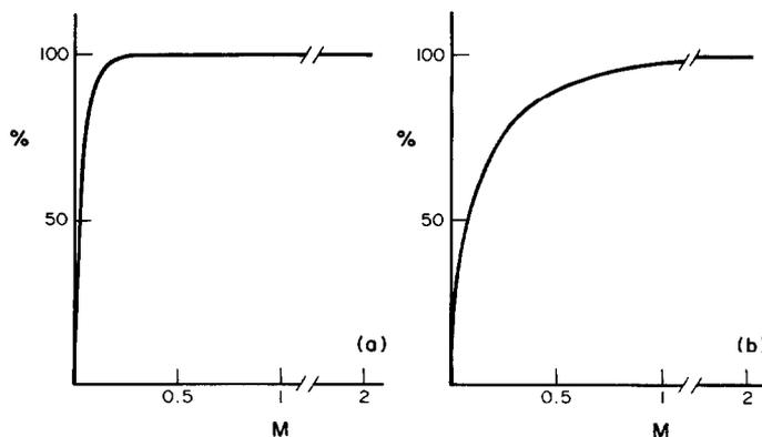
Fig. 1. Percent recovery yield for Pb(II) (a) and Cu(II) (b) from NTA filters as a function of the concentration of the stripping agent,  $10.0 \text{ cm}^3 \text{ HCl}$ .
