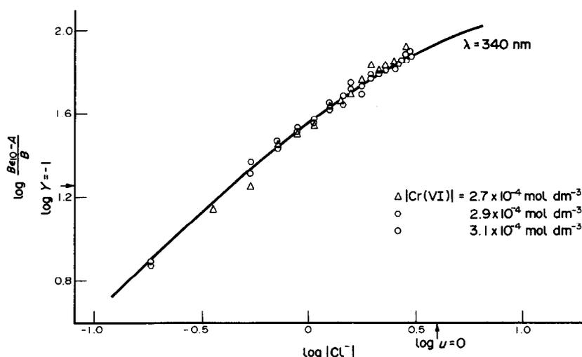
Fig. 3.  $-\log(B\epsilon_{10}-A)/B$  plotted vs  $\log[\text{Cl}^-]$  at  $\lambda = 340$  nm for different chromium(VI) concentration. The full drawn line gives  $\log Y$  as a function of  $\log u$  in the position of the best adjust.
