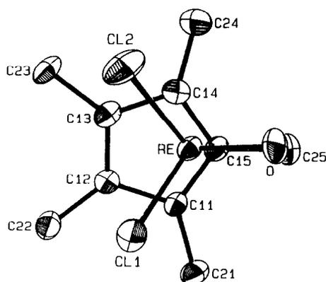
Fig. 6. ORTEP projection of compound **3b**'s molecular structure down the orthonormal vector between the plane of C(11), C(14), C(15) and the metal atom (thermal ellipsoids at 50% probability).
