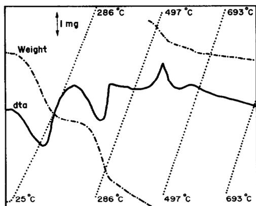
Fig. 1. TGA (---) and DTA (—) curves for  $\text{Ni}_3[\text{Fe}(\text{CN})_5(\text{isonida})_2] \cdot 13.5\text{H}_2\text{O}$ .
