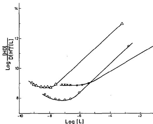
Fig. 3. Extraction of Zn(II) in the presence of ligand with  $[\text{HL}] < [\text{HCl}]$ ,  $[\text{HD}] = 1.05 \times 10^{-2}$  F. (O) Im,  $[\text{HCl}] = 0.10$  M; ( $\Delta$ ) 2MIm,  $[\text{HCl}] = 0.10$  M; ( $\times$ ) His,  $[\text{HCl}] = 0.05$  M.
