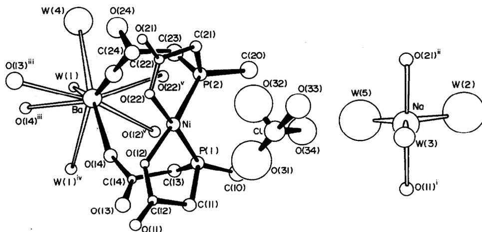
Fig. 1. Perspective view of the structure of  $BaNiG_2 \cdot NaClO_4 \cdot 5H_2O$  with closest intermolecular contacts. Hydrogen atoms (omitted for clarity) are given the numbers of their bonding partners. W denotes the oxygen atom of a water molecule. For symmetry code, see Table 2.
