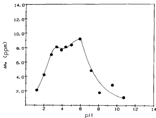
Fig. 4. Dependence of the  $^{17}\text{O}$  paramagnetic chemical shift of glycine upon pH, for Solution A, 300 K and a spectrometer frequency of 24.4 MHz.
