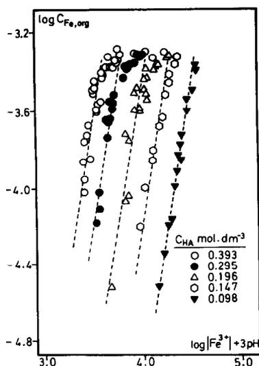
Fig. 3. Plot of the function  $\log C_{\text{Fe,org}} = f(\log |\text{Fe}^{3+}| + 3\text{pH})$  for the experimental data collected at constant total Fe(III) concentrations.
