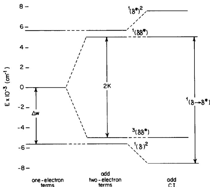
Fig. 2. Relative energies of the  $\delta, \delta^*$ -manifold of electronic states with and without configuration interaction. Parameters used are those for  $\text{Re}_2\text{Cl}_4(\text{PMe}_2\text{Ph})_4^+$  (Table 1.)
