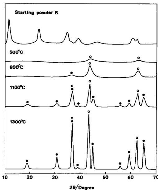
Fig. 2. X-ray diffraction patterns for starting powder B and specimens quenched after heating to various temperatures. Phases: O, MgO; ●,  $\text{MgAl}_2\text{O}_4$ .
