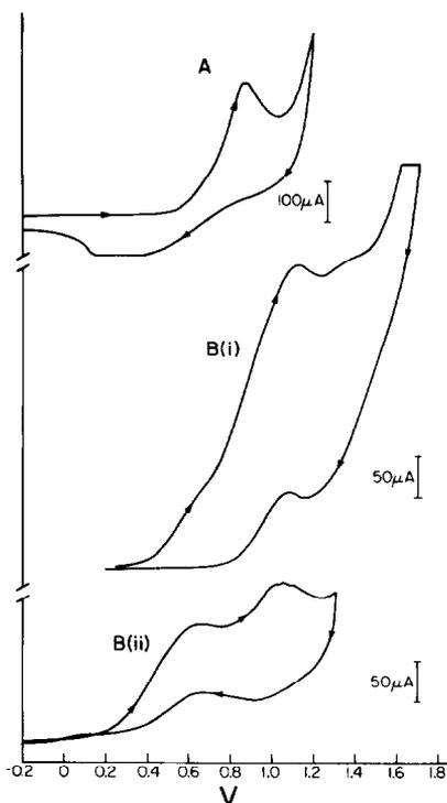
Fig. 4. Cyclic voltammograms obtained during the electro-oxidation of  $[\text{MnY}]_{\text{aq}}$ . (A) No peroxide (pH = 7.96); (B) in the presence of excess peroxide: (i) pH = 6.93; (ii) pH = 11.61.
