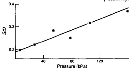
Fig. 3. Stabilization/decomposition for germilene radicals, vs total pressure. Intercept = 0.194; slope = 0.00118.
