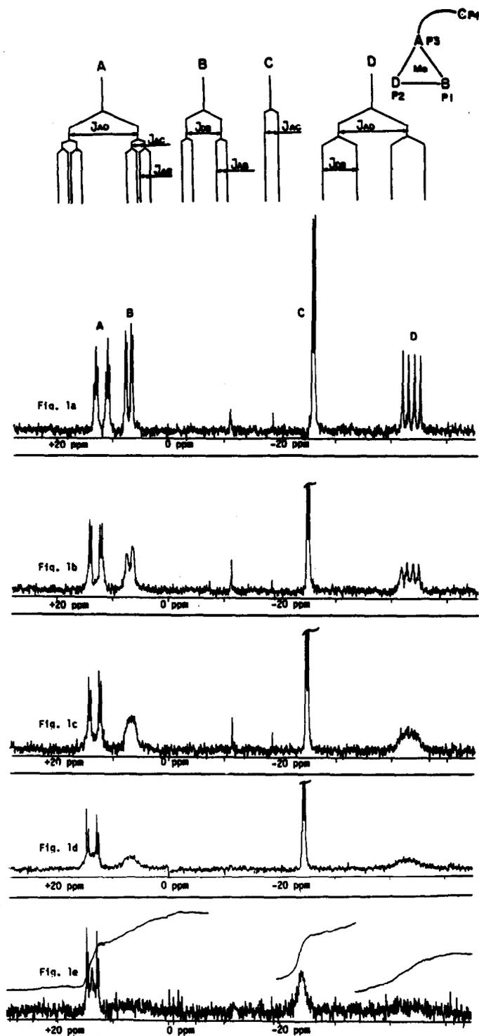
Fig. 1. Variable-temperature  $^{31}\text{P}\{-^1\text{H}\}$  NMR studies. Referenced to  $\text{H}_3\text{PO}_4$  as an external standard at room temperature. (a)  $-40^\circ\text{C}$ , (b)  $0^\circ\text{C}$ , (c)  $10^\circ\text{C}$ , (d)  $25^\circ\text{C}$ , and (e)  $40^\circ\text{C}$ . Peak assignment on top of Fig. 1a.
