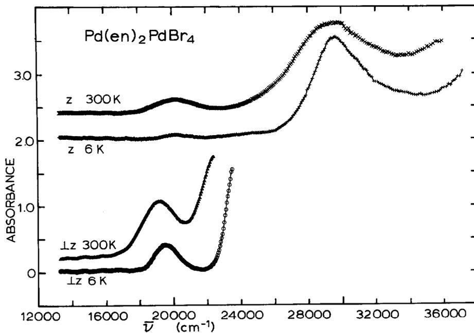
Fig. 24. Polarized spectra for  $\text{Pd}(\text{en})_2\text{PdBr}_4$  crystal,  $5 \mu\text{m}$  thick.
