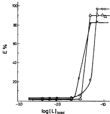
Fig. 5. Extraction of Hg(II) as function of ligand concentrations at  $[\text{HD}] = 1.05 \times 10^{-2}$  F,  $[\text{HCl}] = 0.03$  M. (○) Im, (△) 2MIm, (×) His.
