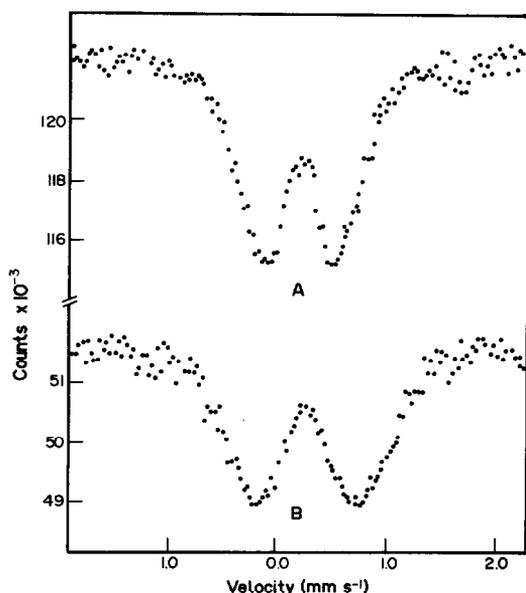
Fig. 2. Mössbauer spectra of  $\text{Fe}(\text{met})(\text{OH})\text{Cl} \cdot 2\text{CH}_3\text{OH}$ : (A) at 297 K, and (B) at 88 K.
