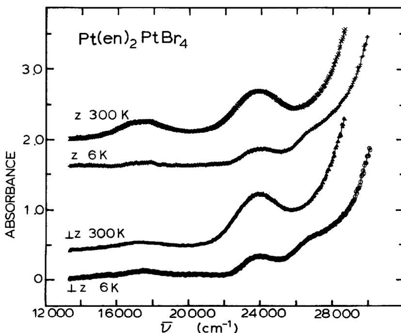
Fig. 10. Polarized spectra for  $\text{Pt}(\text{en})_2\text{PtBr}_4$  crystal,  $7 \mu\text{m}$  thick.
