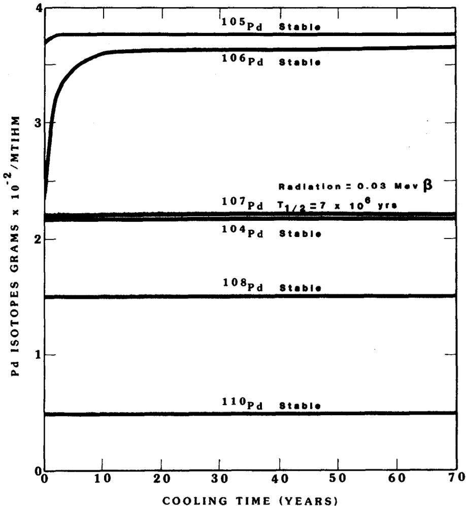
Fig. 1. Pd isotopic mix as a function of fuel cooling time. MTIHM = metric ton of initial heavy metal. Results obtained from the decay of high-level PWR-uranium waste using the ORIGEN-2 code and the conditions shown in Table 1.
