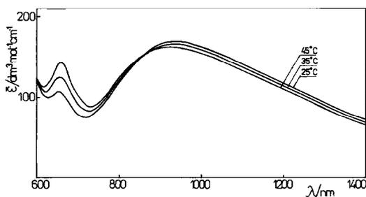
Fig. 8. The influence of temperature on the absorption spectrum of copper(II) for  $\text{CuBr}_2$ -DMF-chlorobenzene solution ( $C_{\text{CuBr}_2} = 0.0051$ ,  $X_{\text{chlorobenzene}} = 0.945$ ).
