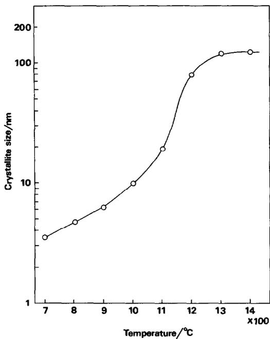
Fig. 6. Crystallite size of spinel with increasing temperature.
