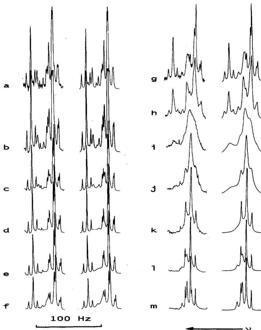
Fig. 8. Experimental and computer synthesised variable temperature  $^1\text{H}$  NMR spectra of  $[\text{PtMe}_3(\text{MeSCH}_2\text{CH}_2\text{S})_2]^+\text{BF}_4^-$  showing the effects of sulphur inversion on the S—Me signals.
