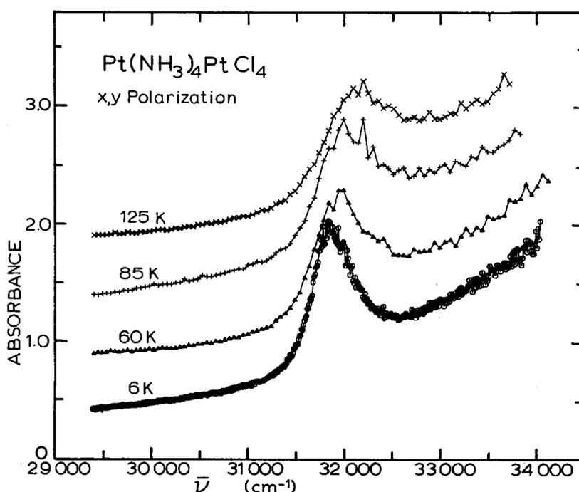
Fig. 3. Temperature dependence of the narrow high-energy band in the  $4\text{-}\mu\text{m}$  MGS crystal of Fig. 2 for  $x,y$  polarization.
