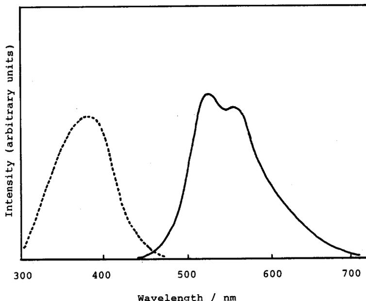
Fig. 4. Emission (—) and excitation (---) spectra of  $\text{ReBr}(\text{CO})_3\text{Y}_{\text{P}}$  in MeOH/EtOH (1:4 v/v) at 77 K.
