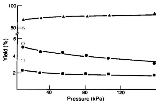
Fig. 2. Yield (%) in the system  $\gamma$  + GeH<sub>4</sub> as a function of the reactant pressure: (▲) GeH<sub>4</sub>, (●) HT, and (■) Ge<sub>2</sub>H<sub>5</sub>T.  $\Delta$ ,  $\circ$  and  $\square$  = the same products in the presence of Ne (2:1). Dose =  $8 \times 10^5$  Gy.
