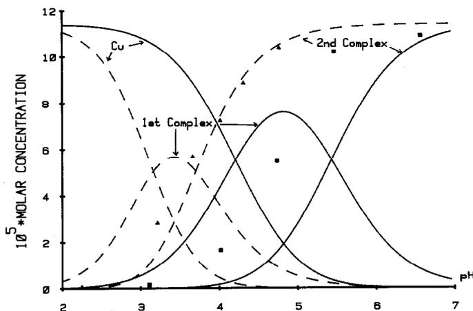
Fig. 3. Species distribution curves for NIBL–Cu and PNML–Cu mixtures,  $R = 15$ . Full line : NIBL ; dotted line PNML. Points are concentration values calculated from circular dichroism measurements<sup>4</sup> for the second complex : (■) NIBL ; (▲) PNML.
