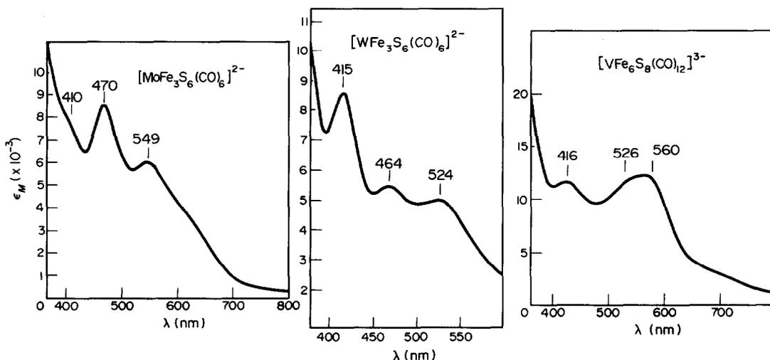
Fig. 2. Visible-absorption spectra of  $[\text{MoFe}_3\text{S}_6(\text{CO})_6]^{2-}$  (5),  $[\text{WFe}_3\text{S}_6(\text{CO})_6]^{2-}$  (7), and  $[\text{VFe}_6\text{S}_8(\text{CO})_{12}]^{3-}$  (9) in acetonitrile solutions.
