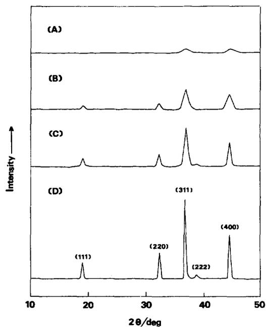
Fig. 4. X-ray diffraction patterns for specimens heated at (A) 700, (B) 1000, (C) 1100 and (D) 1250°C.
