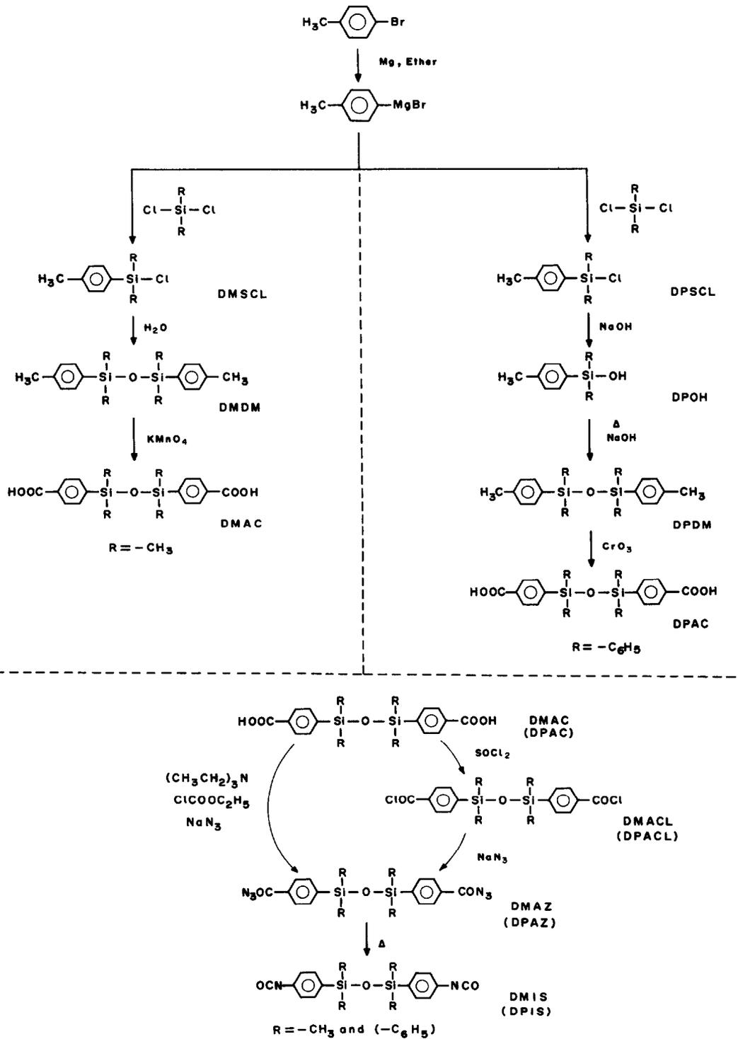
Fig. 1. Synthesis of disiloxane-containing diisocyanates.
