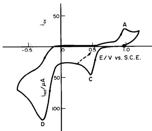
Fig. 2. Cyclic voltammogram recorded on the same solution of Fig. 1, after exhaustive electrolysis at  $+1.0 \text{ V}$  vs S.C.E. ●, Starting potential for cathodic direct scan.
