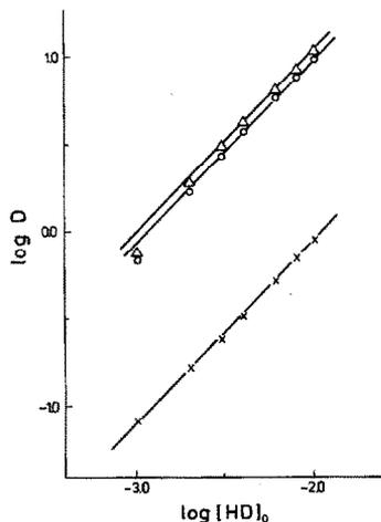
Fig. 4. HD concentration dependency of the  $D$  of Zn(II). (○) [Im] = 0.20 M, [HCl] = 0.10 M; (△) [2MIm] = 0.20 M, [HCl] = 0.10 M; (×) [His] = 0.12 M, [HCl] = 0.06 M.
