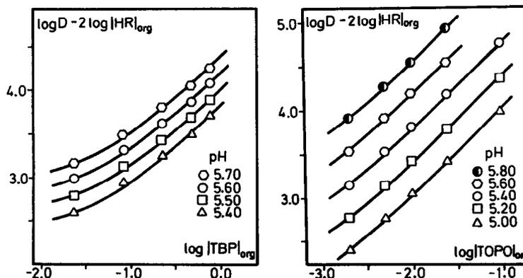
Fig. 3. Position of best fit between the theoretical  $\log Y = f(\log X)$  (continuous lines) and experimental data  $\log D - 2 \log [HR]_{org} = f(\log [S]_{org})$  at different constant pH values in the presence of TBP or TOPO.
