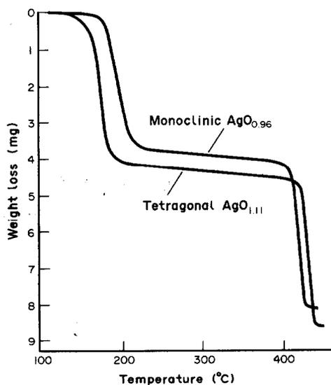
Fig. 2. Thermogravimetry of AgO. Sample weight, 61.5 mg; heating rate:  $4^\circ\text{C min}^{-1}$ ; atmosphere: static air.
