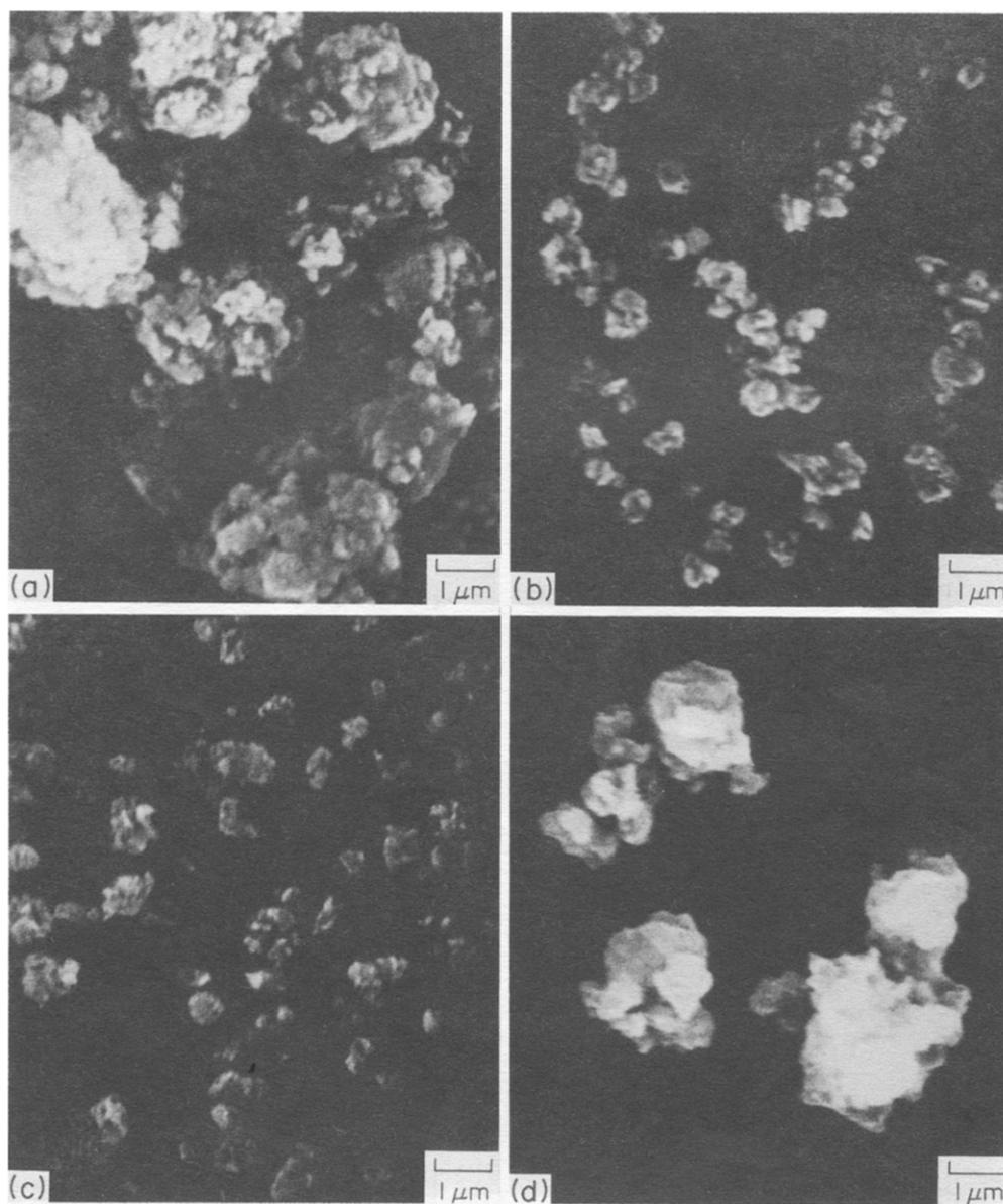
Fig. 4. Electron micrographs for (a) starting powder B, (b) 600°C, (c) 1000°C, and (d) 1300°C. Heating rate is 10°C/min.
