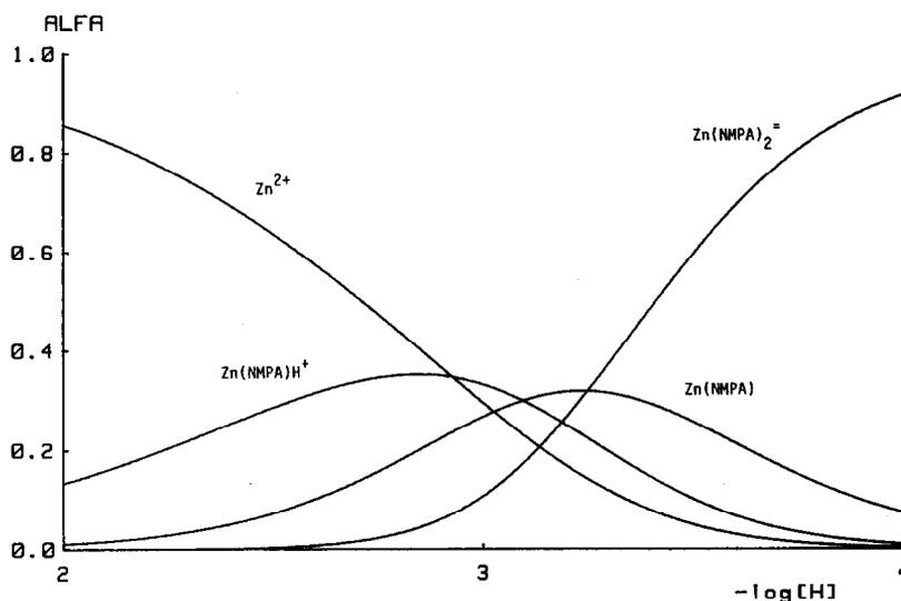
Fig. 5. Species distribution for Zn(II)-NMPA-H complexes.  $[Zn^{2+}] = 1 \text{ mM}$ ,  $[NMPA] = 3 \text{ mM}$ .
