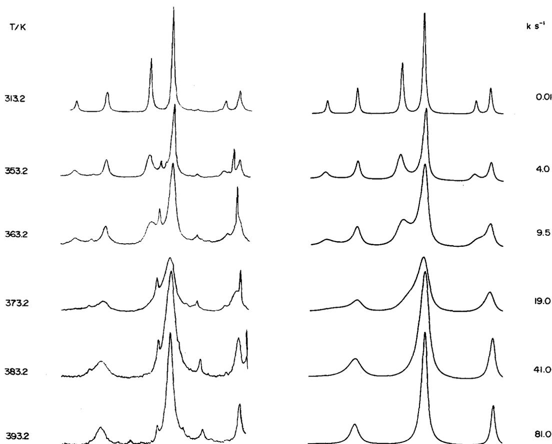
Fig. 5. Variable-temperature experimental and computer-simulated  $^1\text{H}$  NMR spectra of  $[\text{Pd}(\text{dppe})(\mu_2\text{-SMe})_2\text{PtBrMe}_3]$  showing the effects of platinum-methyl group scrambling.
