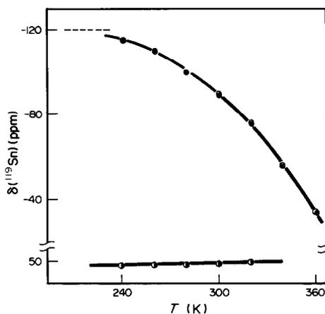
Fig. 1. Temperature dependence of  $^{119}\text{Sn}$  chemical shifts of tribenzyltin(IV) chloride in pyridine (py) and  $\text{CDCl}_3$ . Concentration (mole fraction): (O)  $1.35 \times 10^{-2}$  (py), (●)  $5.11 \times 10^{-2}$  (py), (●)  $2.12 \times 10^{-2}$  ( $\text{CDCl}_3$ ).
