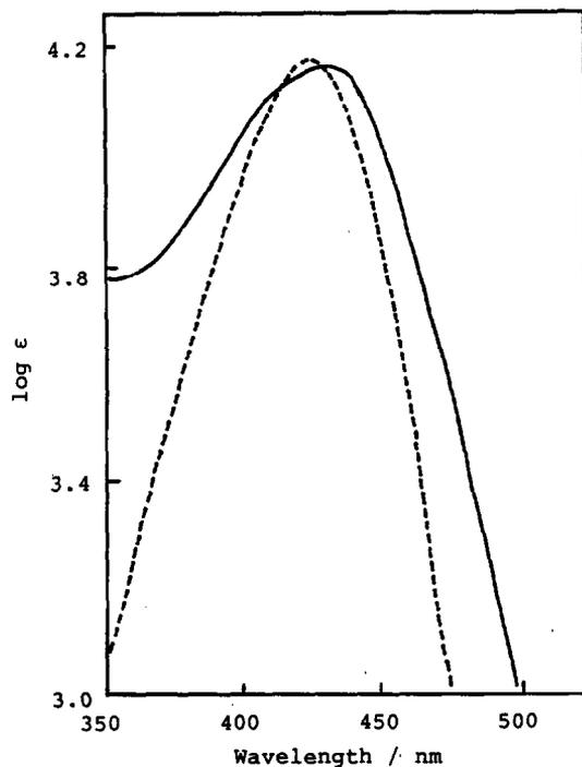
Fig. 3. Electronic absorption spectra of  $\text{ReBr(CO)}_3\text{Y}_{\text{N-H}}$  (—) and  $\text{Y}_{\text{N-H}}$  (---) in MeOH/EtOH (1:4 v/v) at 298 K.
