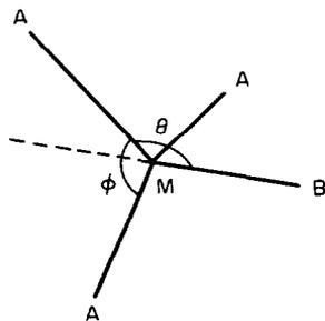
Fig. 4. Application of the Packing Centre Rule in calculating the molecular geometry of the structural pattern MA<sub>3</sub>B ( $\theta = \angle AMB$ ,  $\phi = \angle AMA$ ): the vector sum must be zero along the MB direction.
