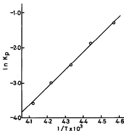
Fig. 3. van't Hoff plot for the oxygenation reaction of  $\text{py}\cdot\text{Co(II)TPP}$ .
