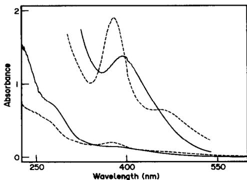
Fig. 2. Comparison of the electronic absorption spectra of  $Mo_2(OBu^t)_6$  (solid line) and  $W_2(OBu^t)_6$  (dashed line) in THF solutions, at  $1.0 \times 10^{-3}$  and  $1.0 \times 10^{-4}$  M.
