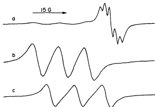
Fig. 3. Typical ESR spectra of the interaction of  $\text{Fe}(\text{NO})\cdot\text{L}_2$  with bases ( $T = 298$  K): (a)  $\text{Fe}(\text{NO})_2(\text{Et-xant})$  [obtained during dissolution of  $\text{Fe}(\text{NO})(\text{Et-xant})_2$  in *i*-amyl alcohol:pyridine (3:1)], (b)  $\text{Fe}(\text{NO})(\text{Et-xant})_2$  in *i*-amyl alcohol, and (c)  $\text{Fe}(\text{NO})(\text{Et}_2\text{dtc})_2$  [obtained by adding (a) to  $\text{Ni}(\text{Et}_2\text{dtc})_2$ ].
