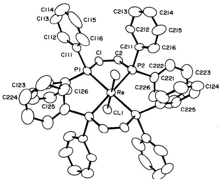
Fig. 2. ORTEP representation of  $\text{ReCl}_2(\text{dppee})_2$  in which atoms are given as their 50% probability ellipsoids. Unlabeled Cl, P and C atoms are related to the corresponding labeled atoms by an inversion center.
