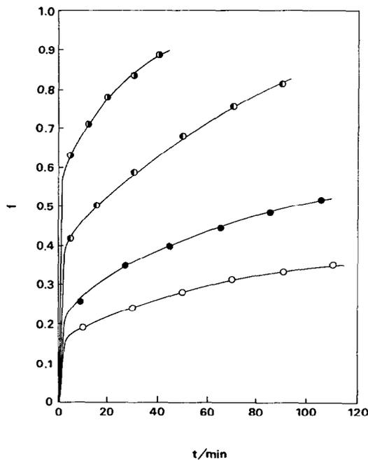
Fig. 8. Isotherms for crystallization of spinel at (○) 960, (●) 1020, (◐) 1100 and (◑) 1160°C.
