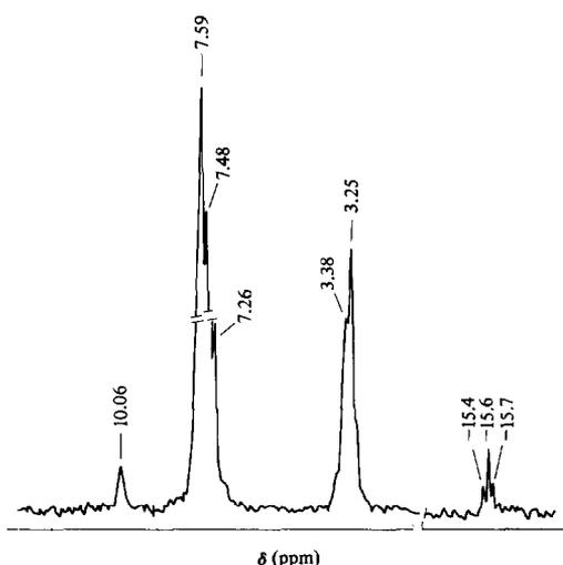
Fig. 3.  $^1\text{H}$  NMR spectrum of  $[\text{Ir}(\text{H})(\text{Cl})(\text{CO})(\text{DPEA})]\text{Cl}$ .
