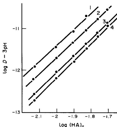
Fig. 1. Extraction of Pr(III) with various  $C_{HA}$  in different organic solvents: (1)  $CCl_4$ , (2) benzene, (3) toluene, and (4) xylene.
