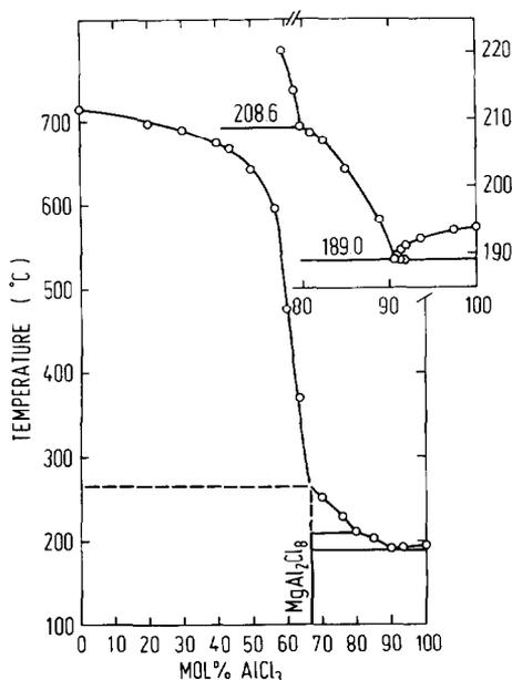
Fig. 1. The  $\text{MgCl}_2$ – $\text{AlCl}_3$  phase diagram.
